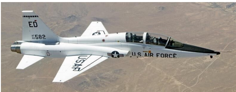
The Area Rule-influenced designs of the B-58 (Top) and the T-38 (Above) showing the narrow fuselages.
