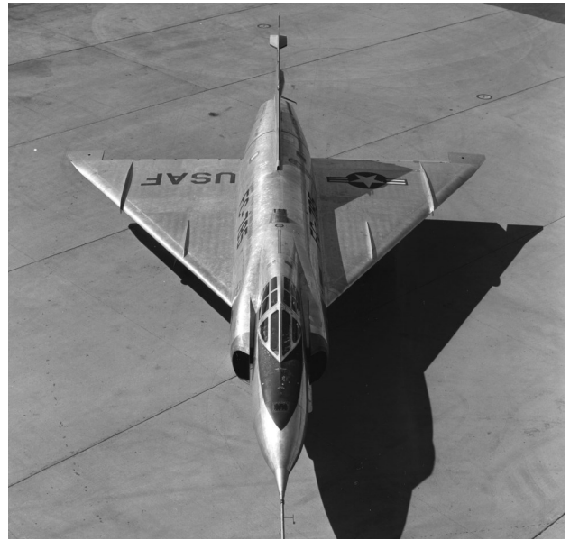
Above (L and R): The early F-102 with the straight fuselage before the Area Rule redesign.
