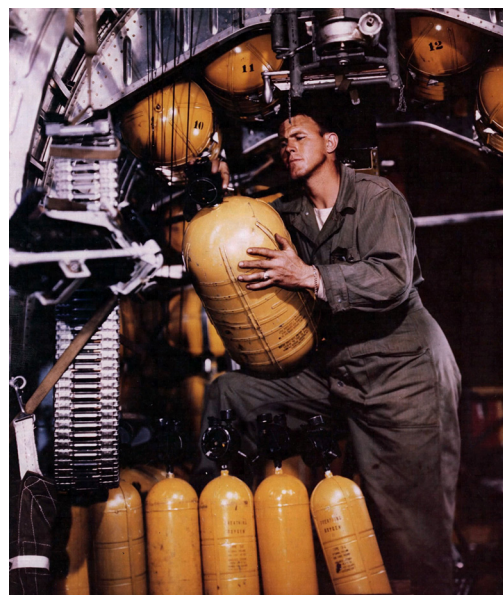
Right: Maintenance technician servicing the oxygen bottle system in a B-24.
