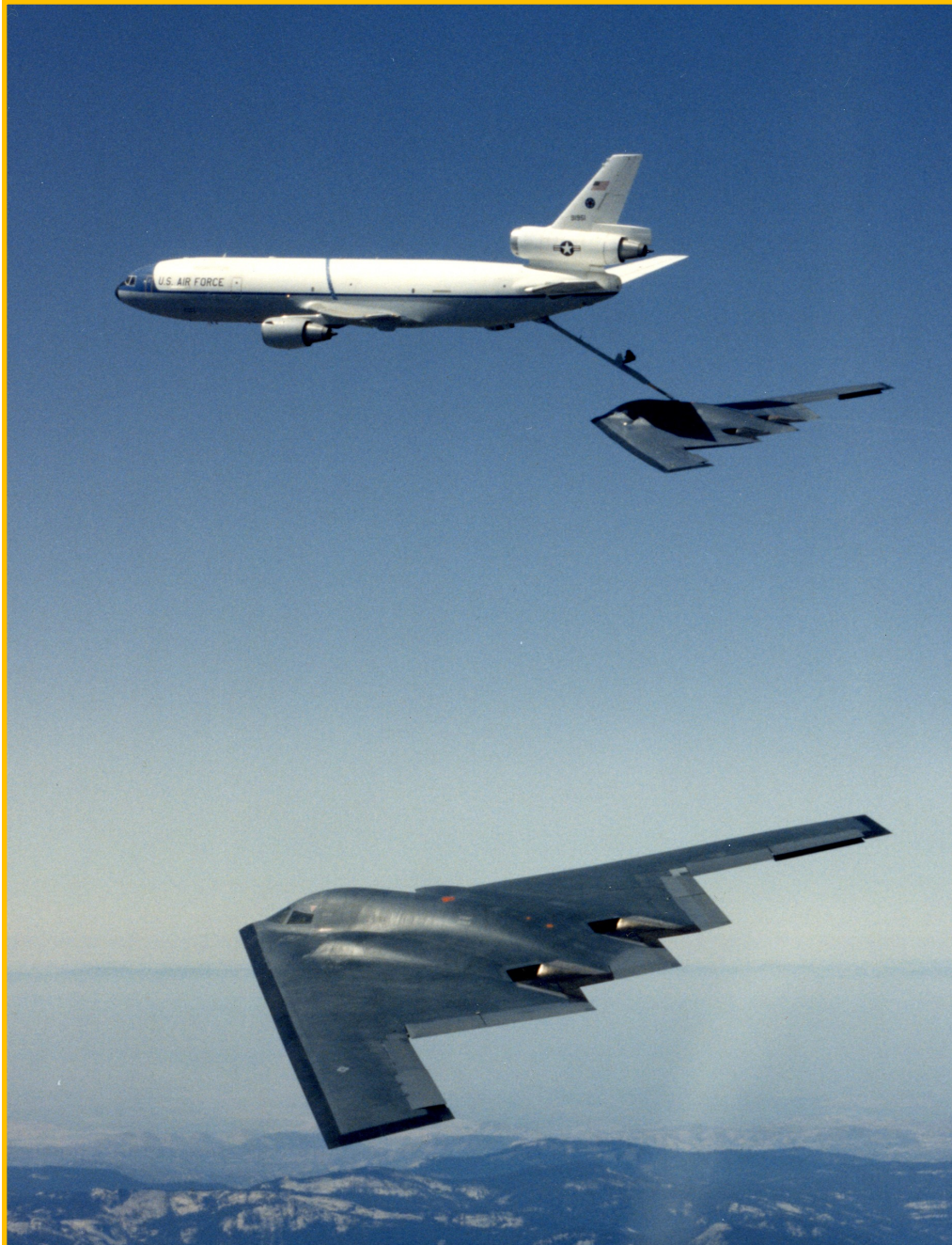
Two Northrop Grumman B-2 Spirit aircraft take on fuel from a KC-10 Extender near Edwards AFB, Calif., during early flight testing of the new stealth bombers.
