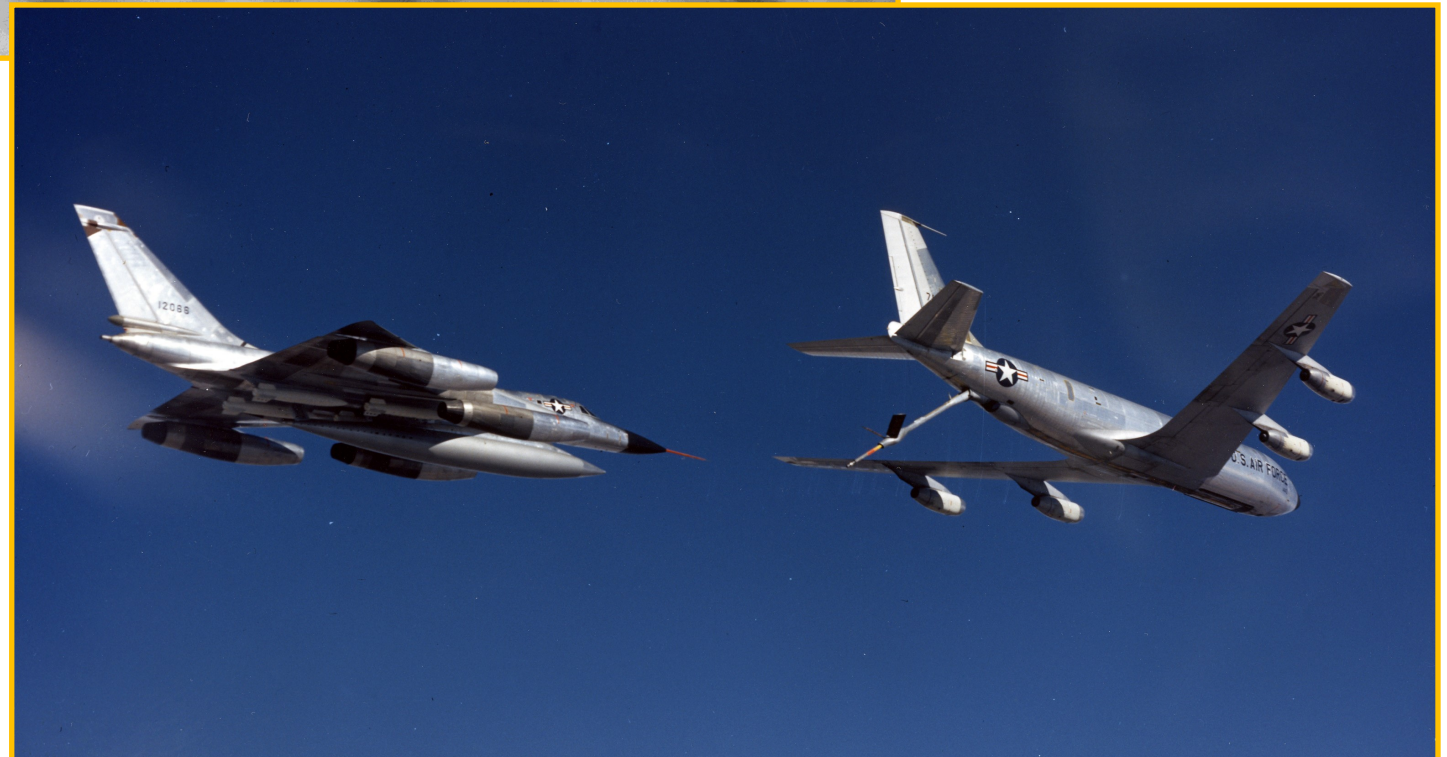
One of the most challenging aircraft to perform in-flight refueling, the B-58 Hustler. With the highly-swept delta wing and limited visibility, crews had to remain alert during this delicate activity.
