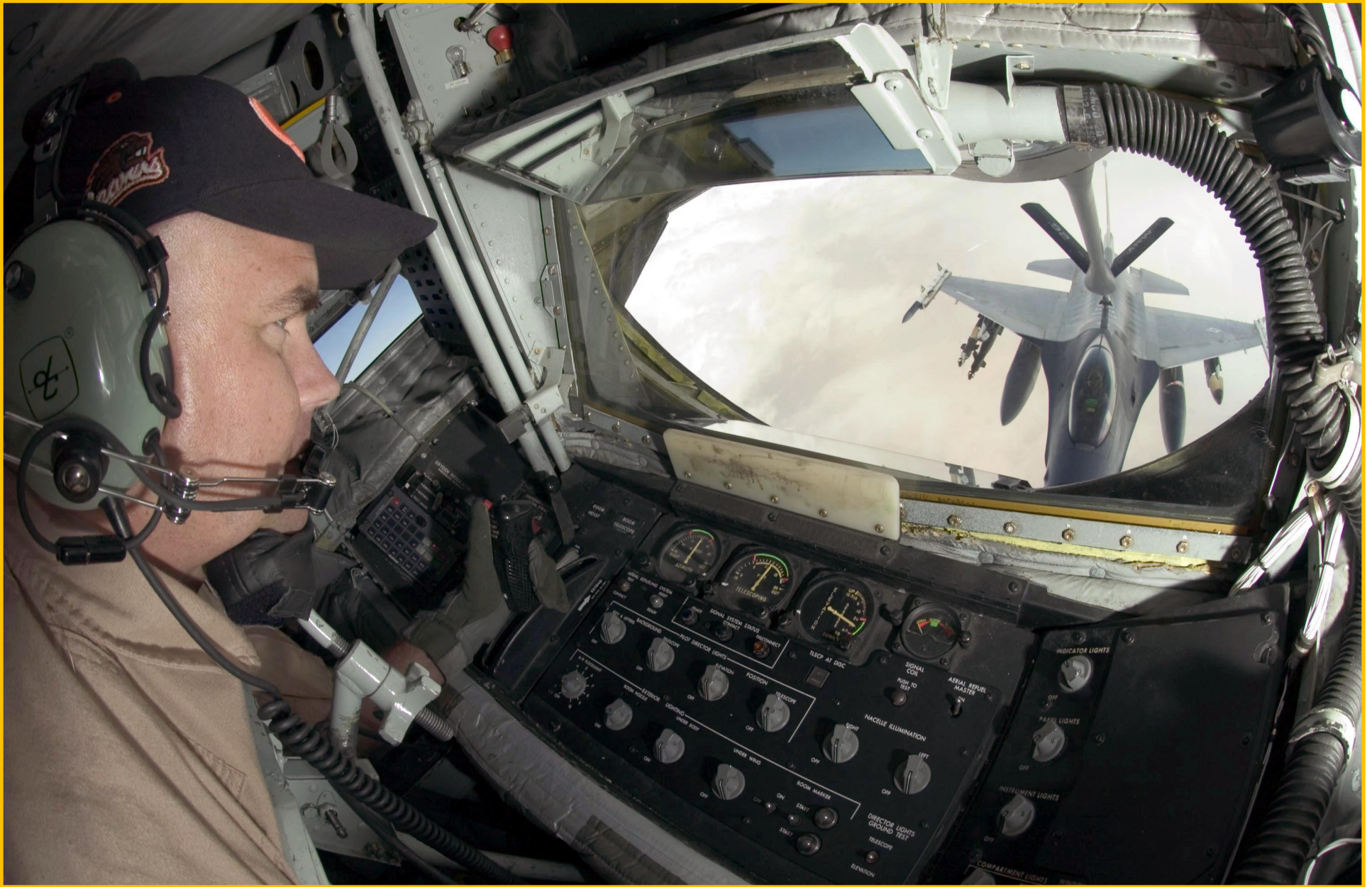
Boom operator TSgt John Baughman connects the 92nd Air Refueling Squadron's KC-135 Air Refueling Tanker from Farichild AFB, Wash., with an F-16 from Aviano Air Base's 55th Fighter Squadron in support of Operation Iraqi Freedom. (USAF Photo by MSgt John E. Lasky)
