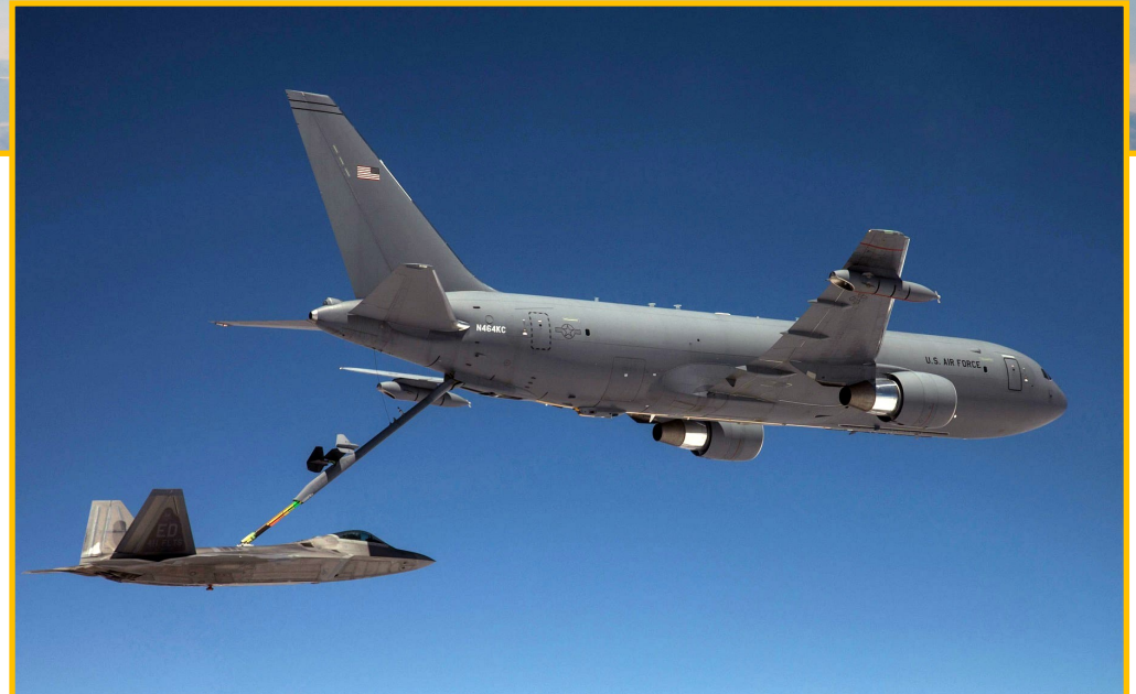
Supported by the 418th Flight Test Squadron (FLTS) and the 461st FLTS at Edwards AFB, Calif., certification testing between the KC-46 Pegasus and F-22 Raptor was completed in November 2019.
