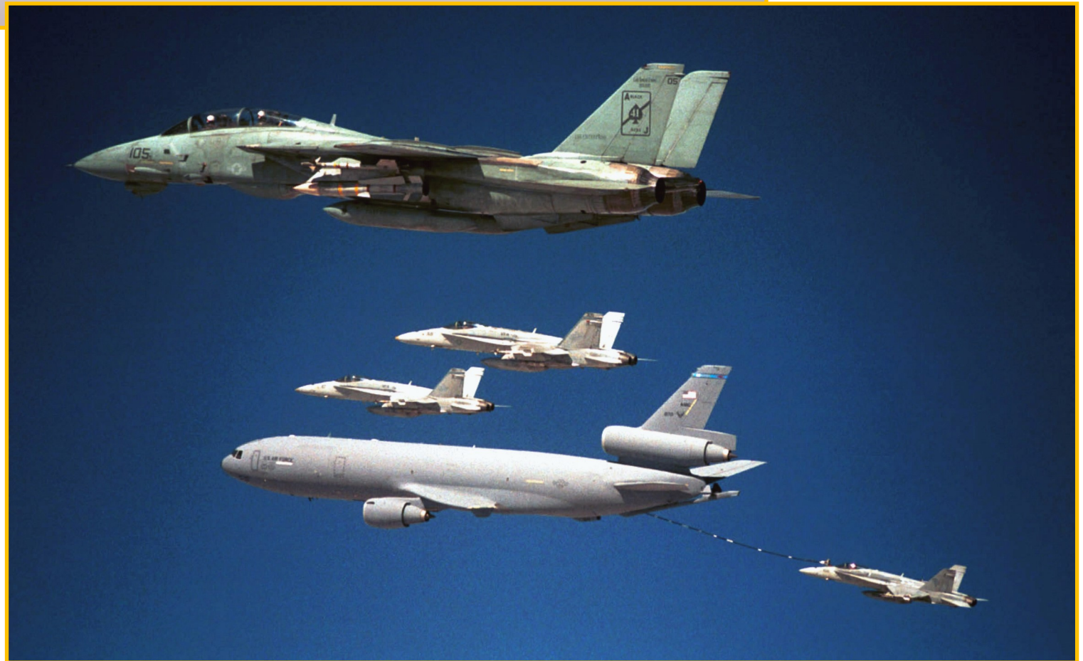
US Navy (USN) F-14D Tomcat and F/A-18C Hornets conduct air-to-air refueling operations with a US Air Force KC-10 Extender aircraft from the 763rd Expeditionary Air Refueling Squadron, during a refueling mission flown in support of Operation Enduring Freedom. Unlike the KC-135, the refueling hose was a permanent installation.
