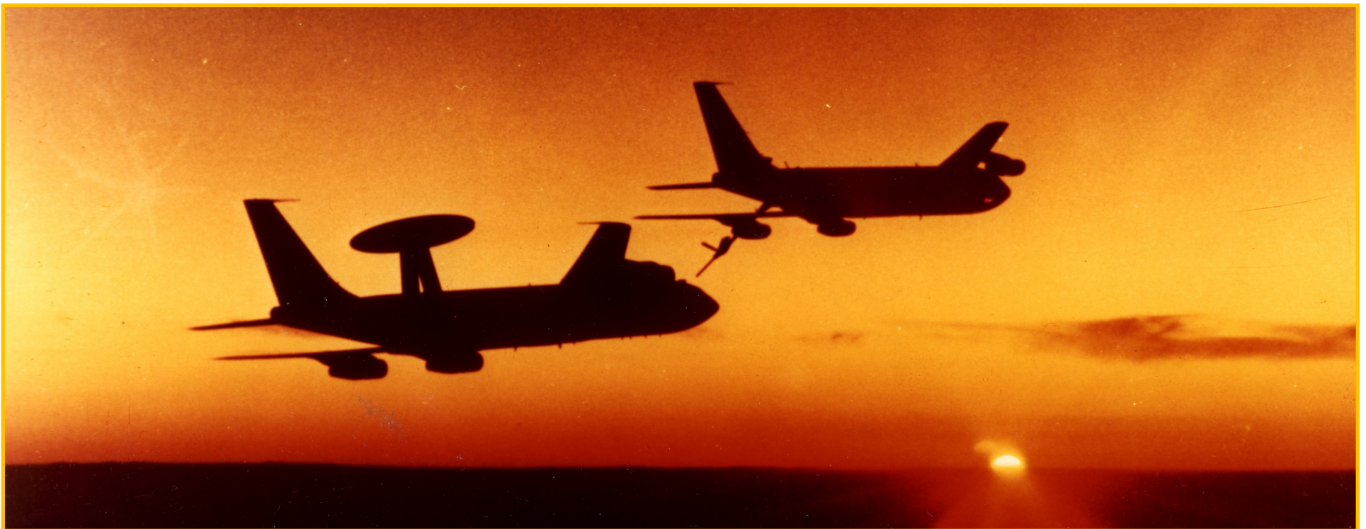
Sunset aerial refueling operation between a KC-135E Stratotanker and a Boeing E-3A AWACS.
