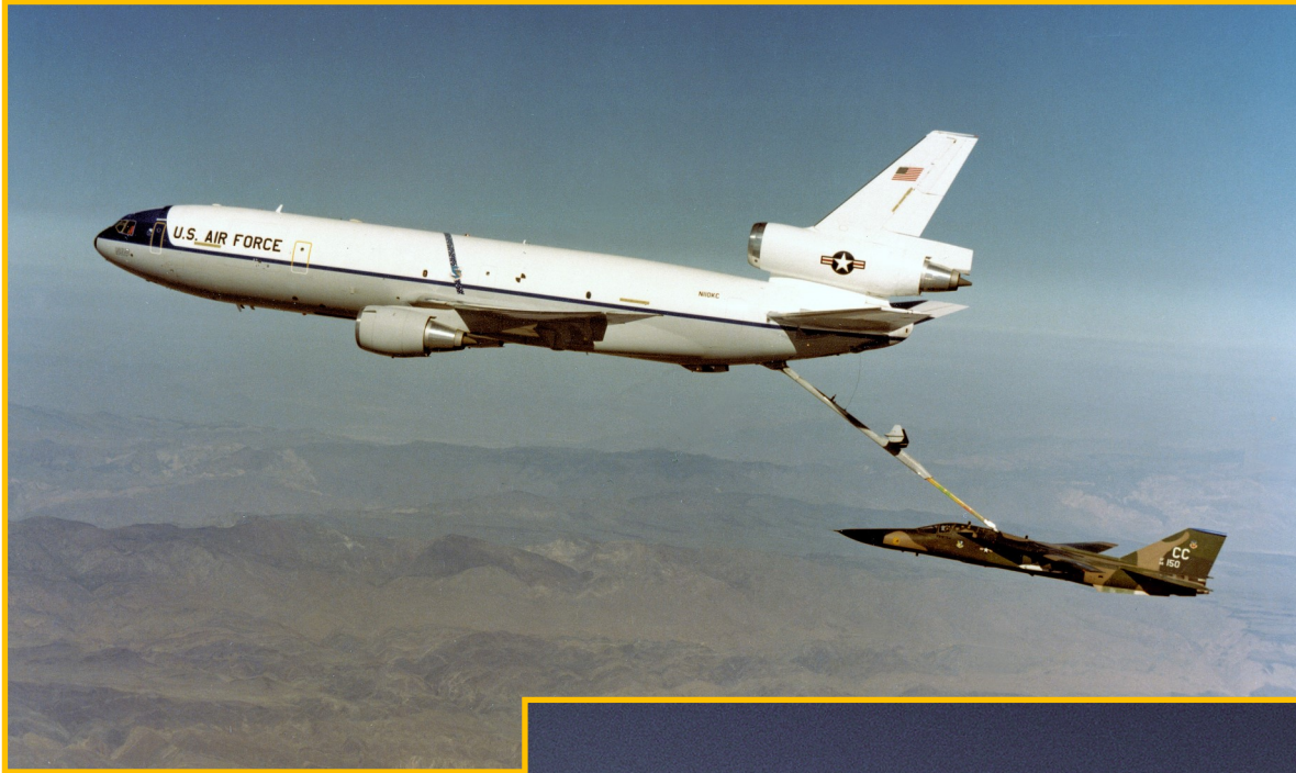
A McDonnell Douglas KC-10 Extender provides fuel to a General Dynamics F-111 Aardvark from Cannon AFB, NM.
