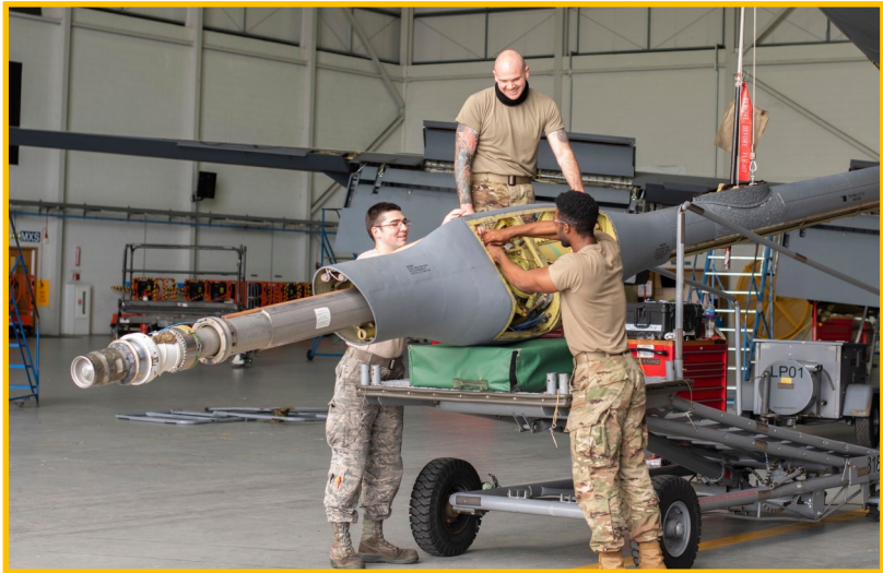
Airmen of the 100th Maintenance Squadron Hydraulics section repair the flying boom of a KC-135 Stratotanker at RAF Mildenhall, England, July 17, 2020. The 100 MXS maintains the only permanent fleet of KC-135s in the United States in Europe and Air Forces Africa theatre. (USAF photo by Airman 1st Class Joseph Barron)
