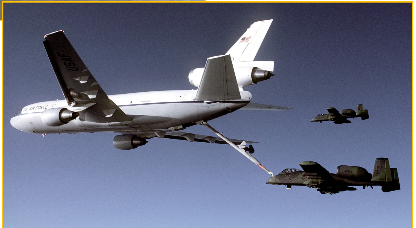
KC-10 Extender aircraft from the 78th Refueling Squadron (AFRES) refuels an A-10 Thunderbolt II from the 917th Tactical Fighter Group (AFRES) as another A-10 awaits in turn in the background. (USAF photo by Ken Hackman)
