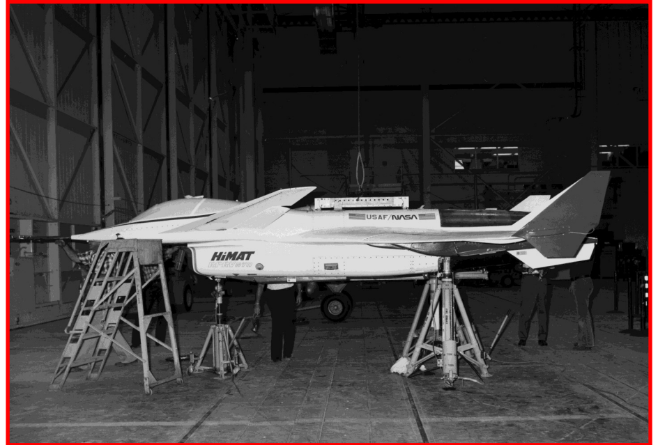
HiMAT, RPRV 870, during weight and balance checks on August 7, 1978. Note the Rockwell logo on the vertical stabilizer is painted over.
