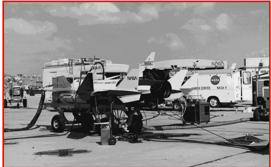
Ground testing of the GE J85-21 while installed in the first HiMAT vehicle, commenced on September 12, 1978. The large hoses attached to the vehicle in the photo above, right provided cold air to the avionics bay to prevent overheating in the hot desert sun. Note the signatures of HiMAT program personnel on the inside of the avionics bay cover above, left.
