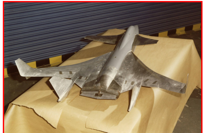
Rockwell designed HiMAT around a modular core in order for different design configuration testing shown at left. At least one HiMAT wind tunnel model received the square, 2D thrust vectoring nozzle modification. Rockwell constructed a full-scale 2D nozzle mockup that was test fit on the second HiMAT, yet no actual testing followed.
