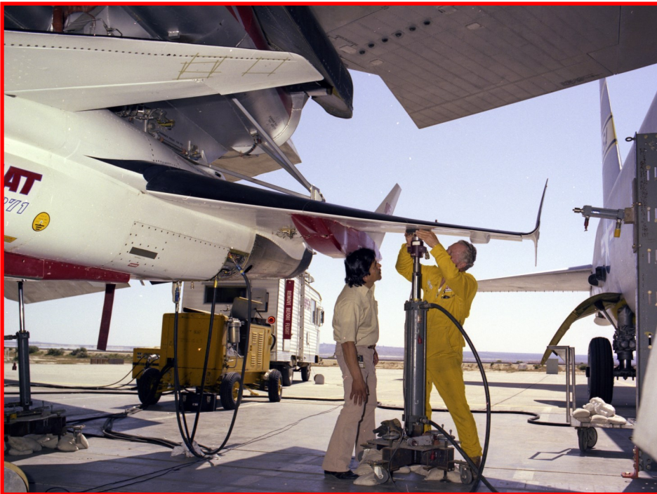
This series of photographs show HiMAT, RPRV 871, during NB-52B mating and calibration operations on April 22, 1982. In addition to new markings, ship 2 received new instrumentation on the upper wing and canard surfaces. All of this instrumentation required delicate calibration prior to its next flight.
