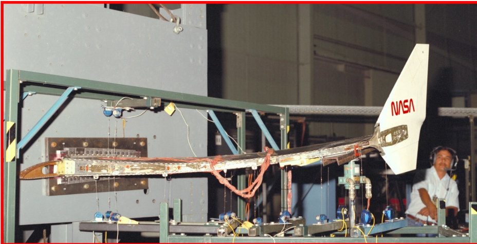
Predicted HiMAT composite wing bend and twist measurements during an 8G windup turn at 30,000 feet
