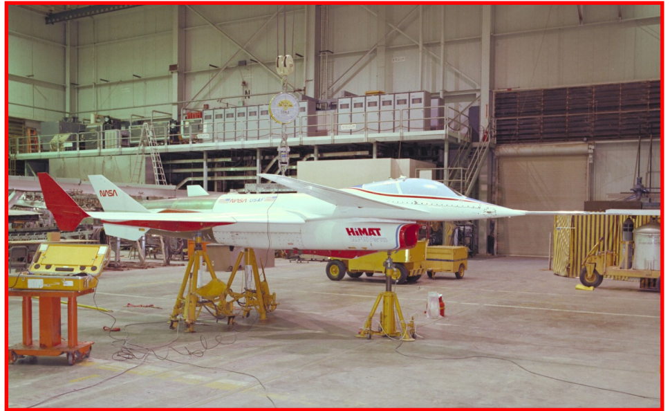
Prior to taking over flight duties from RPRV 871, RPRV 870 undergoes weight and balance checks on December 10, 1981.
