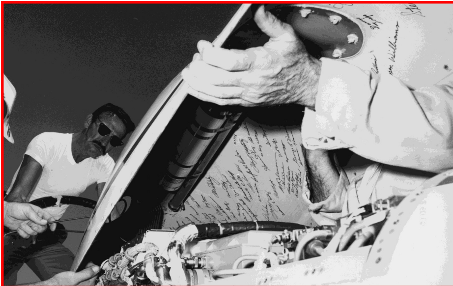
Ground testing of the GE J85-21 while installed in the first HiMAT vehicle, commenced on September 12, 1978. The large hoses attached to the vehicle in the photo above, right provided cold air to the avionics bay to prevent overheating in the hot desert sun. Note the signatures of HiMAT program personnel on the inside of the avionics bay cover above, left.
