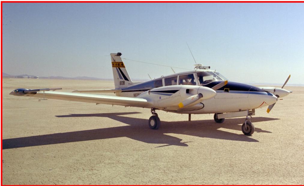
Two years prior to the arrival of the first HiMAT test aircraft, NASA test pilot William H. "Bill" Dana practiced perfecting remote landing techniques from the ground-based cockpit utilizing a camera and telemetry system installed in NASA's PA-30 Twin Comanche.
