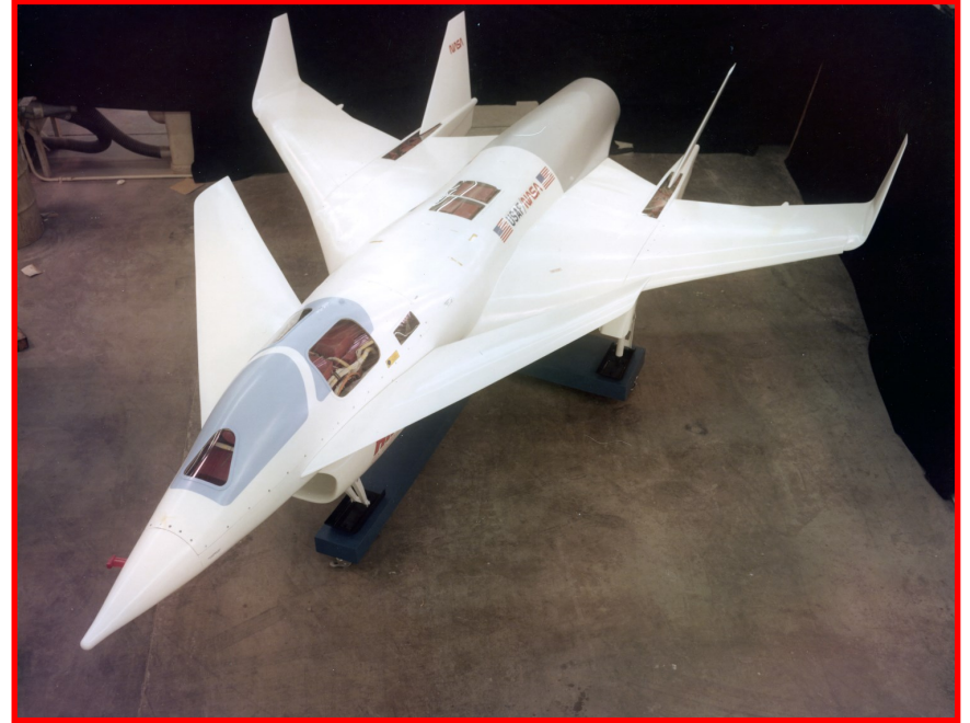
Rockwell constructed at least two full-scale mockups of HiMAT. One had clear windows enabling internal components to be viewed. Notable is the compact size of the internal structure.
