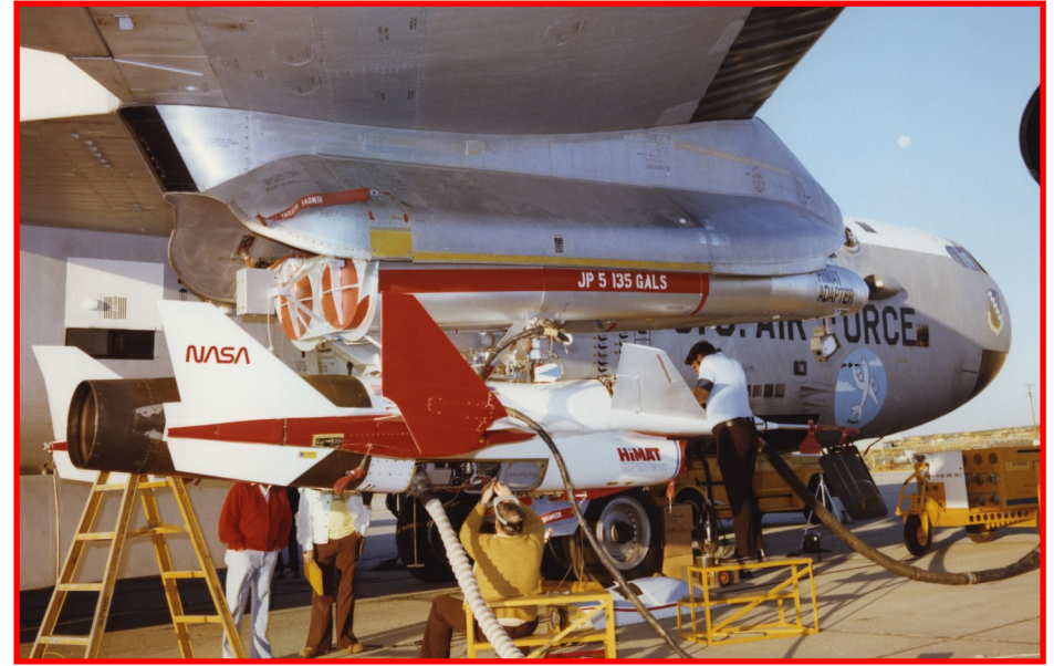
After a year of ground testing and simulations, the first HiMAT is ready to begin flight testing. Towing HiMAT out to the NB-52B in July, 1979 (above, left) prior to the first captive test flight. A full moon hovers in the background as technicians finish final checks before starting engines on the NB-52B mothership (above, right).
