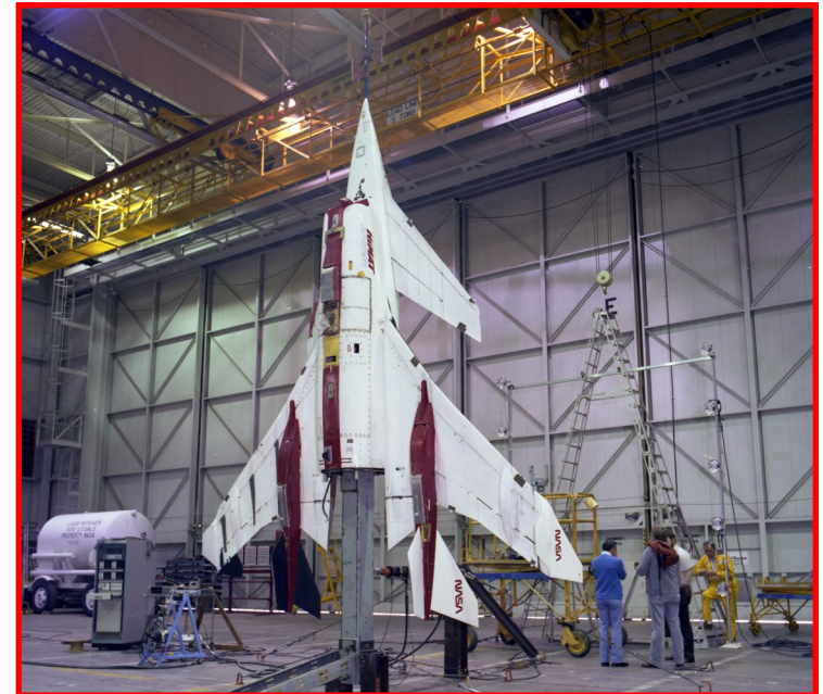
With the flight program over, the first HiMAT was placed in storage while the second was used for a series of composite aeroelasticity tests. These photos taken February 7, 1983, show RPRV 871 in the NASA ADFRF Loads Laboratory during photogrammetric measurement testing.
