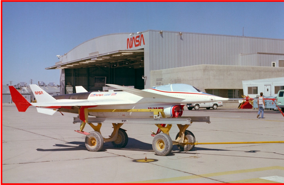
After a year of ground testing and simulations, the first HiMAT is ready to begin flight testing. Towing HiMAT out to the NB-52B in July, 1979 (above, left) prior to the first captive test flight. A full moon hovers in the background as technicians finish final checks before starting engines on the NB-52B mothership (above, right).
