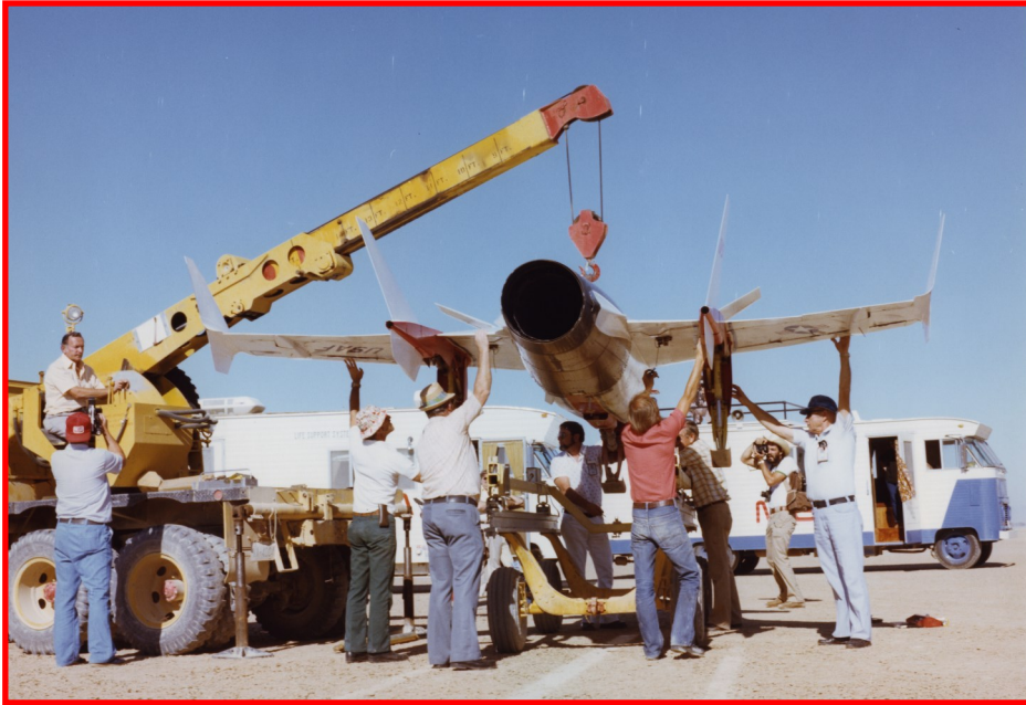
The laborious task of loading HiMAT onto its transport cart fell to the ground support crew that traveled to the landing site in vans shown in the background.
