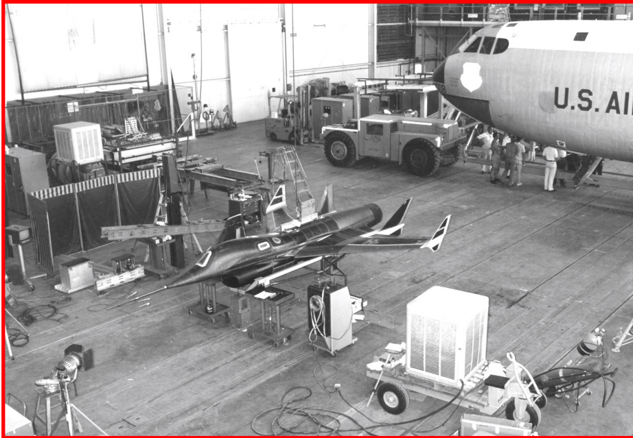
The second HiMAT, RPRV 871, began ground testing almost immediately upon arrival as shown above during moment of inertia testing on July 18, 1978.
