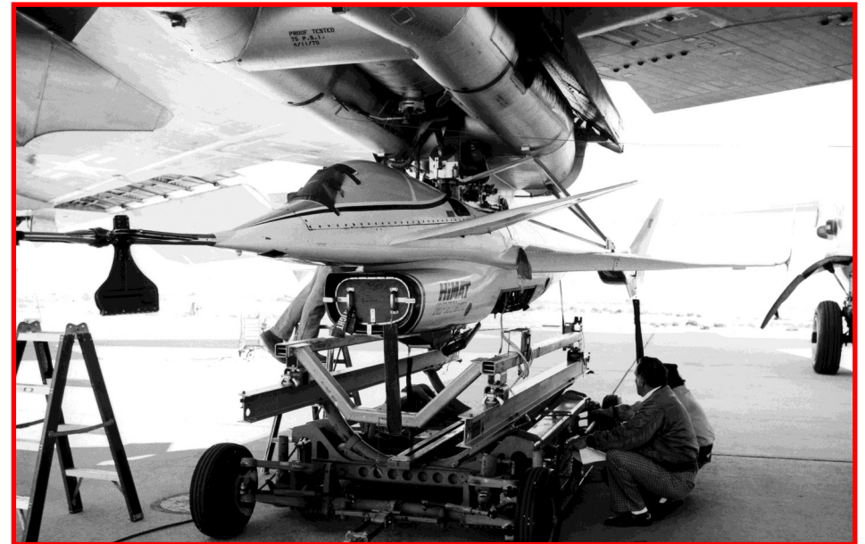
As shown in this series of black & white photos on this page and the following, mating HiMAT to the NB-52B mothership could be a tedious, time-consuming task. Little room to work made connecting the many instrumentation & electrical cables, safety latches and fuel connection more challenging.
