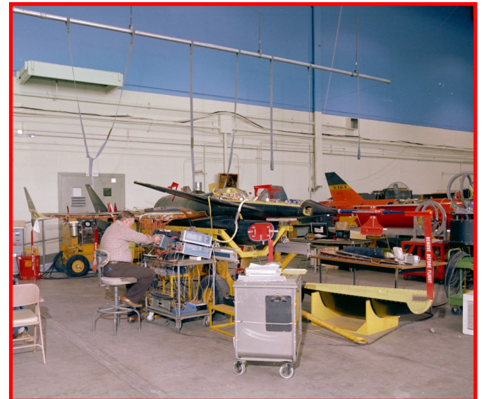
A NASA technician runs HiMAT RPRV 871 avionics system through a series of flight simulations through the use of ground based flight simulator setup attached directly to the onboard flight control computer. Note the red NASA Firebee II drone in the background.
