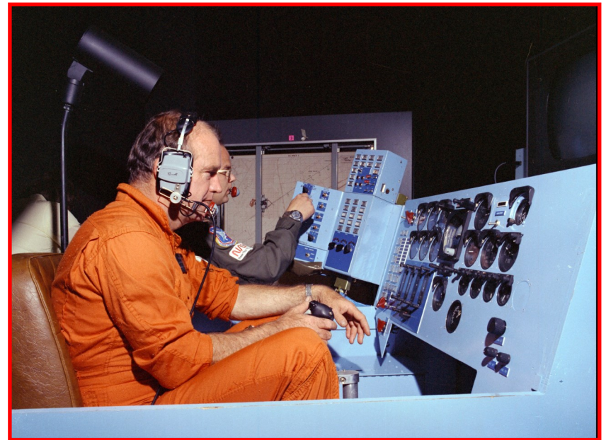
Two years prior to the arrival of the first HiMAT test aircraft, NASA test pilot William H. "Bill" Dana practiced perfecting remote landing techniques from the ground-based cockpit utilizing a camera and telemetry system installed in NASA's PA-30 Twin Comanche.
