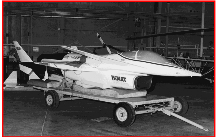
The second mockup, constructed from wood and fiberglass, gave an accurate representation of the actual vehicle. Crated at Rockwell and shipped to ADFRF, the mockup could be shown to visiting dignitaries. This mockup is currently stored at the Air Force Flight Test Center Museum at Edwards AFB, CA, awaiting restoration.
