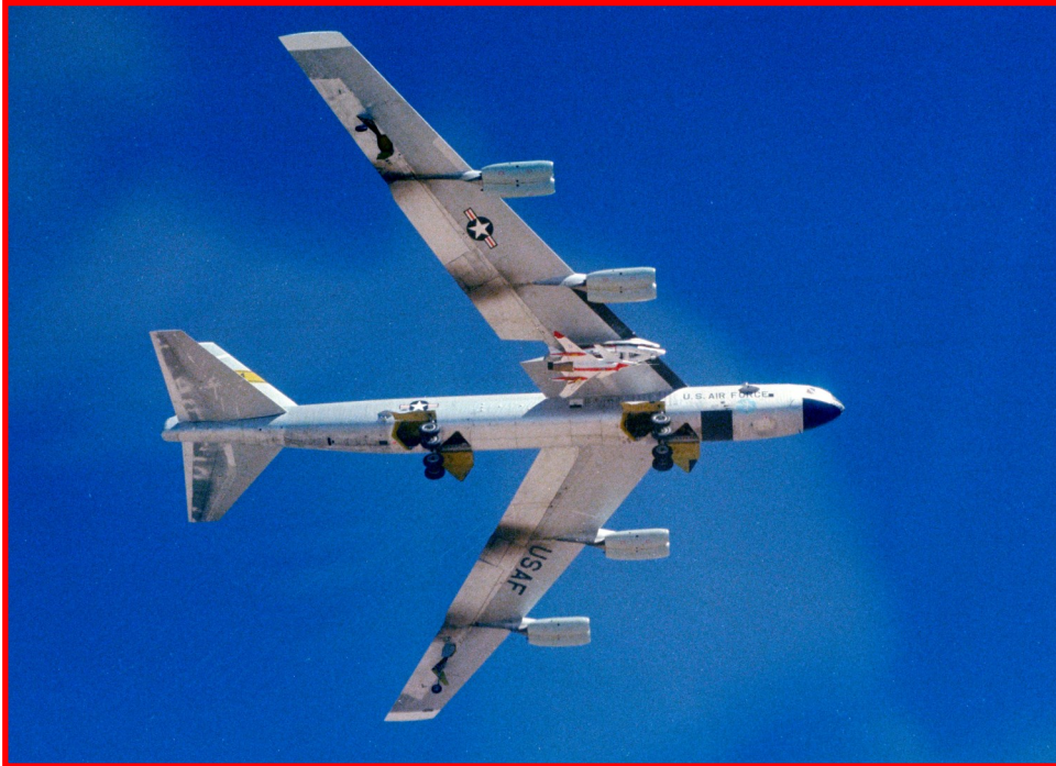
The small test aircraft is barely visible on the right wing of its NB-52B mothership. HiMAT completed two, planned, captive flights before taking to the air on its own.
