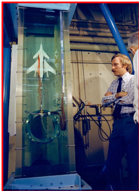
NASA tested a 1/15th scale HiMAT model in the water tunnel at Ames/Dryden Flight Research Facility during May 1979. Inexpensive water tunnel models made use of colored dyes injected into the water flow to visualize airflow under different flight conditions.
