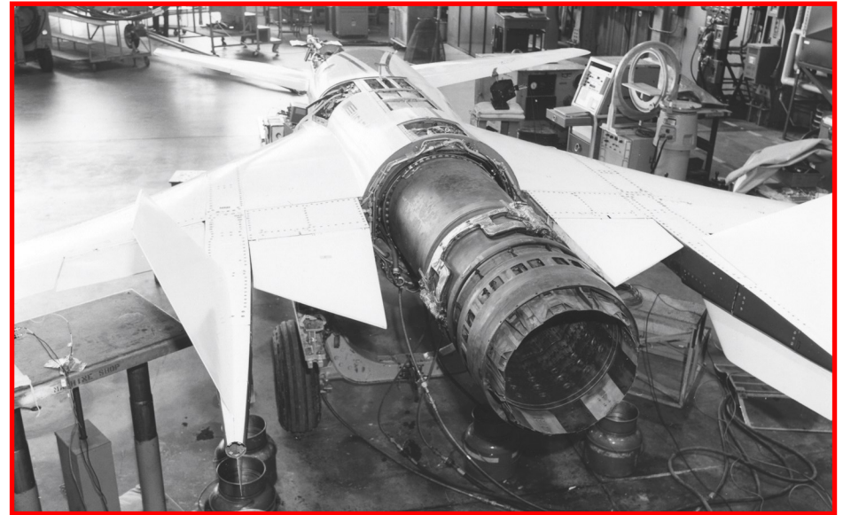
Maintenance access to the GE J85-21 turbojet on the HiMAT aircraft required the removal of the entire aft metal engine fairing.
