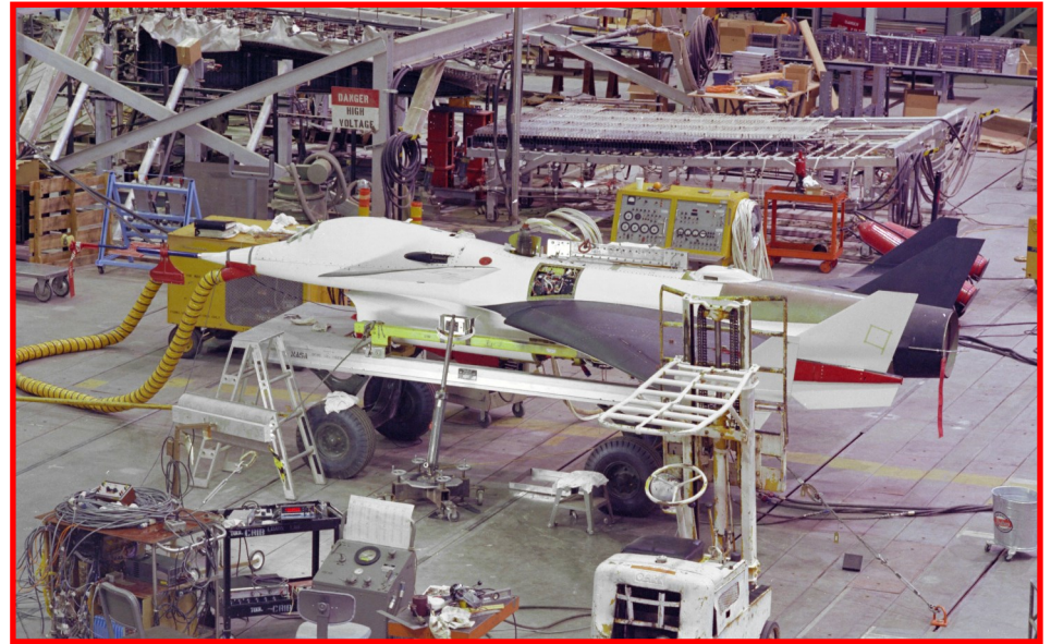
The second HiMAT receives final systems checks to the avionics system prior to its first captive flight in June 1981.
