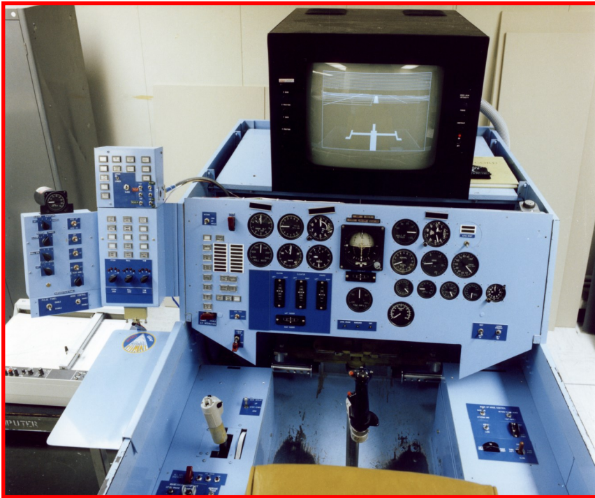
The HiMAT remote cockpit (left) with the video display contained just the basic information required for the pilot. HiMAT flight markings added to the NB-52B after each mission (above). Red flames on each HiMAT stencil depicted powered free flights.
