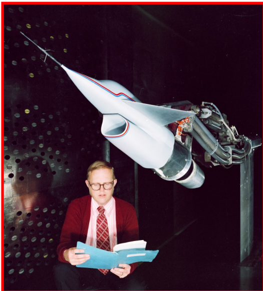
NASA's Lewis Research Center performed wind tunnel testing on a HiMAT inlet test model, as well as the J85-21 engine. Note the canard shape of this model.
