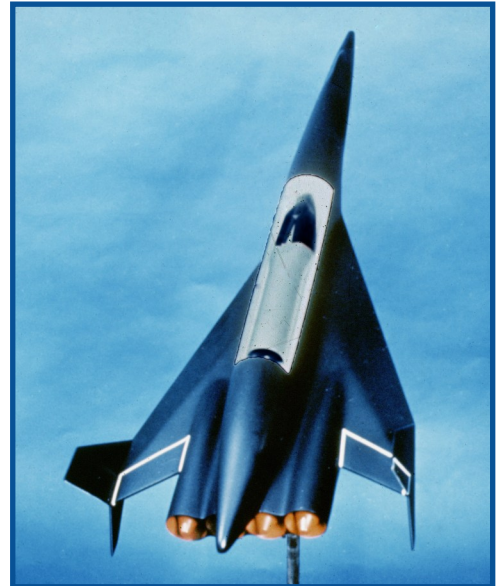
Above (2): Several contractors submitted proposals under the Advanced Interceptor study from the U.S. Air Force in the late 1960's. This design proposed using scramjet engines as well as an internal payload bay on the upper fuselage. Much of the information gathered from this study was applied to the hypersonic X-24C designs.
