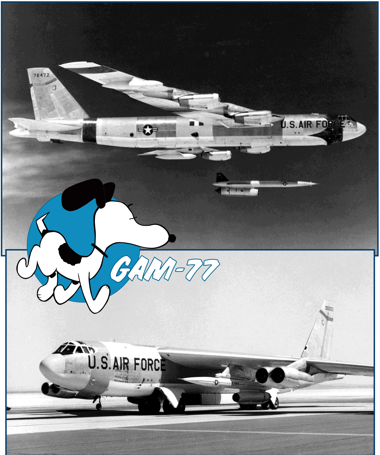
Top: A GAM-77 Hound Dog is launched over the Air Force Missile Test Range, Eglin AFB. Barely visible on the nose of B-52G, 57-6472, is the GAM-77 nose art.
