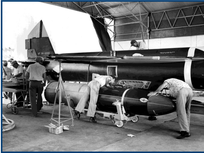
Left: Maintenance technicians install one of the Marquardt RJ43-MA-3 ramjet engines used to power the BOMARC .
