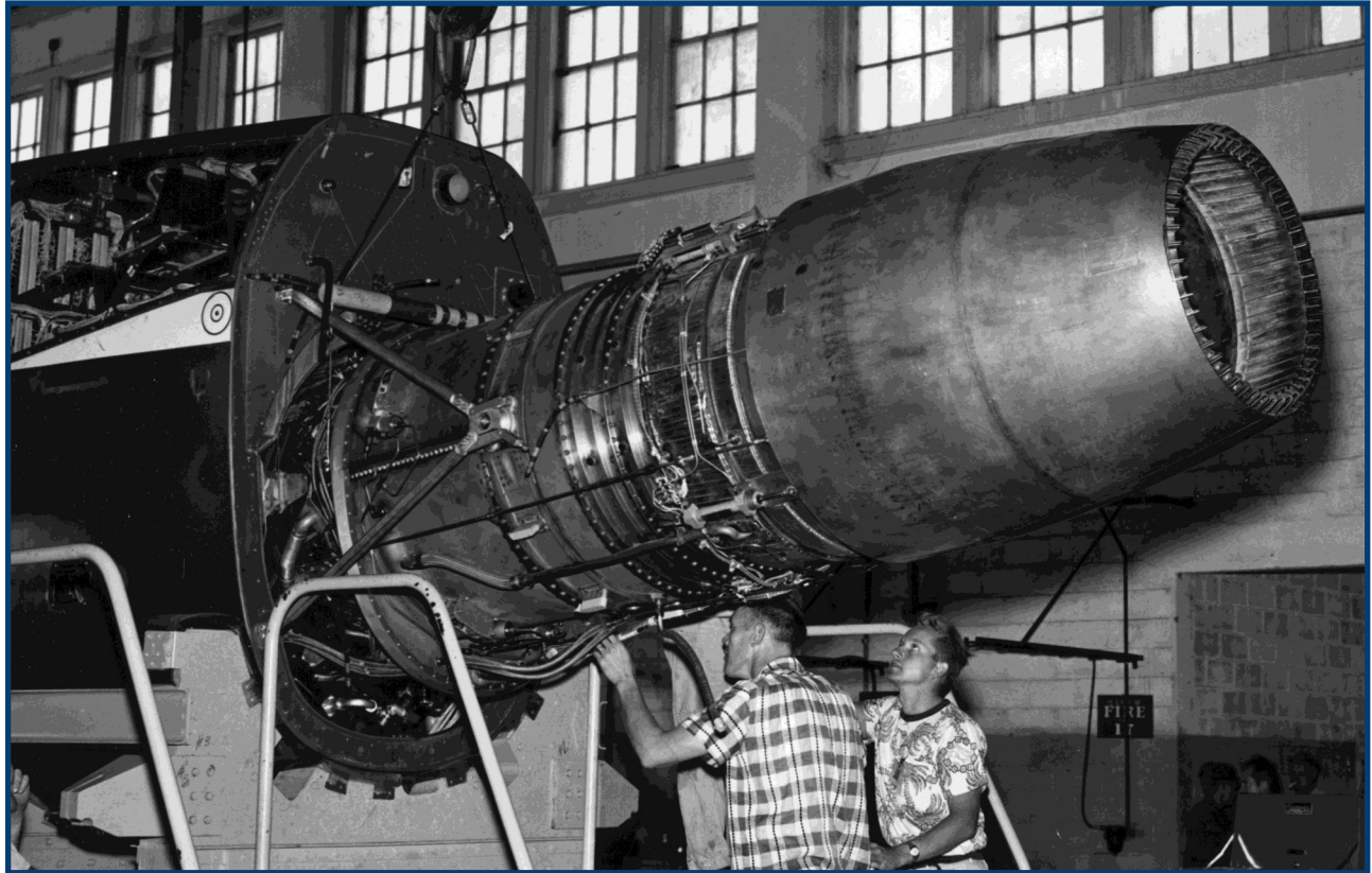
All: Initially powered by an Allison J71 turbojet, later Snarks upgraded to the Pratt & Whitney J57-P-3 and finally the J57-P-17 with 10,500 pounds of thrust.
