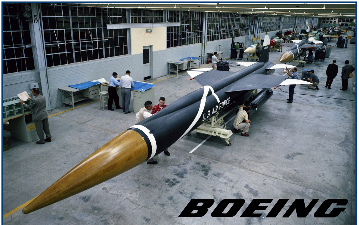
Top: First flown in 1952, the Boeing BOMARC ( B Oeing M ichigan A erospace R esearch C enter) originally carried an F-99 designation, but this changed three years later to IM-99. The XF-99 shown above had the vertical stabilizer on the bottom and did not yet incorporate the ramjet engines for cruise flight.
