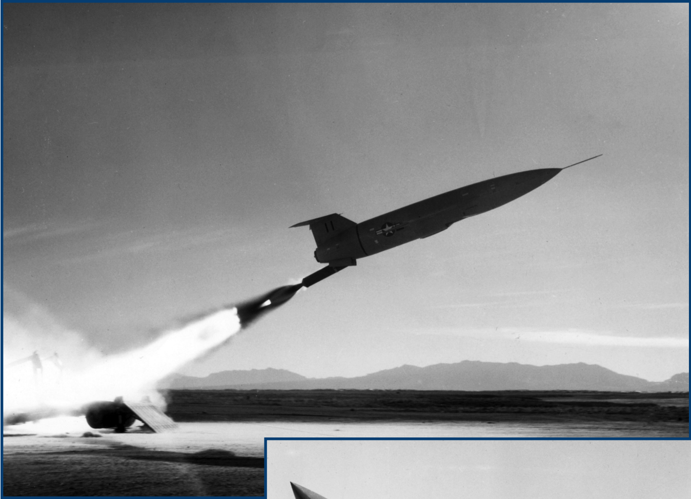
Top and Bottom: With initial test launches performed from a concrete hard stand at the Missile Test Center, latter launches made use of a specially designed mobile platform.
