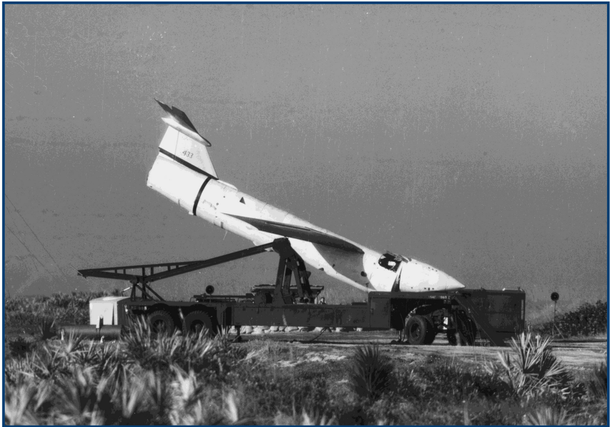
Above: Not all Matador launches went as planned. This missile ended up with moderate damage when it tipped over on its nose prior to launch.
