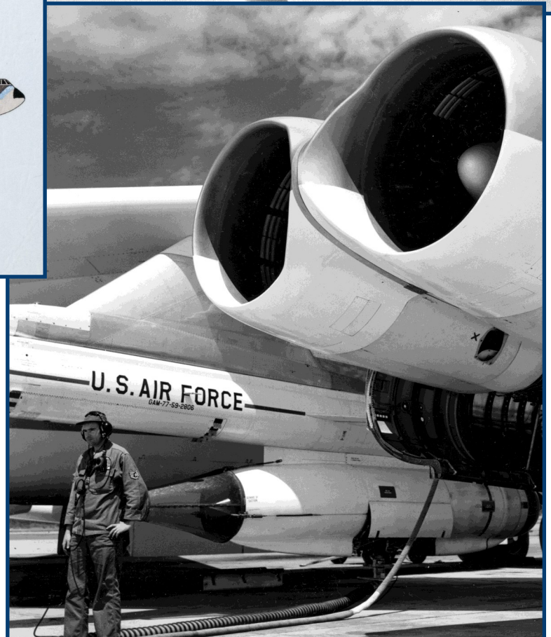
Right: Static engine run on the Hound Dog 's J52 turbojet. Note the FOD cover placed over the intake on the missile to protect the engine from damaging debris.
