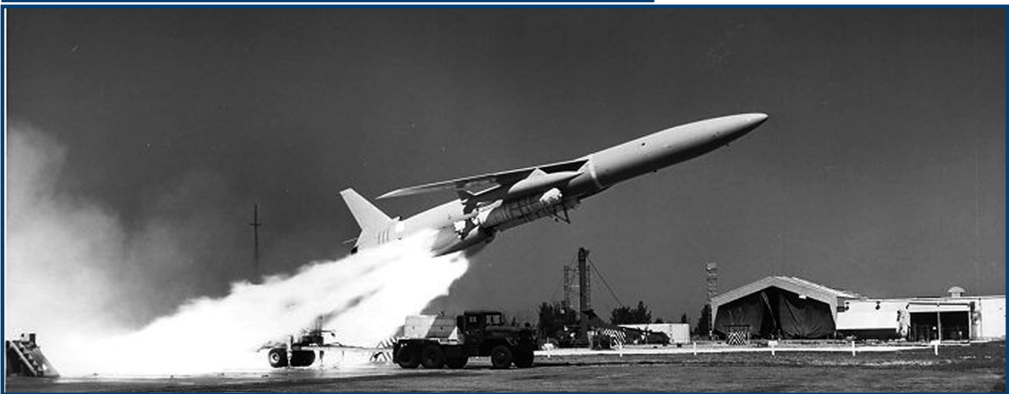
Top Left: Clearly visible in this launch view are the external fuel tanks mounted on each wing of the SM-62 to extend its range.
