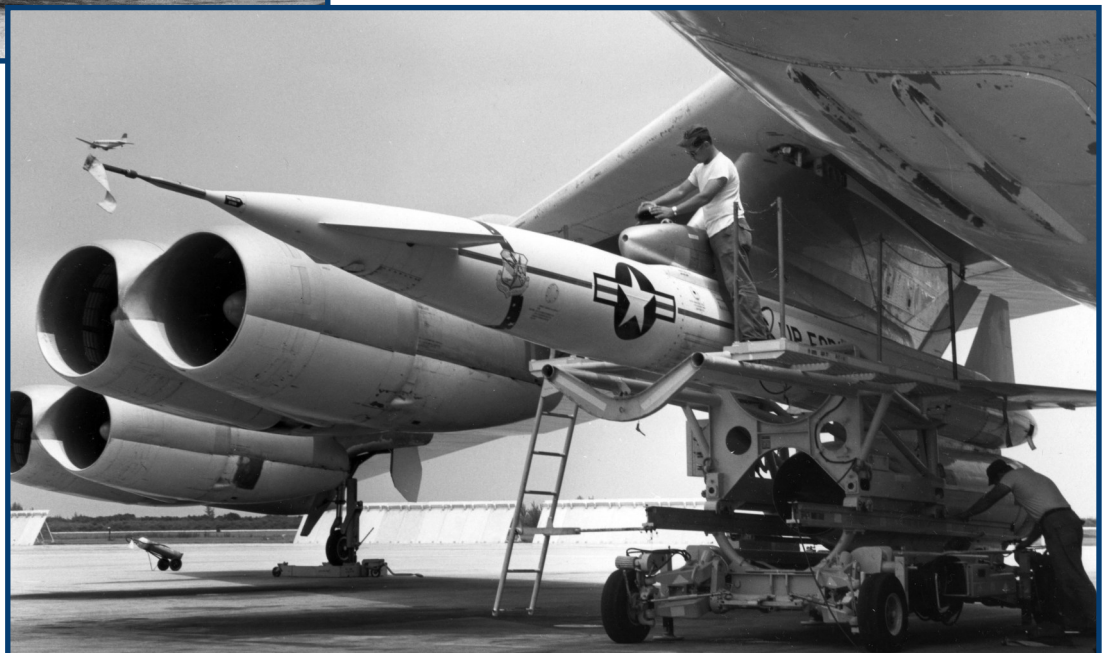
Right: The mobile transport carts for Hound Dog are also used for mounting the missile to the B-52 and contained folding walkways for maintenance personnel.
