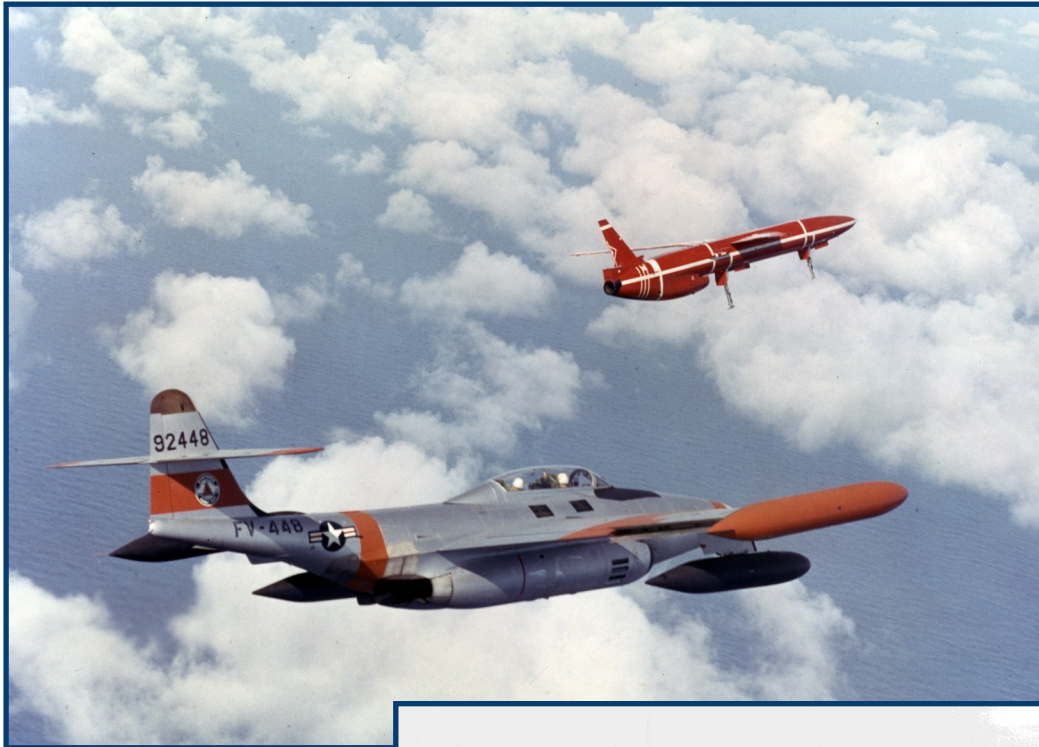
Left: The Northrop F-89 served as an inflight radio control for the N-69 Snark missile after booster release. The landing skids are shown extended as it approaches the Skid Strip at the AFMTC, Cape Canaveral, Florida.
