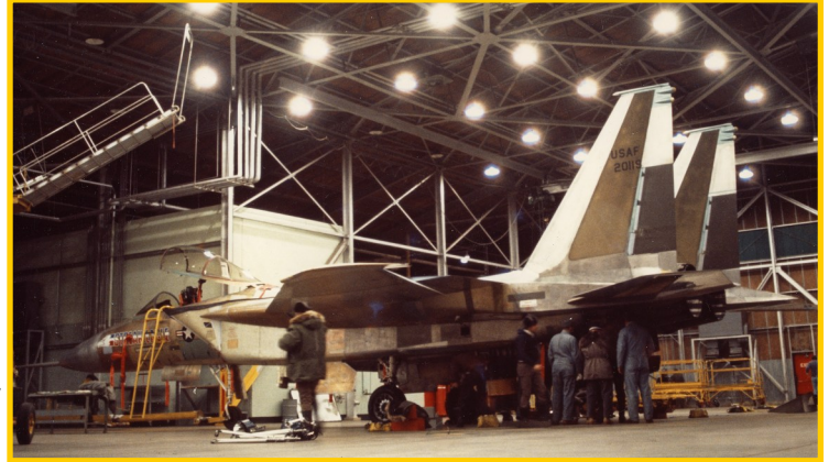
'Streak Eagle' in the hangar at Grand Forks AFB, North Dakota during the record flight attempts. Note the small balancers on top of each vertical stabilizer.
