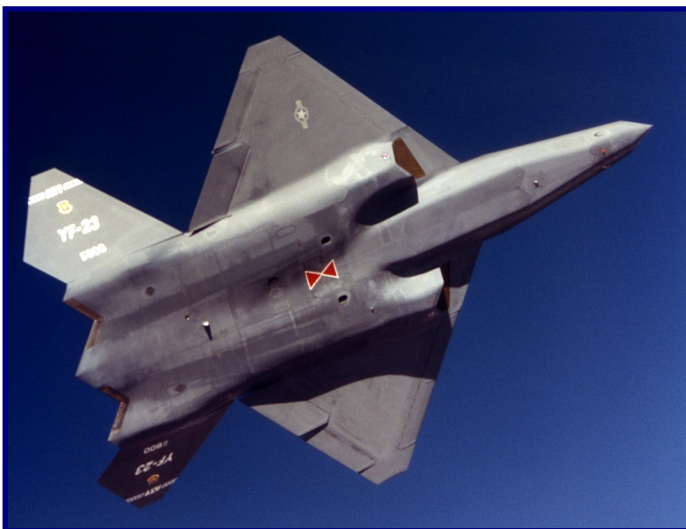
To prevent injury to ground personnel while under the aircraft, the ram air scoop was highlighted with a set of red and white triangles for visibility. The unintended coincidence looked like a Black Widow hourglass while the aircraft was in flight.
