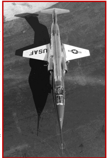
Beautiful overhead view of Lockheed NF-104A 56-0760 which gives a nice perspective of the nose and wing tip modifications made to the Aerospace Trainer aircraft. (AFTC History Office, Edwards AFB)
