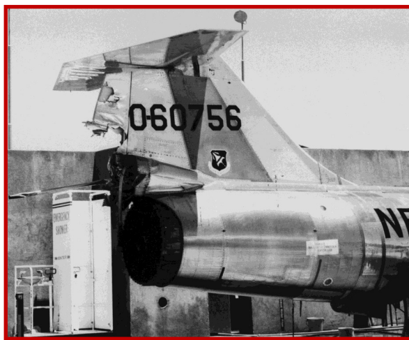
Tail damage of NF-104A #56-0756 on June 15, 1971. (AFTC History Office, Edwards AFB)
