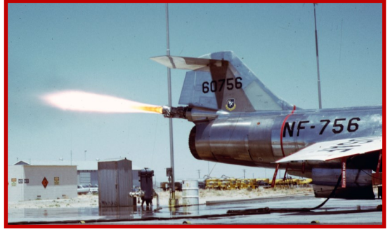
The LR-121-NA-1 rocket engine in NF-104A 56-0762 is test fired on the ground prior to in-flight testing. (Photo by Ed Kopowski ,Sr.)
