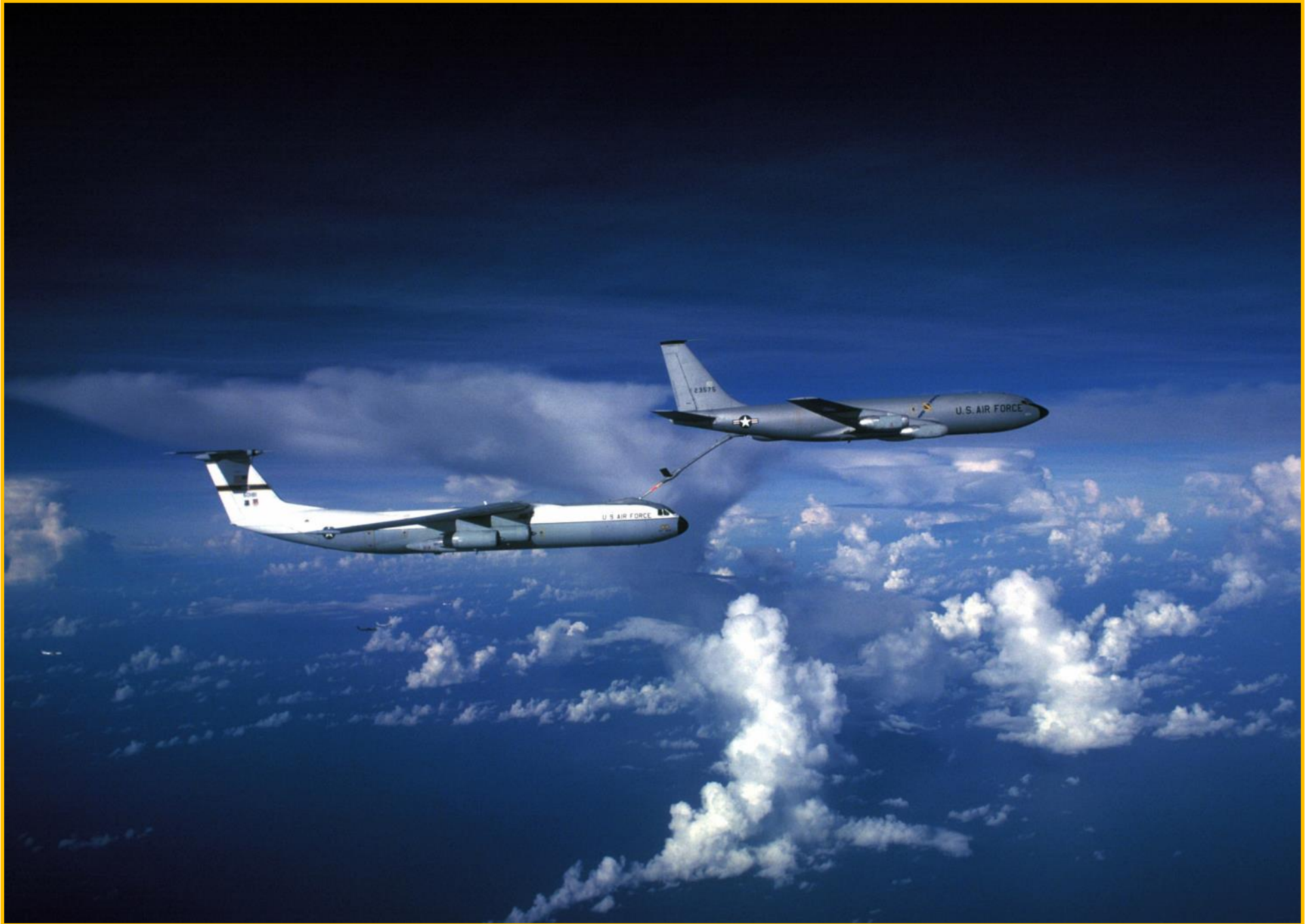
A KC-135A Startotanker #62-3575 provides fuel to C-141B Starlifter #66-0181 during Air Force exercise OCEAN VENTURE '81 on August 8, 1981.
