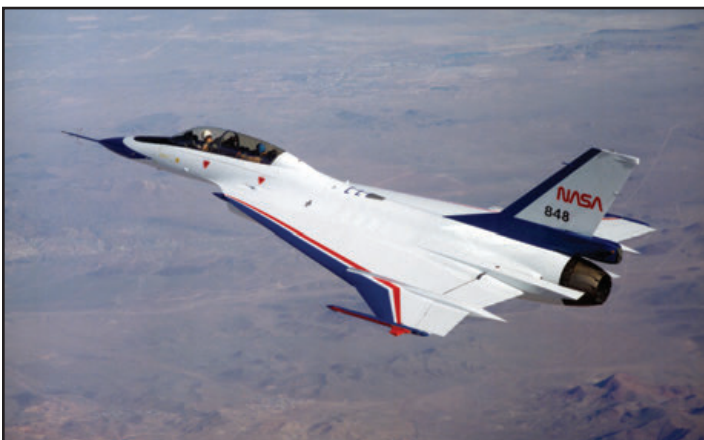
With a bright red, Dynamic Engineering Inc. (DEI) flutter exciter mounted on the left Sidewinder missile rail, NASA 848 performs another test mission from Edwards AFB on 27 February 1992. (NASA)
