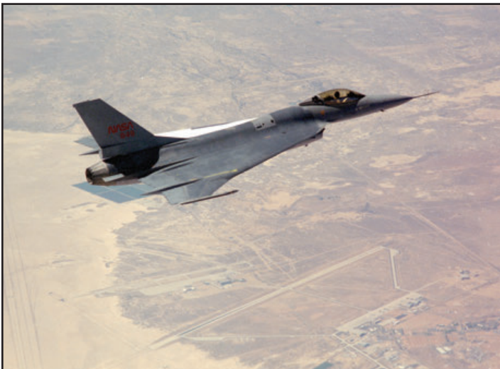
NASA test pilot Steven Ishmael takes F-16XL, NASA 849 up on its first Functional Check Flight (FCF) on 3 May 1990. While adding the laminar flow glove, the small strakes on the wing upper surface were removed. The medium gray panel in front of the in-flight refueling receptacle covers the suction pump assembly for the wing glove. (NASA- all)
