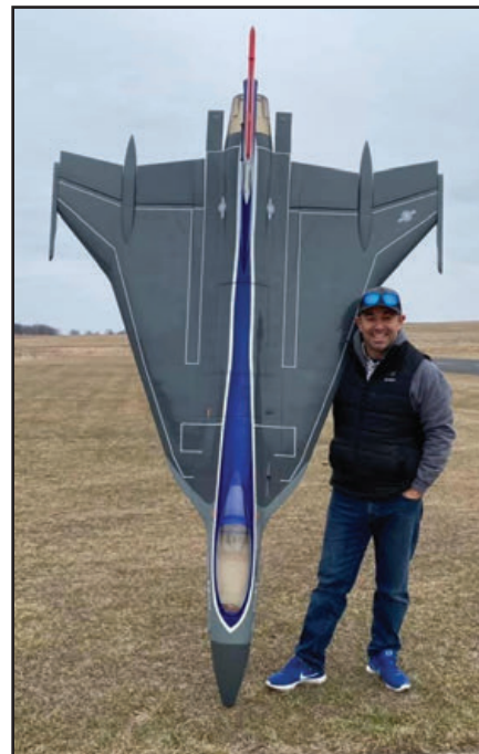
A 1/6th scale remote control (R/C) F-16XL made by Global Knight Models. The model measures 108 inches long with a 70 inch wingspan. (Global Knight Models)
