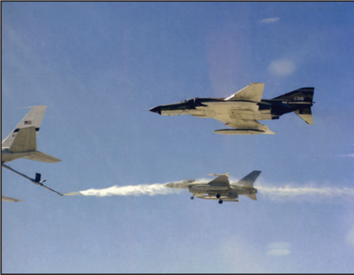
F-16A 75-0749, performs water ingestion testing behind a modified KC-135 on 19 August 1978. (AFTCHistoryOffice)
