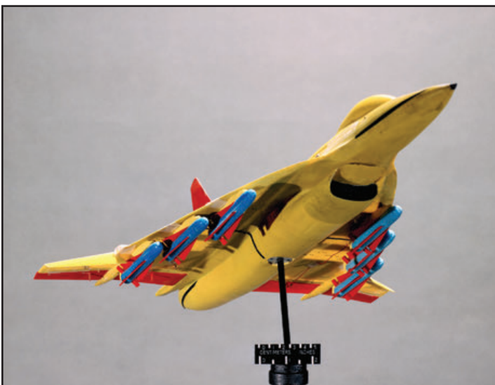
NASA Langley tested a variety of external store configurations including six AGM-65 Mavericks. (NASA Langley)
