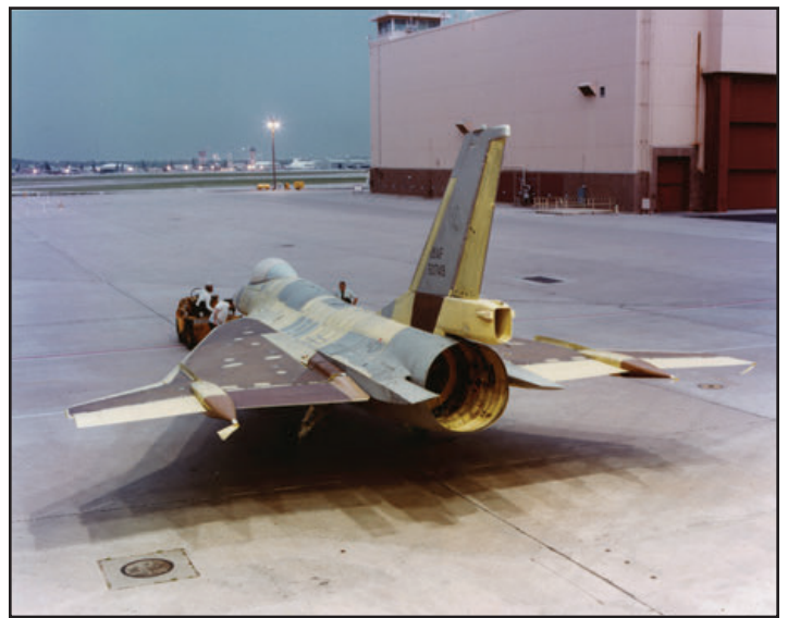
With loads testing successfully completed, the F-16XL, went through final assembly of the air-frame having the control surfaces, landing gear, nose radome and other internal components installed. The aircraft is shown here heading to the paint shop during May 1982. (Lockheed Martin)
