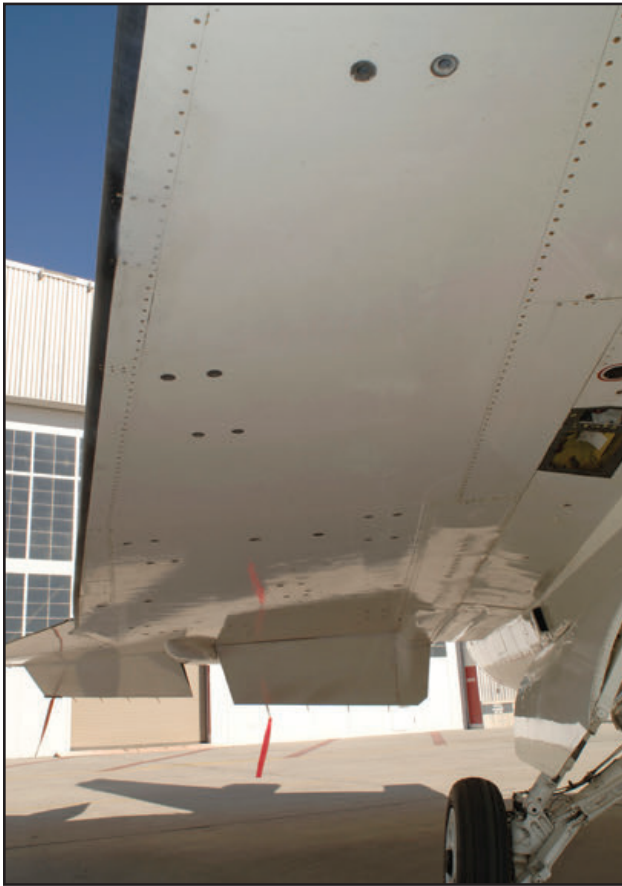
Wing hardpoints were built into the underside of the wing for the carriage of additional weapons or fuel tanks, while the fuselage is modified to allow for semi-submerged AMRAAM missiles. (Tony Landis)
