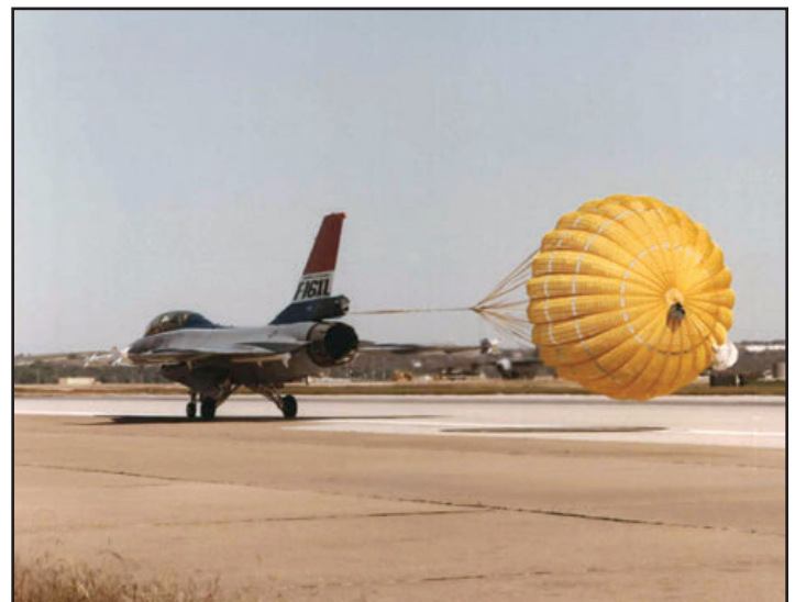
Taxi testing for the second F-16XL in October 1982, slowly building up to the final high-speed taxi on 30 October. At the end of the high-speed taxi, the braking parachute deployment was tested. (Lockheed Martin)
