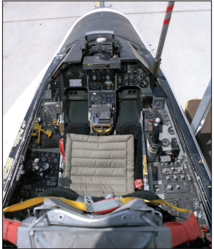
The series of images on this page and the following page show the front and aft cockpits of XL-2 in July 1996, near the end of the NASA test program. Note the addition of the white GPS antenna in front of the HUD, and controls for the Supersonic Laminar Flow experiment in the aft cockpit. (Tony Landis)
