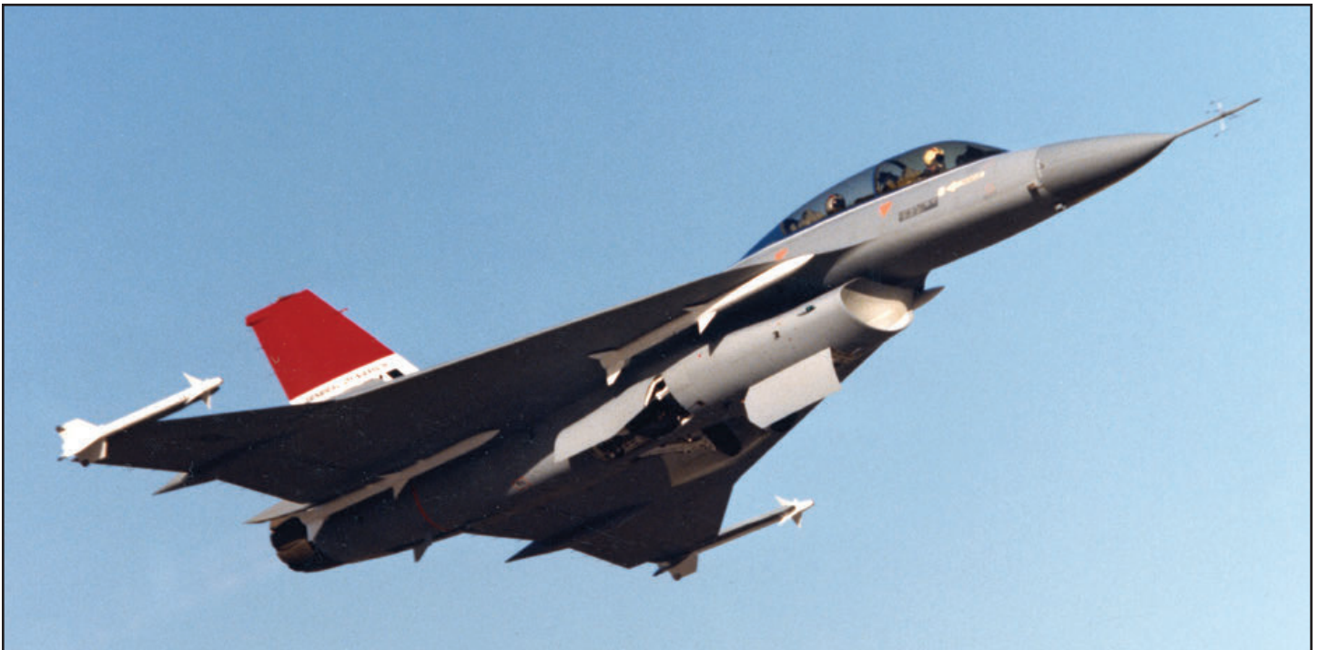
While the single-seat F-16XL, 74-0749, was powered by the Pratt & Whitney F100-PW-200, the two-seat aircraft, 75-0747, made use of a single General Electric F101-GE-102 powerplant. This was replaced by an F110-GE-100 'Slimline' engine in mid-July 1984. (Sheryl Tierney collection- top; Keith Svendsen collection- above)
