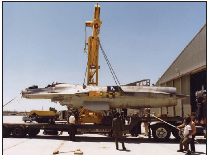
The Air Force made use of F-16A 75-0749 for early climatic testing, putting the FSD airframe through extreme heating and cold tests inside the McKinley Climatic Laboratory at Eglin AFB, FL. (USAF)
