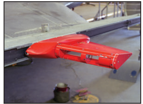
The use of the DEI flutter exciter on the wingtip of the F-16XL's, provides dynamic force input to stimulate structural vibration modes. (NASA)
