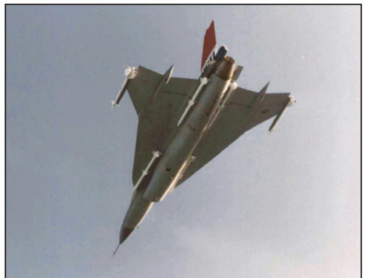
A series of images taken during the third flight of the F-16XL on 17 July 1982. Clearly visible is the lack of ventral stabilizing fins on the lower aft fuselage of the F-16XL. With the extended fuselage and new wing design, the ventral fins were no longer required for lateral stability. (Lockheed Martin)
