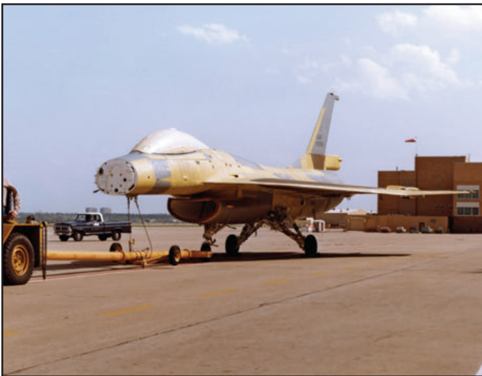
With the modifications complete, the first F-16XL is moved to the General Dynamics loads testing facility for static proof testing on 2 April 1982, as seen in the four photos above and single image below left. (Lockheed Martin)
