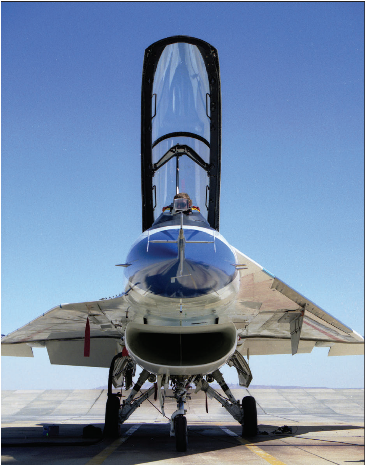
The asymmetric design of the wings on NASA 848 during the SLFC program show up well in this view. (NASA)
