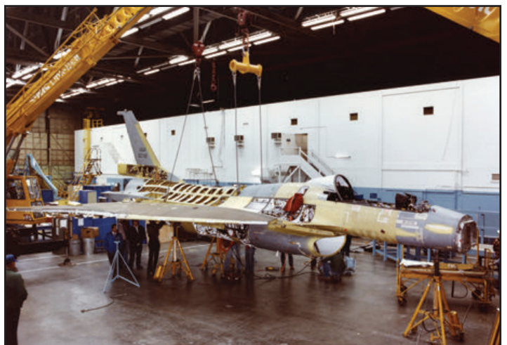
The first airframe, 75-0749, (also referred to as XL-1) is shown in the demate jig on 22 July 1981 in the photo at top left. Gaps for the fuselage extensions are easily viewed. By 23 March 1982, the modified airframe was beginning to look like the F-16XL as seen in the additional four photos on this page. (Lockheed Martin)
