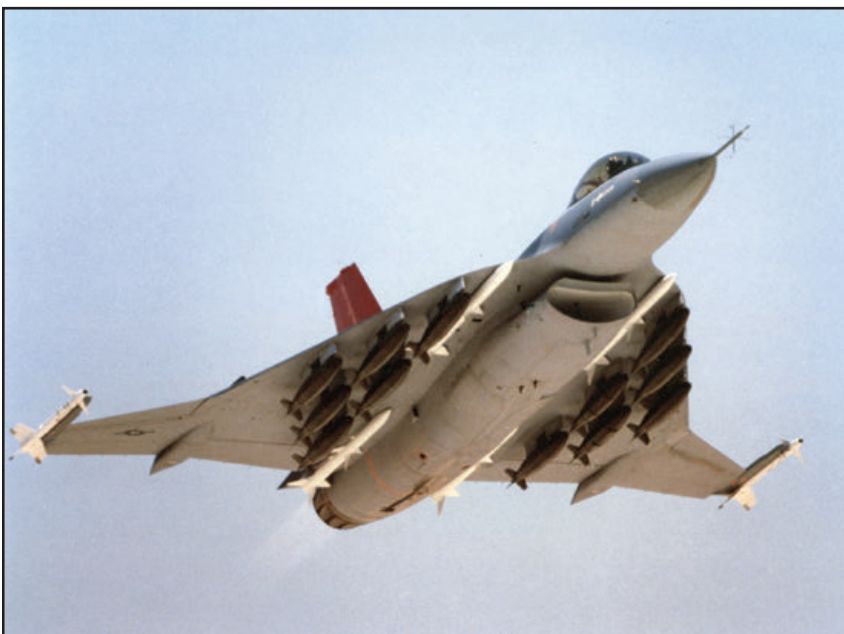
A typical air-to-ground mission load consisted of 12-Mk82, 500 pound, free-fall, gravity bombs attached to Lode 14 wing pylons. (Lockheed Martin- above; Keith Svendsen- right)
