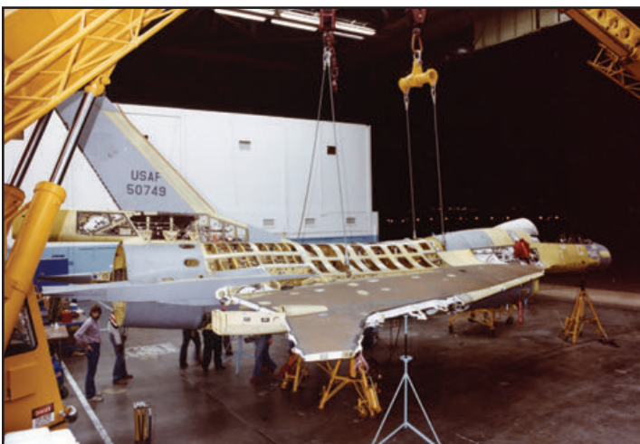
The first airframe, 75-0749, (also referred to as XL-1) is shown in the demate jig on 22 July 1981 in the photo at top left. Gaps for the fuselage extensions are easily viewed. By 23 March 1982, the modified airframe was beginning to look like the F-16XL as seen in the additional four photos on this page. (Lockheed Martin)
