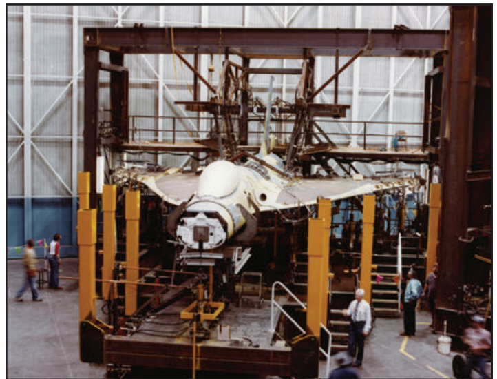
Initial ground testing began with main fuselage loads and flexibility tests conducted in specially constructed loads test rig at General Dynamics. (Lockheed Martin)
