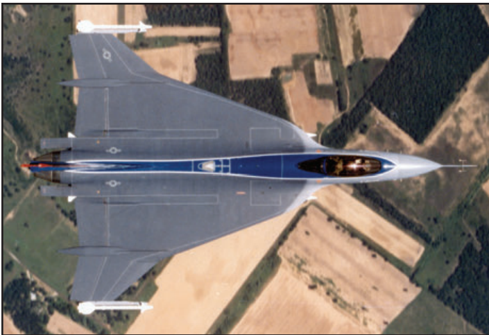
The gray walkway striping and other stenciling applied over the FS36118 dark gray and blue were FS36231 gray. When the demonstrator markings were painted over in March 1983, the vertical stabilizer received a coat of FS36270 gray. (Lockheed Martin- top, left; Keith Svendsen- top, right)
