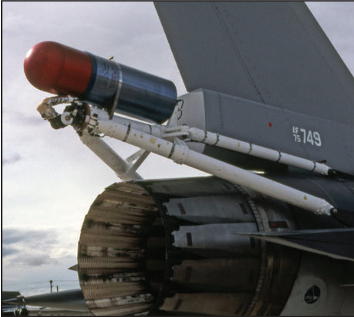
Close-up detail of the spin chute modification on F-16XL, 75-0749 on 3 March 1983. Note that the drag chute box has been blocked off and the tail of the aircraft is now overall gray with white serial number. (Keith Svendsen)
