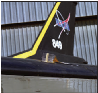
While NASA 848 performed testing on the SLFC wing glove, F-16XL NASA 849 continued testing various experiments added to the upper surface of the wings beginning in November 1995 and continuing into the following year. Boundary layer measurement rakes and hot film instrumentation were added in January and February 1996. (NASA- all)
