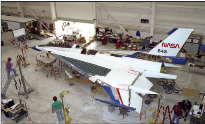
Boeing completed assembly of the SLFC wing glove and delivered it to NASA on 17 December 1994 (top 2). NASA technicians quickly went to work installing the wing glove attachment fittings to NASA 848 (middle 4). Once the adhesive cured, the attachment fixture was removed and passive glove fairings installed in March 1995. (NASA- all)
