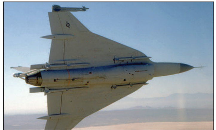
Sporting a fresh coat of paint, F-16XL 75-0749 is equipped with the spin chute assembly for additional high AoA testing on 7 August 1984, piloted by Lt. Col. Edwin Thomas. (Keith Svendsen- both above)
