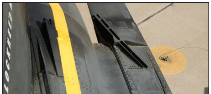
F-16XL, 75-0749, was taken out of service for 10 days in late January 1983 for installation of a spin chute assembly prior to high AoA testing. (Lockheed Martin- above; Tony Landis- 2 at right)
