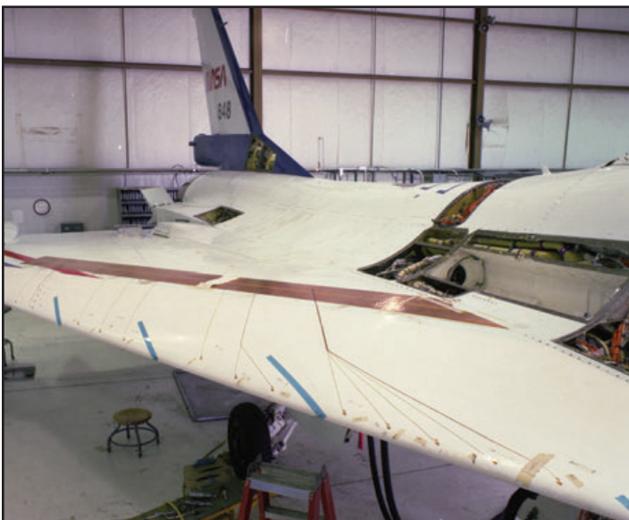
In the 5 photos above, NASA 848 receives a passive wing glove modification and associated instrumentation during July & August 1992. (NASA)
