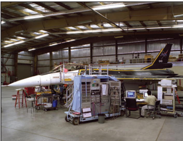
F-16XL NASA 849 is set up for ground vibration testing inside NASA hangar 4826 on 16 January 1997. (2 at top and above). (NASA)
