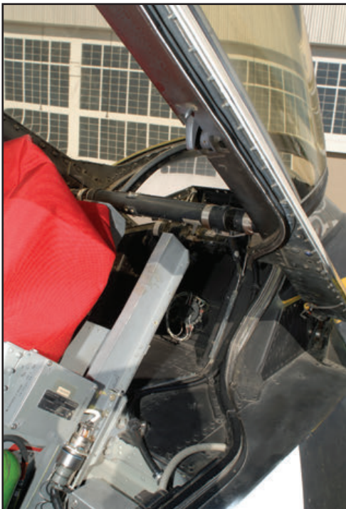
Left and right side cockpit consoles, Aces II ejection seat and aft cockpit area details of F-16XL, 75-0749. The custom red cover, and black, sheep skin padding on the seat were unique to the NASA flight test program. (Tony Landis)
