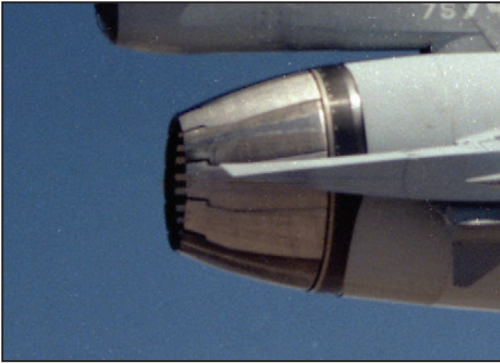
There was no discernible external difference in the engine exhaust nozzle of the GE F110 'Slimline' and F110-GE-129 engines. (Keith Svendsen- top left; NASA- top right)
