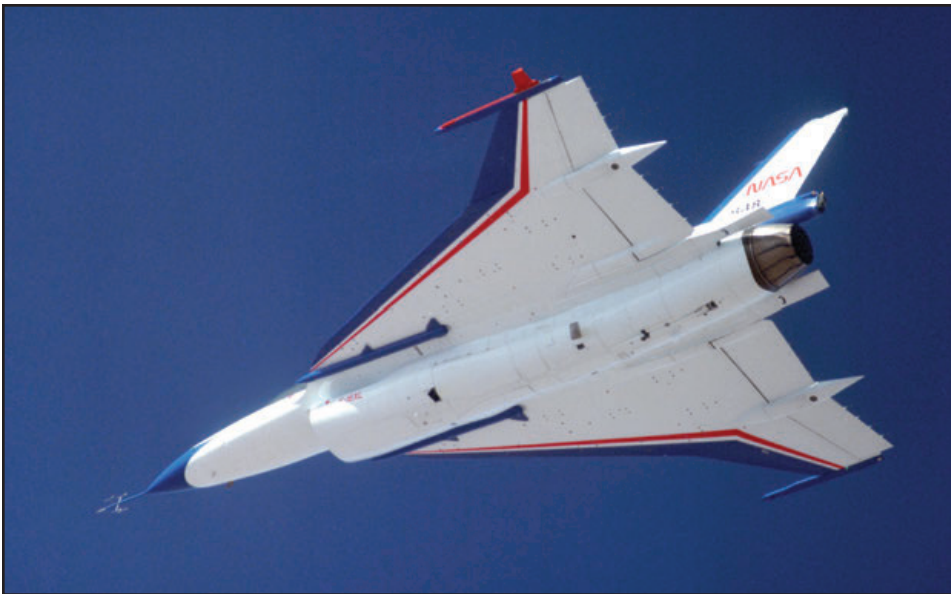
The use of the DEI flutter exciter on the wingtip of the F-16XL's, provides dynamic force input to stimulate structural vibration modes. (NASA)
