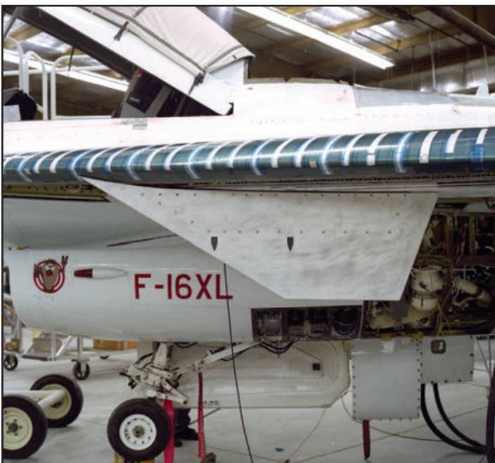
Test instrumentation and the associated orange wire dominated the interior of the F-16XL with the wing glove installed (top left). The turbo compressor exhaust vented out the right side of the aircraft (top right). A larger shock fence under the left wing replaced those on both wings. Note the Tasmanian Devil logo on the inlet. (above). NASA added test instruments to the upper left side of both front and aft cockpit control panels. (2 at right) (NASA- all)
