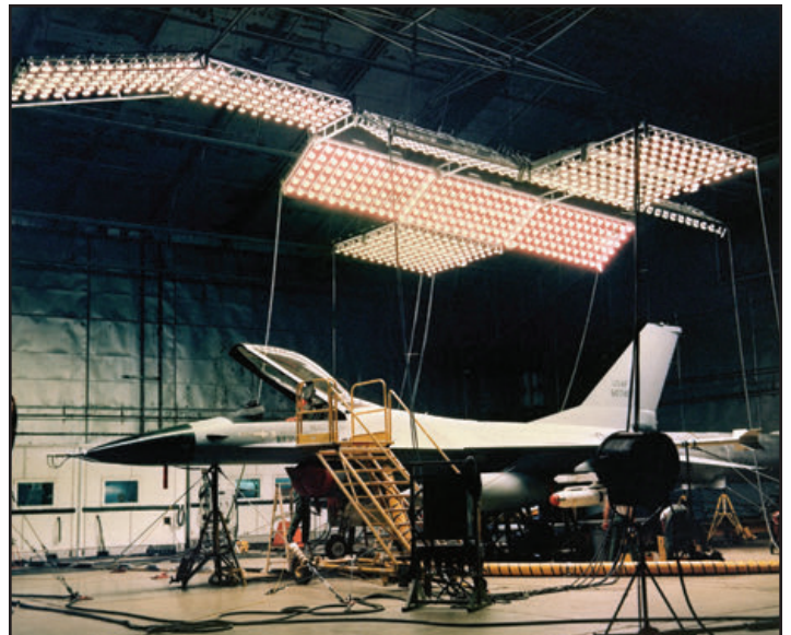
The Air Force made use of F-16A 75-0749 for early climatic testing, putting the FSD airframe through extreme heating and cold tests inside the McKinley Climatic Laboratory at Eglin AFB, FL. (USAF)
