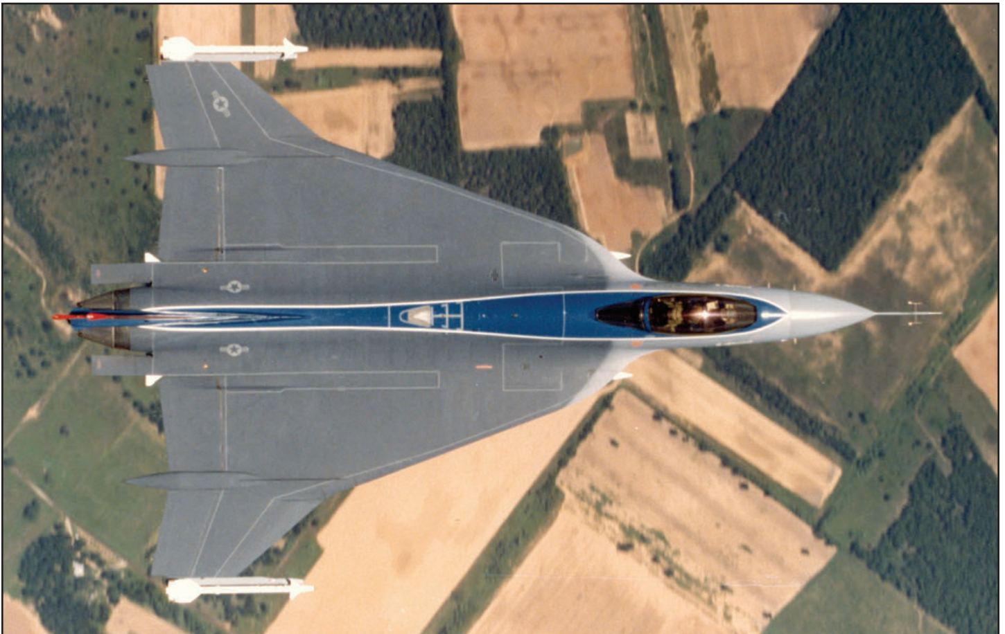
In addition to the 115 percent increase in wing area, the fuselage length was extended by 56 inches with a 30-inch plug added at fuselage station 189, and a 20-inch plug at fuselage station 373. (Lockheed Martin)
