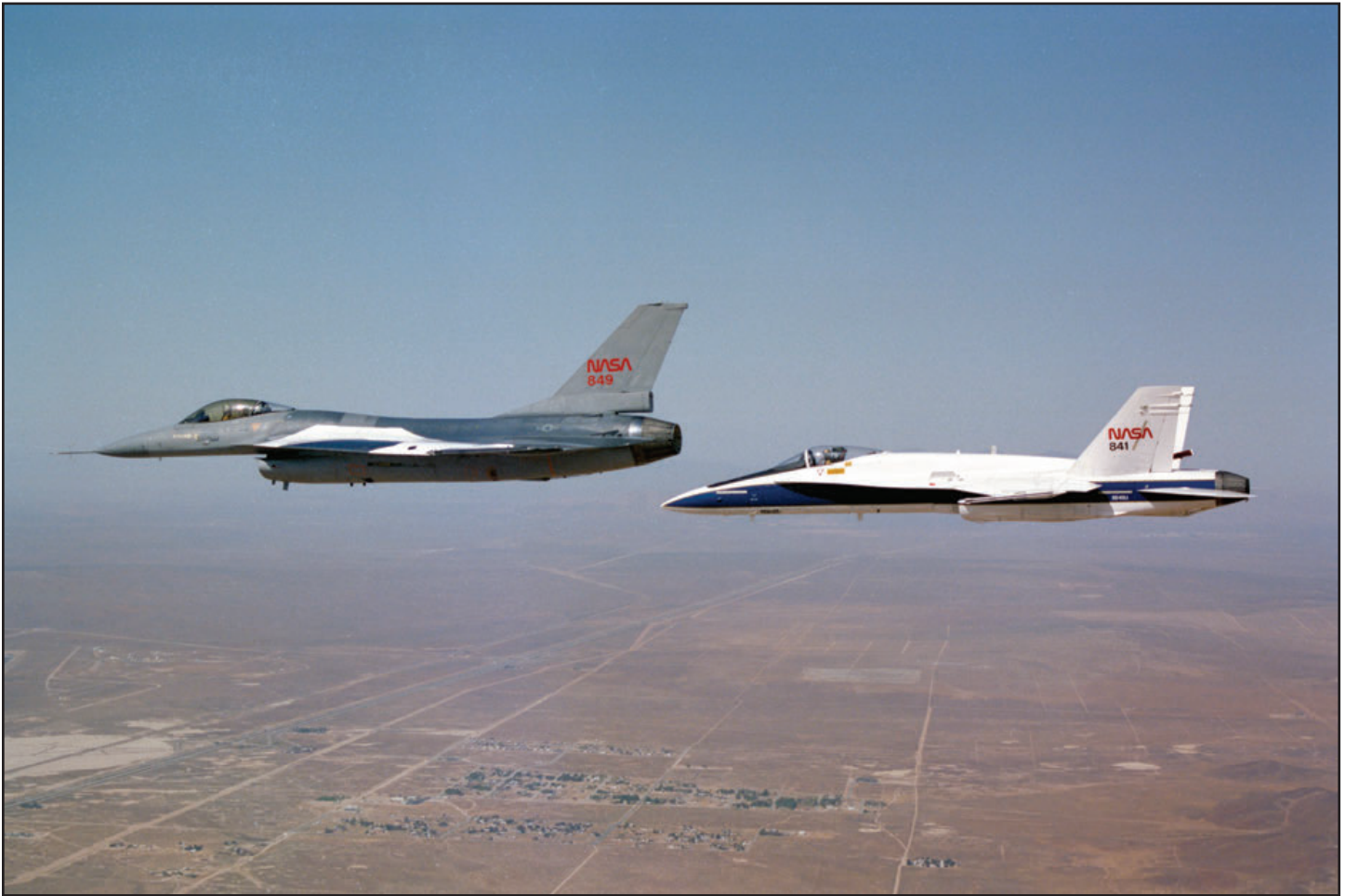
With its speed brake partially open, a safety chase F/A-18A, NASA 841, pulls in close to F-16XL NASA 849 during a test mission near Edwards AFB on 11 September 1991. (NASA)
