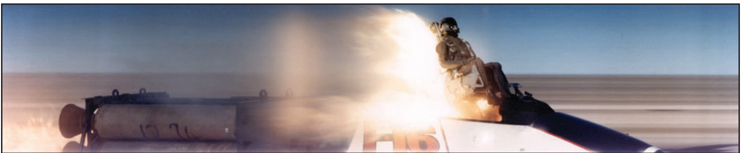
Rocket-propelled F-16 ejection seat test of the McDonnell Douglas ACES II ejection seat at the High-Speed Test Track, operated by the 846th Test Squadron at Holloman AFB, New Mexico. (USAF Photo)
