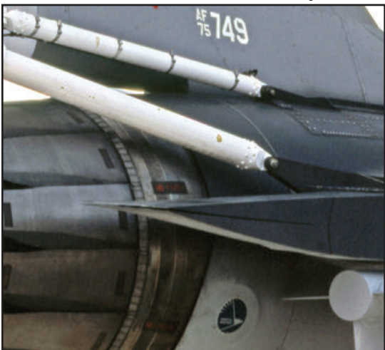
The gray walkway striping and other stenciling applied over the FS36118 dark gray and blue were FS36231 gray. When the demonstrator markings were painted over in March 1983, the vertical stabilizer received a coat of FS36270 gray. (Lockheed Martin- top, left; Keith Svendsen- top, right)
