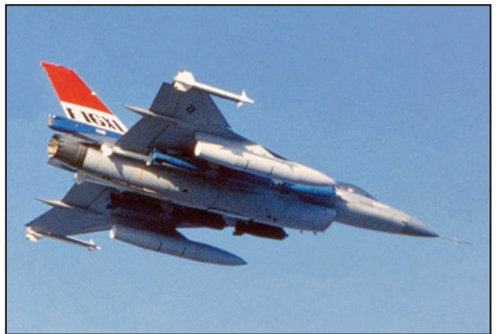
Taken during test missions on 13 December and 17 December 1982, the photos above, and the following page, show F-16XL, 75-0749, carrying a load of 6-CBU-58 cluster bombs and 2-370 gallon wing tanks in addition to the dummy AMRAAM's and Sidewinders. (Michael Grove, Sr.-2 at top; Keith Svendsen-3 above and 4 on following page)
