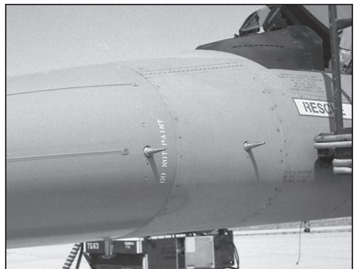
Various probes located on the left and right sides of the forward fuselage on the F-16XL include Angle-of-Attack, Total Temperature and Pitot probe. Note 'Do Not Paint' stencil on radome. (Keith Svendsen- both)
