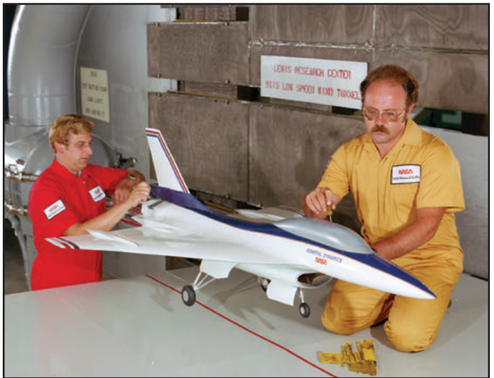
NASA's Lewis Research Center (now Glenn Research Center) in Cleveland, OH, was responsible for propulsion and engine inlet design testing. NASA Lewis made use of the 9 x 15 foot Low-Speed Wind Tunnel. (NASA Glenn)
