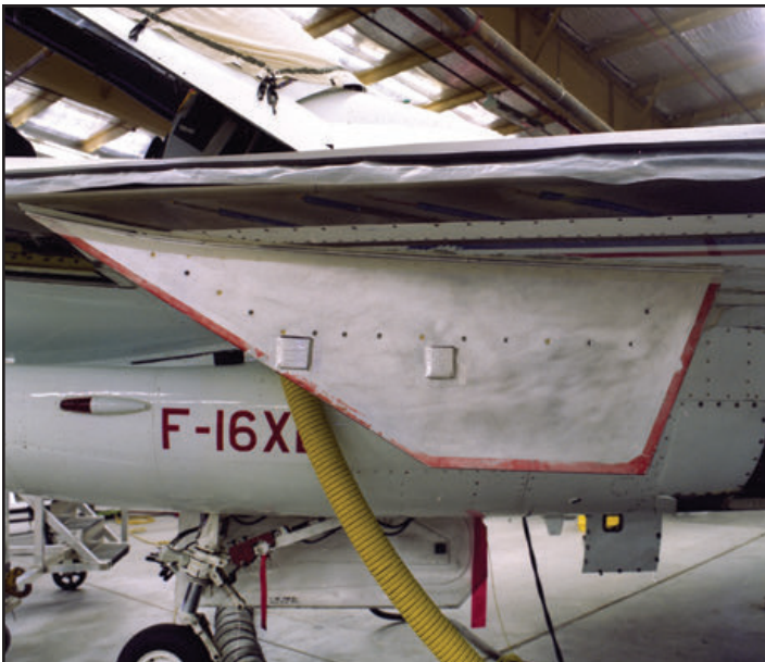
A smaller, highly swept, shock fence design mounted on NASA 848 on 8 October 1996. (NASA)
