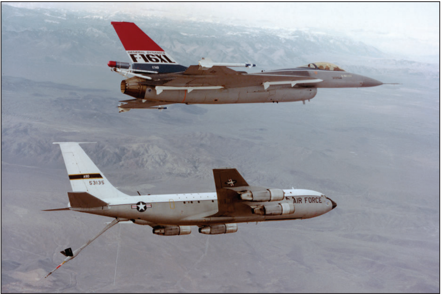
Moving into close formation with the NKC-135E Stratotanker prior to taking on fuel, the F-16XL is shown during a 2.5 hour high AoA mission on 14 February 1983. (Sheryl Tierney collection)
