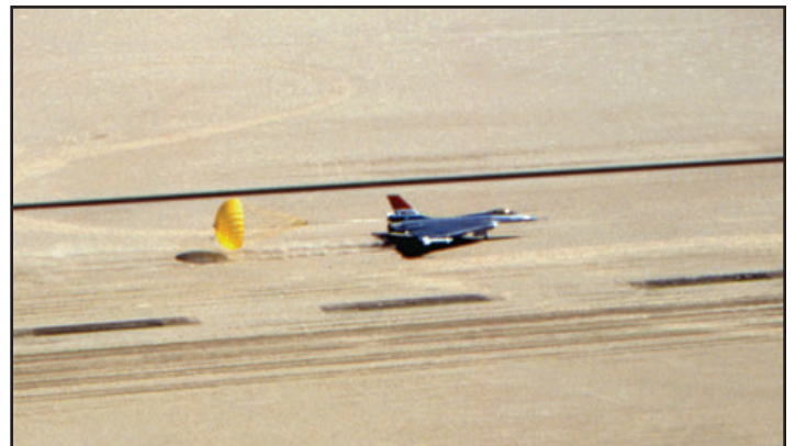
During a test mission on 3 August 1982, the F-16XL suffered a failure of the left hand speedbrake actuator and began leaking hydraulic fluid. The pilot made a precautionary landing on the dry lakebed at Edwards. (Keith Svendsen)
