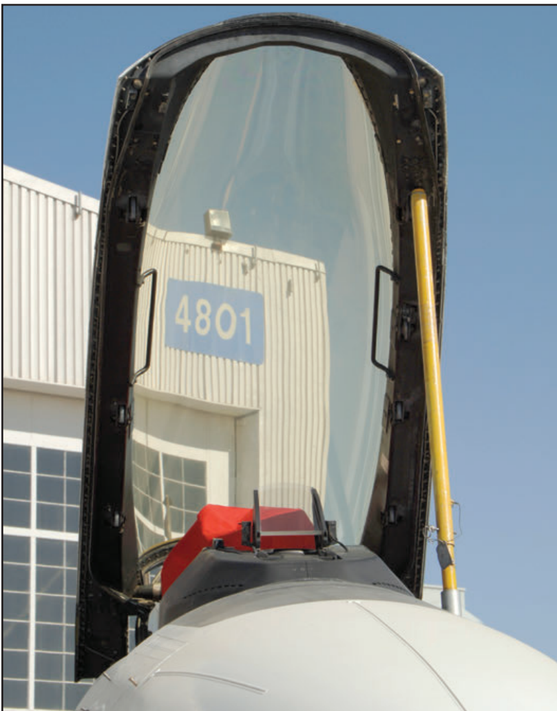
The two-piece plastic canopy used on the F-16XL was identical to those on the standard F-16A/B models. An inflatable pressurization seal on the cockpit sill mates with the edge of the movable canopy, while a non-inflatable rubber seal on the canopy prevents water entry. (Tony Landis)
