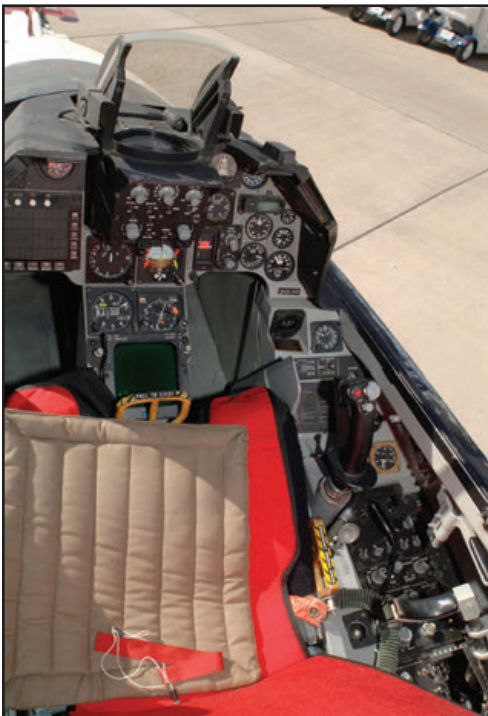
Left and right side cockpit consoles, Aces II ejection seat and aft cockpit area details of F-16XL, 75-0749. The custom red cover, and black, sheep skin padding on the seat were unique to the NASA flight test program. (Tony Landis)
