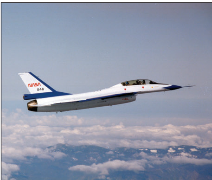
F-16XL NASA 848 during a test mission on 9 March 1992. Note the forward canopy section is clear while the aft canopy section is gold-tinted. A common practice on early two-seat F-16's. (NASA)
