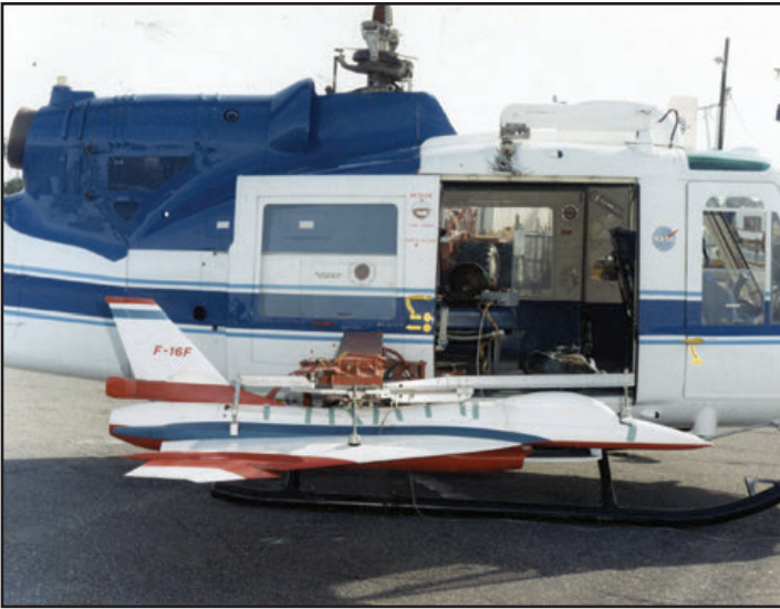
Testing the spin characteristics of the General Dynamics F-16XL design required the use of large scale models released from a NASA UH-1 helicopter over the Atlantic ocean and recovered via parachute at the end of each test mission. Note the model above carries an F-16F designation. (NASA Langley)
