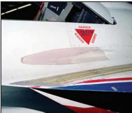
During May and June 1993, NASA technicians added more instrumentation, a modified leading edge, gun bay cover and shock fences under each wing to F-16XL NASA 848. (NASA- 6 above)
