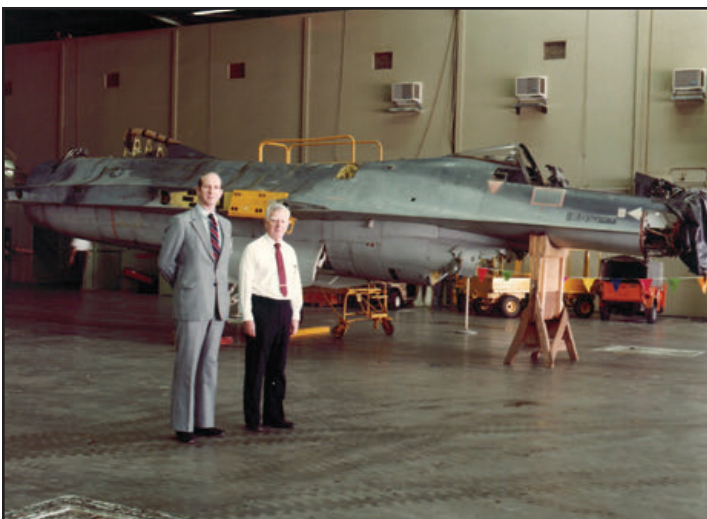
Performing during the annual open house at Edwards AFB on October 31, 1980, F-16A, 75-0747, suffered a blown nose tire on takeoff. The pilot chose to make an emergency landing on the dry lakebed and the aircraft was substantially damaged when the nose gear collapsed. The airframe was returned to General Dynamics via C-5 Galaxy and rebuilt as the two-seat F-16XL. (Lockheed Martin)
