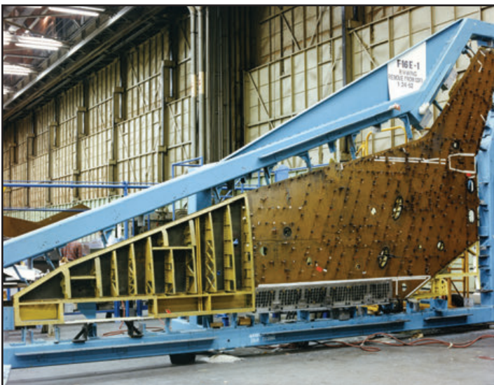
Just a year after first metal was cut, the completed right wing assembly is ready for installation on the first F-16XL, 75-0749 on 24 January 1982. (Lockheed Martin)
