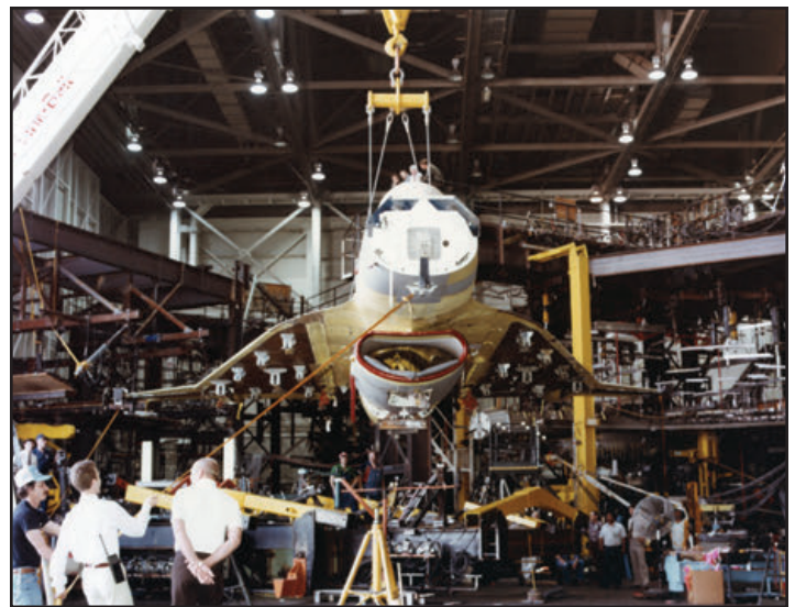
Once fuselage testing was completed, the first F-16XL aircraft was positioned for testing of the new wing design structure on 14 April 1982. Note the many hydraulic attach points on the lower wing surface. (Lockheed Martin)
