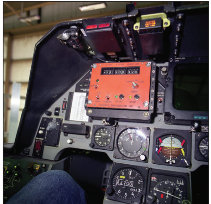
The front and aft cockpits of F-16XL, NASA 848, on 18 October 1991, show some instrument changes required for the Supersonic Laminar Flow Control program. Note the weapon control panel has been removed from the front instrument panel (above left). (NASA)
