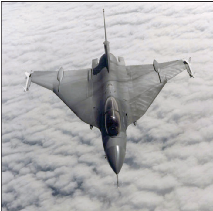
Officially known as Deceptive Camouflage, or Splinter Camouflage, this particular variation, which included a false canopy and upper surface markings applied to the bottom of the aircraft, was the brainchild of aviation artist Keith Ferris. Ferris designed many variations of the Splinter scheme that were tested on various aircraft during the 1970's and 1980's. (Lockheed Martin)
