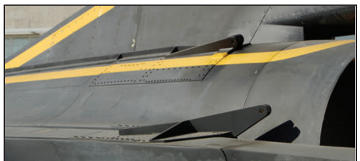
The dorsal fairing of the vertical stabilizer contained a Norwegian-type drag chute system with an increased area of 19-foot diameter, gold-color canopy. (Lockheed Martin- above left; Tony Landis- 2 above)
