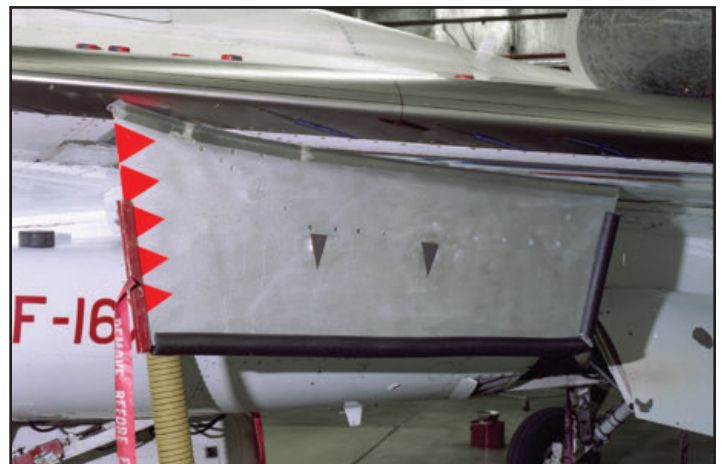
The shock fence design was changed a few times during the course of the SLFC project. The red markings and black foam were to prevent injury while on the ground. (NASA)
