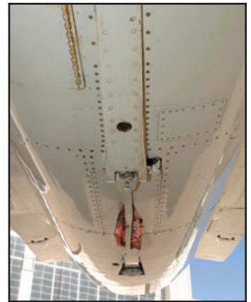
The 2 ventral fins carried by standard F-16's were not required on the F-16XL due to the lengthened fuselage. Standard F-16 tail hook arresting assembly is located in aft fuselage. (Keith Svendsen- above, left; Tony Landis- 2 above)
