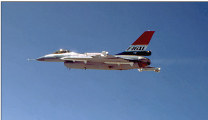
During a test mission on 3 August 1982, the F-16XL suffered a failure of the left hand speedbrake actuator and began leaking hydraulic fluid. The pilot made a precautionary landing on the dry lakebed at Edwards. (Keith Svendsen)
