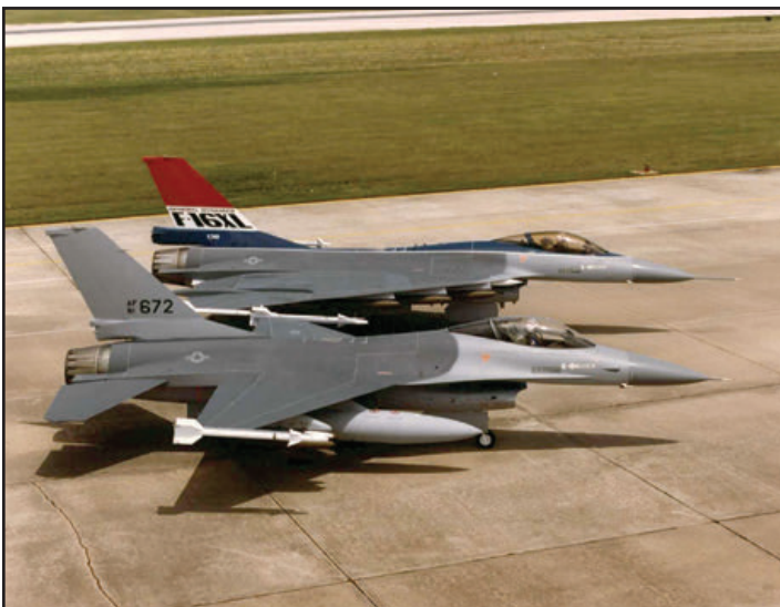
F-16XL 75-0749 is parked next to F-16A 81-0672 on the ramp in Ft. Worth. Both aircraft are configured for a typical air-to-ground mission. The F-16A required two external wing tanks and carried only 6-Mk82's, while the F-16XL could perform the same mission with twice the payload and no external tanks. (Lockheed Martin)
