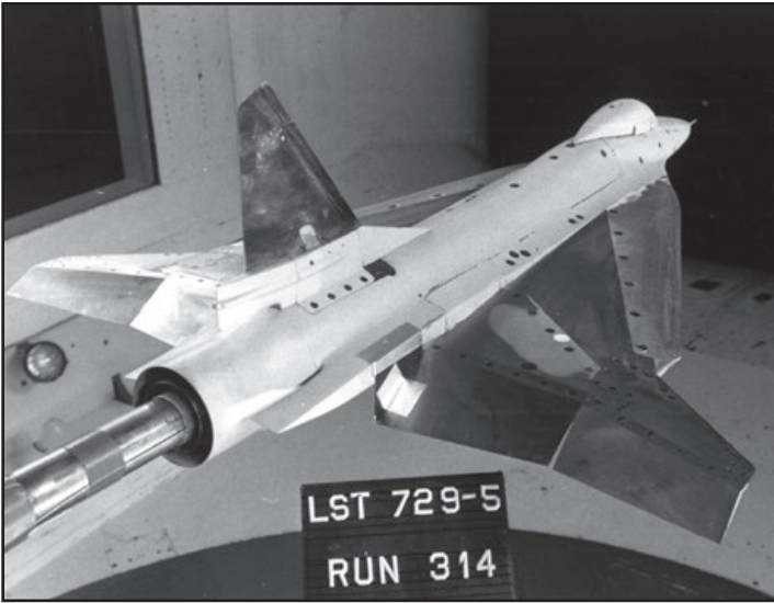
To check for power loss to control surface gaps, a gap sealer is placed on the inboard edge of the right elevon prior to run 314. (Robert Bradley collection)
