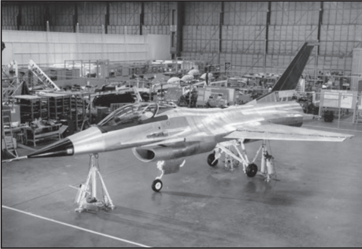
The first YF-16 under construction at the General Dynamics facility in Ft. Worth, TX. (Lockheed Martin)
