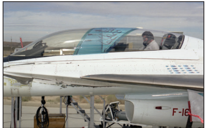
Prior to a research mission on 12 September 1996, NASA engineers attempted to modify the airflow over the canopy by adding thin foam covered in blue tape (above and far left). A portion of this section failed during the flight (left). Airflow tufts were also added near the back of the canopy. NASA technician, Bob Cummings, runs checks from the aft seat of the F-16XL (above). Note the different shock fence in the photo above left. (NASA- all)
