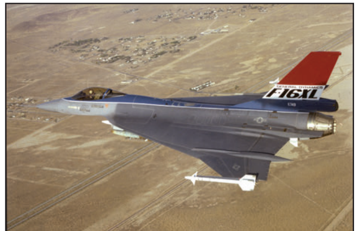
Beginning 13 October 1982, F-16XL, 75-0749, began a series of 11 stability & control, and weapon separation tests with 6 Mk82 bombs. The small white objects mounted on the trailing edge fairings are camera pods used for filming the bomb release. (AFTC History Office)
