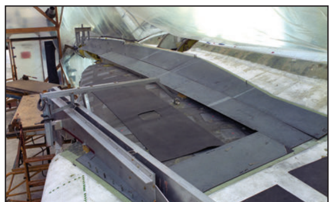
Modifications to NASA 848 began in July 1993 and continued over the next two years. The forward structure for the new wing is shown above. (NASA- all)
