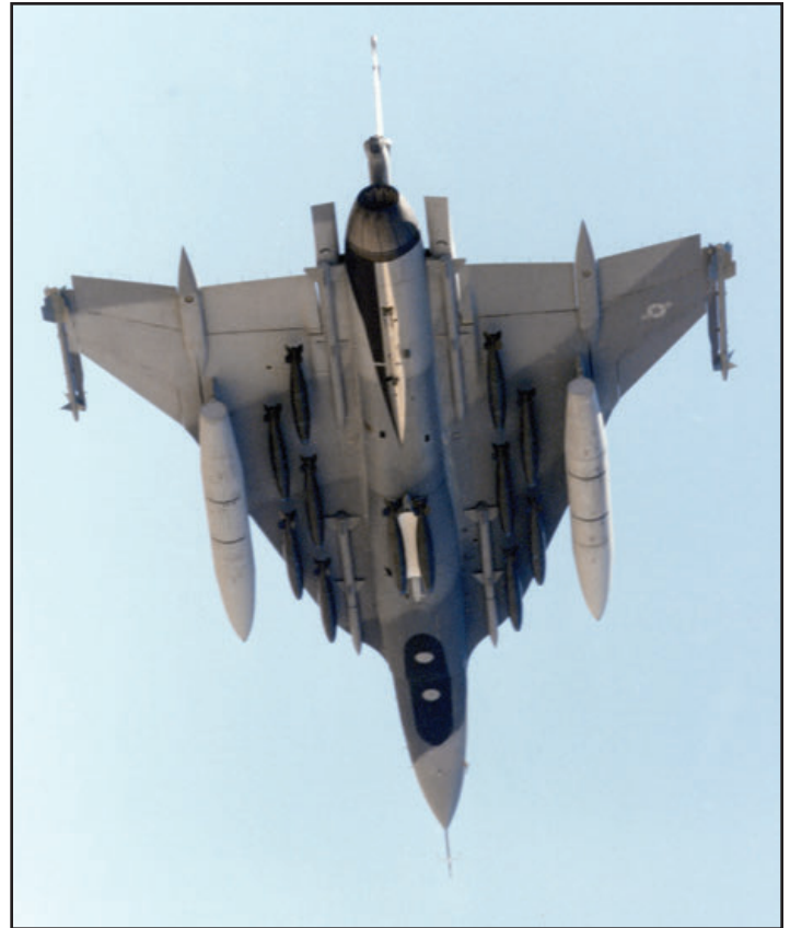
F-16XL, 75-0747, flew 2 missions on 14 July 1983 with a weapon load of 12-Mk82 bombs, 5 under each wing and 2 mounted on the centerline station, along with 2-370 gallon fuel tanks. (Lockheed Martin)
