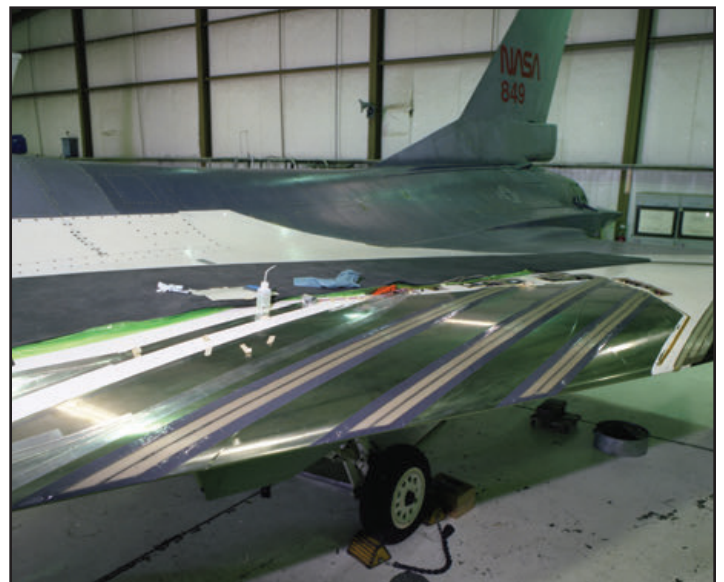
Active SLFC wing glove on F-16XL NASA 849 with instrumented strip tubes installed on 28 August 1992. (NASA)
