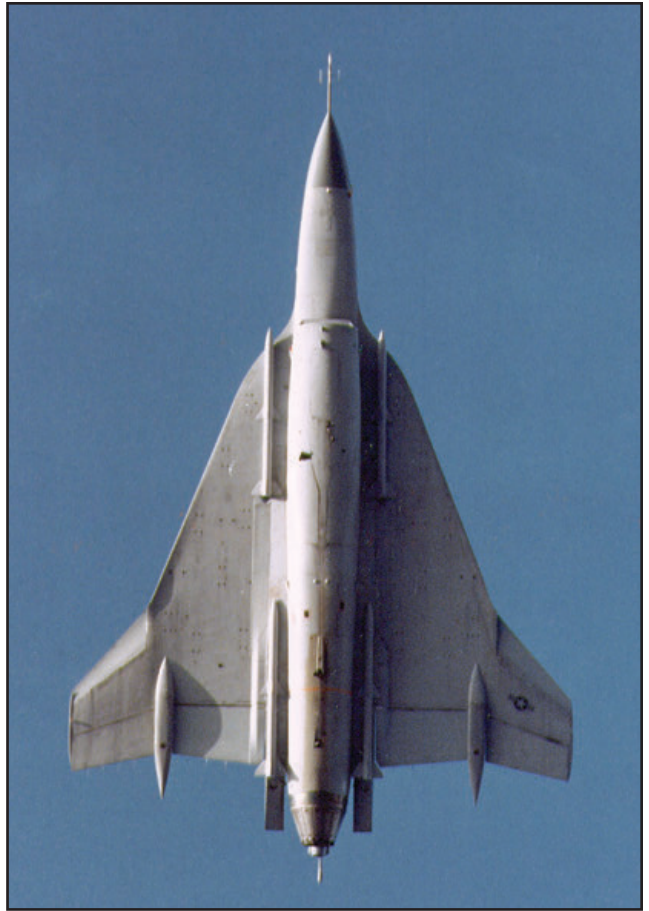
Both F-16XL aircraft performed test missions with wingtip fairings in place of the Sidewinder missile rails as shown in the photo above taken on 23 March 1983 of F-16XL, 75-0749. (Lockheed Martin via Mike Moore)
