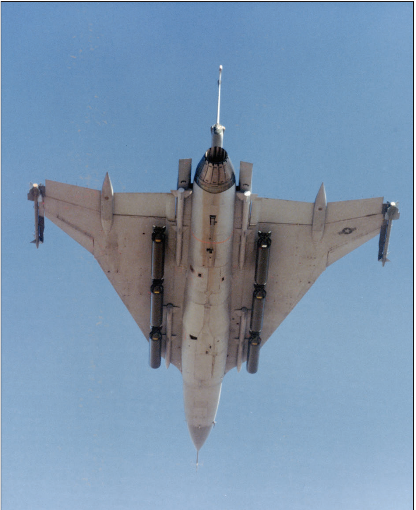
Clean bottom view of F-16XL, 75-0749, taken on 20 July 1983 during a performance test mission out of Edwards AFB while carrying 6-SUU-65, free-falling cluster bombs. Note the missing control tabs on the aft fins of the dummy Sidewinder missiles. (Sheryl Tierney collection)
