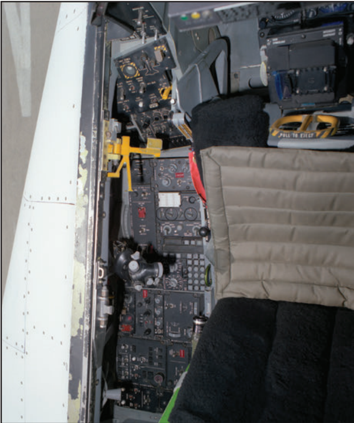
The series of images on this page and the following page show the front and aft cockpits of XL-2 in July 1996, near the end of the NASA test program. Note the addition of the white GPS antenna in front of the HUD, and controls for the Supersonic Laminar Flow experiment in the aft cockpit. (Tony Landis)
