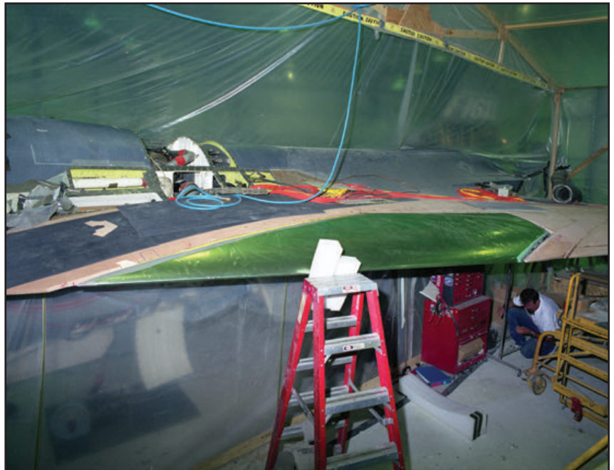
As seen in these images taken on 21 July 1989, NASA technicians immediately went to work installing the small laminar flow wing glove on the left wing of XL-1, soon to be bearing serial number NASA 849. (Lockheed Martin)
