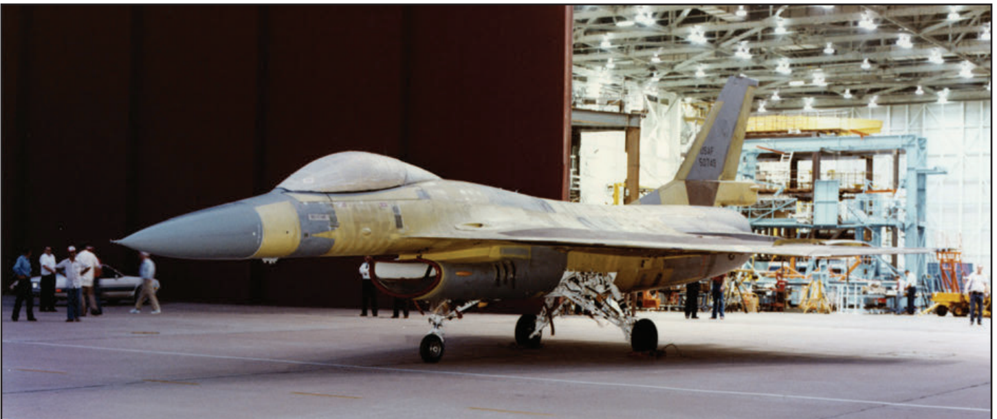
With loads testing successfully completed, the F-16XL, went through final assembly of the air-frame having the control surfaces, landing gear, nose radome and other internal components installed. The aircraft is shown here heading to the paint shop during May 1982. (Lockheed Martin)
