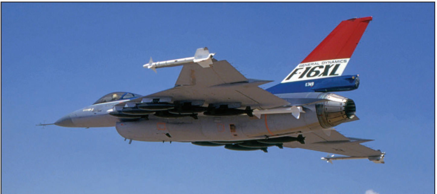
F-16XL, 75-0749 performed 4 flights over 2 days in order to conduct performance testing with 12 Mk82 bombs prior to actual weapon release testing. (AFTC History Office, 2 at center; Keith Svendsen, above)
