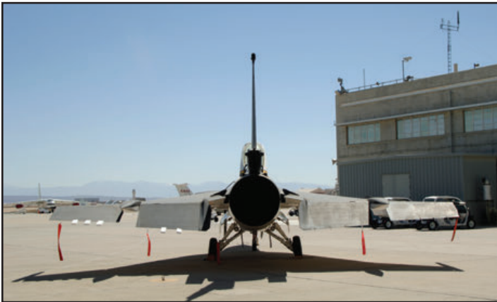
The wing is made up of graphite polyimide composite skins attached to an aluminum under-structure, each incorporating independently-actuated elevon and aileron for pitch and roll control. Leading edge flaps are installed outboard on leading edge sweep break. (Tony Landis)
