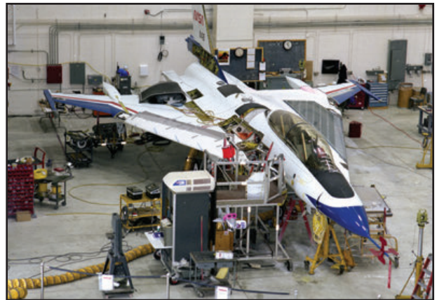
Boeing completed assembly of the SLFC wing glove and delivered it to NASA on 17 December 1994 (top 2). NASA technicians quickly went to work installing the wing glove attachment fittings to NASA 848 (middle 4). Once the adhesive cured, the attachment fixture was removed and passive glove fairings installed in March 1995. (NASA- all)
