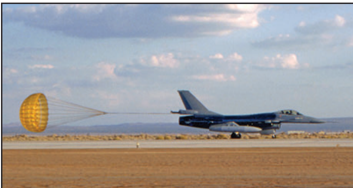
Streaming its distinctive gold braking parachute, F-16XL, 75-0749, comes in to land at Edwards AFB after a brief test mission on 28 October 1983. (Keith Svendsen)
