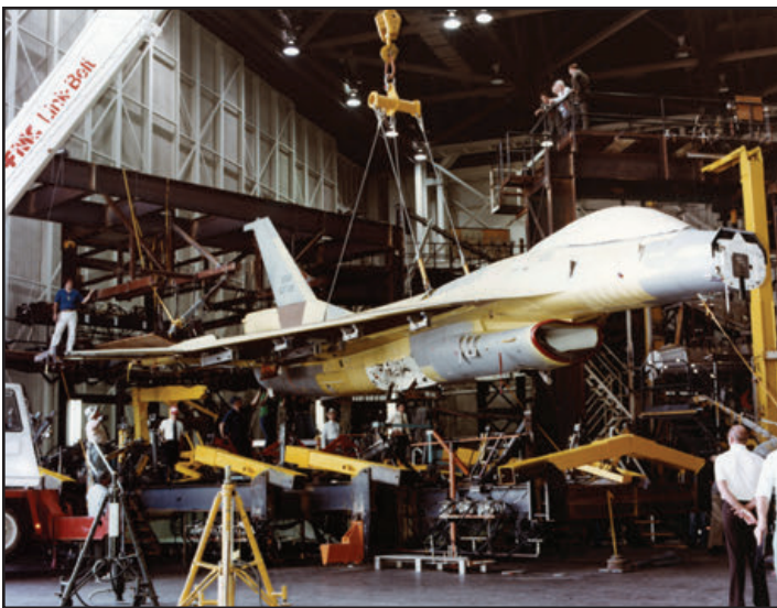
Once fuselage testing was completed, the first F-16XL aircraft was positioned for testing of the new wing design structure on 14 April 1982. Note the many hydraulic attach points on the lower wing surface. (Lockheed Martin)
