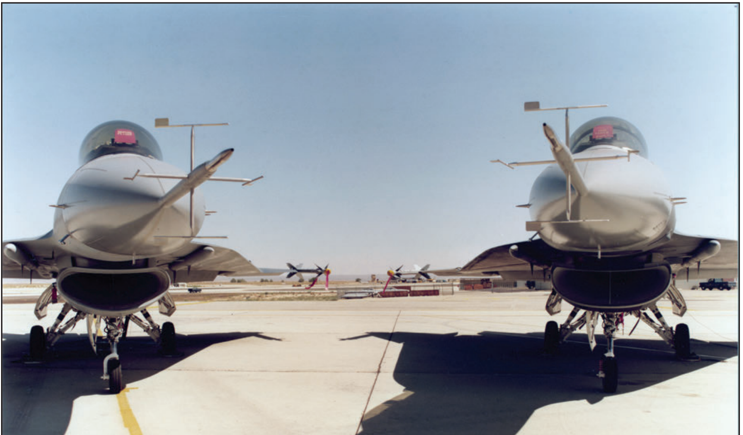
With both F-16XL's parked together at Edwards AFB, a good comparison can be made between the standard inlet on 75-0749 (left) and the LNSI on 75-0747 (right). (Sheryl Tierney collection)
