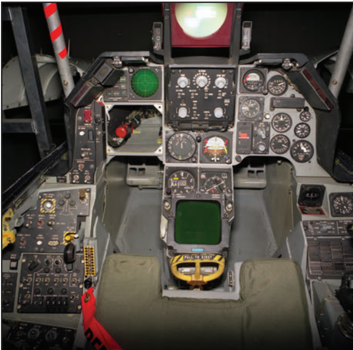
The front and aft cockpits of F-16XL, NASA 848, on 18 October 1991, show some instrument changes required for the Supersonic Laminar Flow Control program. Note the weapon control panel has been removed from the front instrument panel (above left). (NASA)
