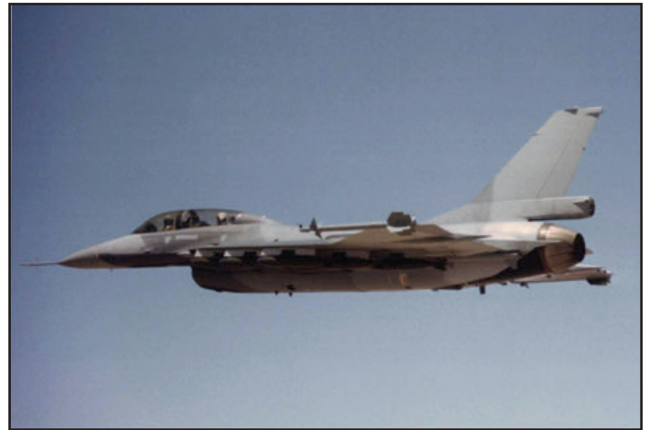
F-16XL, 75-0747, flew 2 missions on 14 July 1983 with a weapon load of 12-Mk82 bombs, 5 under each wing and 2 mounted on the centerline station, along with 2-370 gallon fuel tanks. (Lockheed Martin)
