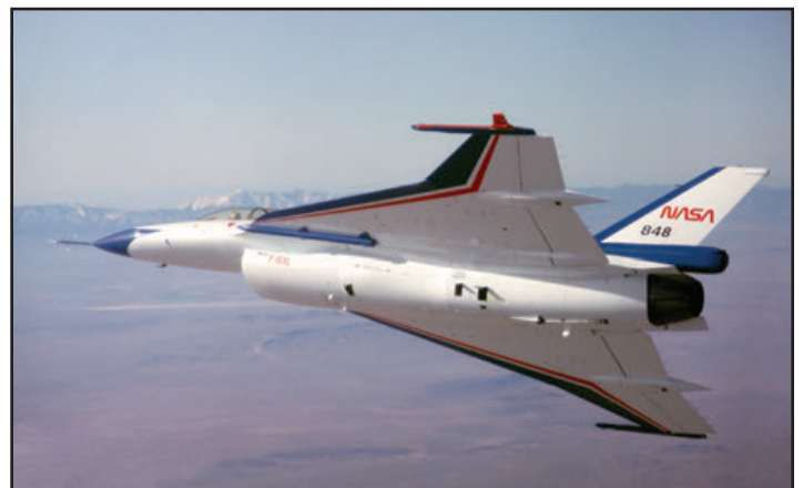
With a bright red, Dynamic Engineering Inc. (DEI) flutter exciter mounted on the left Sidewinder missile rail, NASA 848 performs another test mission from Edwards AFB on 27 February 1992. (NASA)
