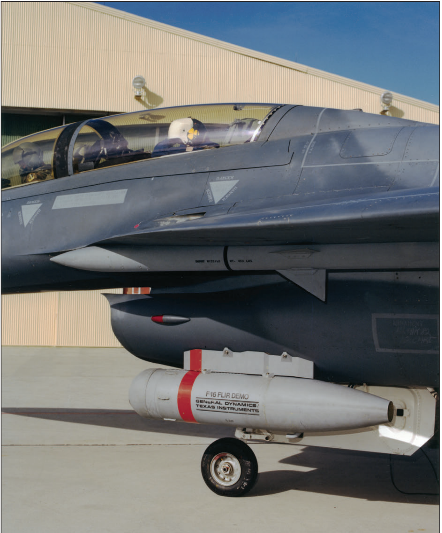
Lt. Col. Marty Bushnell and General Dynamics pilot, Kevin Dwyer, performed 3 test flights on F-16XL, 75-0747, between 14 and 16 December 1983 with an F-16 Forward Looking Infrared (FLIR) demonstration pod attached to the left side of the inlet. Only XL-2 was equipped with load stations on each side of the inlet and this was the only time an F-16XL carried a store in this location. (Sheryl Tierney collection)
