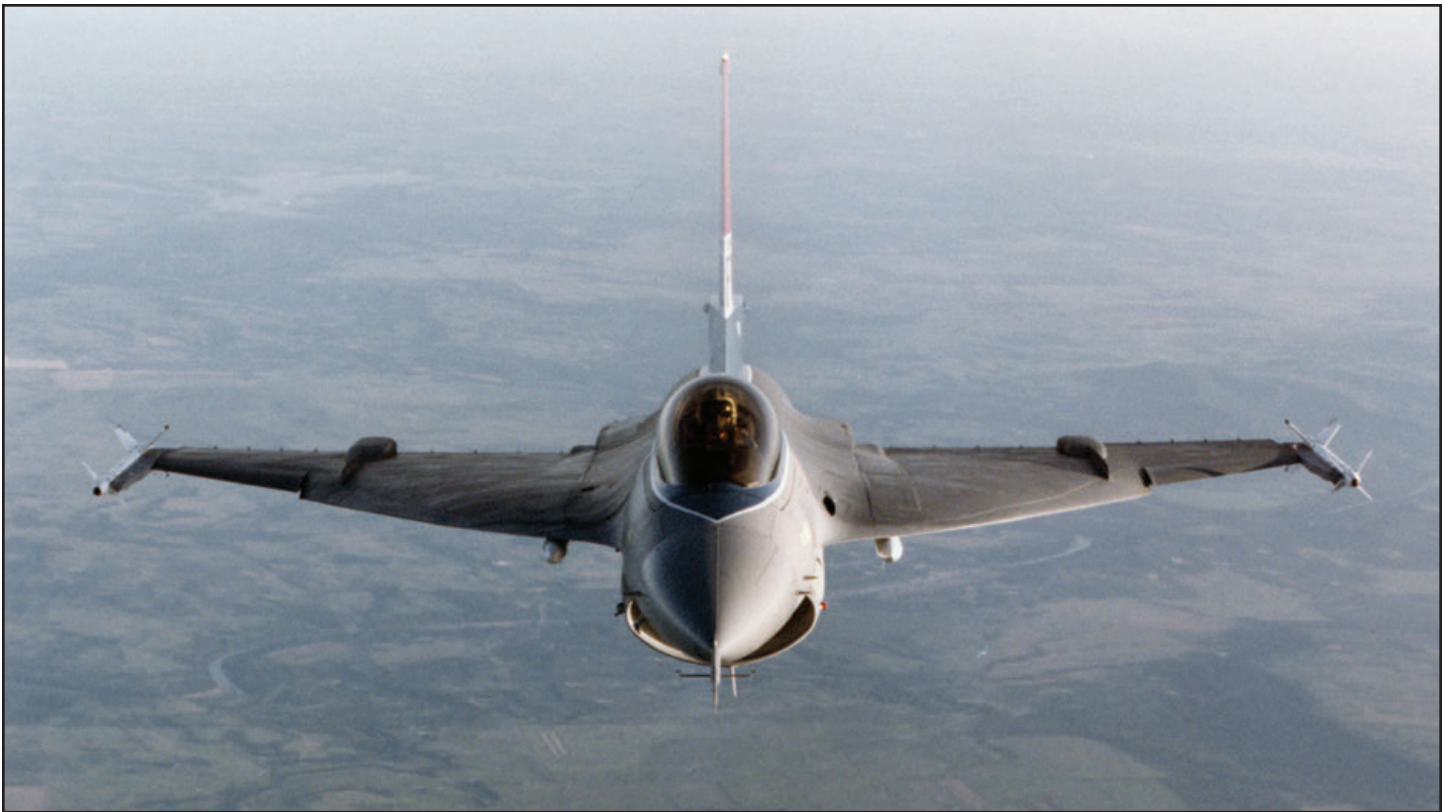
The clean lines of the cranked-arrow wing design applied to the F-16 show up well in this front view of the F-16XL during flight number 3 on 17 July 1982. (Lockheed Martin via Sheryl Tierney)
