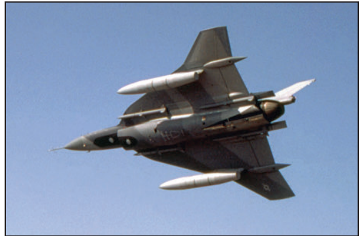
F-16XL, 75-0747, with wingtip fairings in place of the Sidewinder missile rails. (Keith Svendsen)
