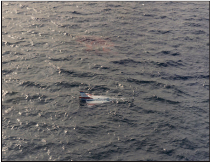
Testing the spin characteristics of the General Dynamics F-16XL design required the use of large scale models released from a NASA UH-1 helicopter over the Atlantic ocean and recovered via parachute at the end of each test mission. Note the model above carries an F-16F designation. (NASA Langley)
