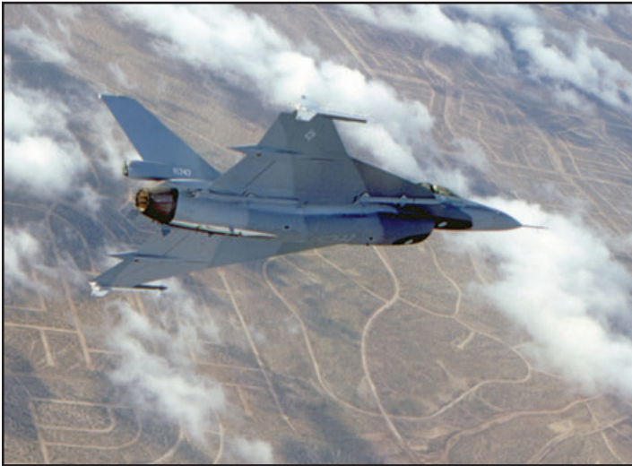
Originally a single-seat F-16A, XL-2 received a two-seat modification during conversion to an F-16XL air-frame. Visible in the inset is the updated data block used on the aircraft during the F-16XL test program. Note it shows the aircraft type as an F-16B and the serial number is now 75-0747A. (Keith Svendsen- all 4 above)
