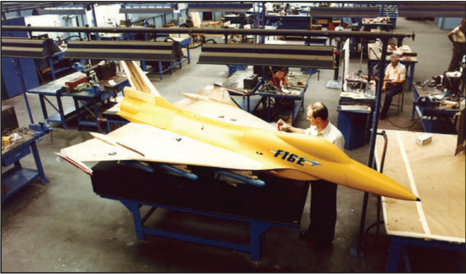
Testing the spin characteristics of the General Dynamics F-16XL design required the use of large scale models released from a NASA UH-1 helicopter over the Atlantic ocean and recovered via parachute at the end of each test mission. Note the model above carries an F-16F designation. (NASA Langley)
