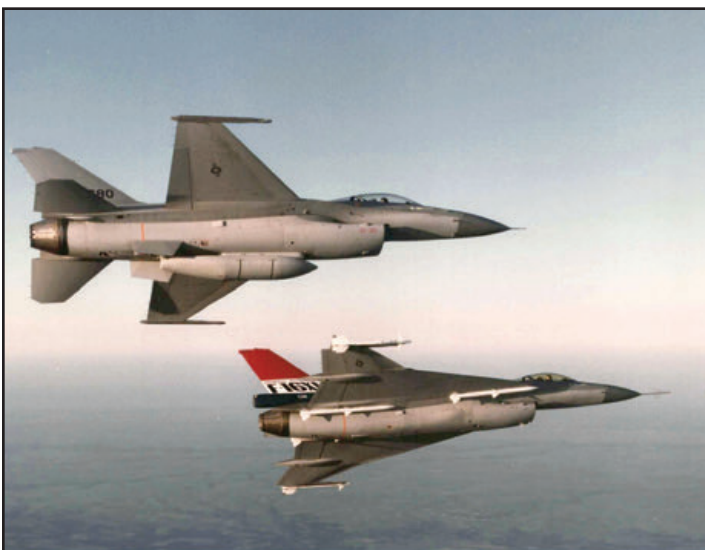
A series of images taken during the third flight of the F-16XL on 17 July 1982. Clearly visible is the lack of ventral stabilizing fins on the lower aft fuselage of the F-16XL. With the extended fuselage and new wing design, the ventral fins were no longer required for lateral stability. (Lockheed Martin)
