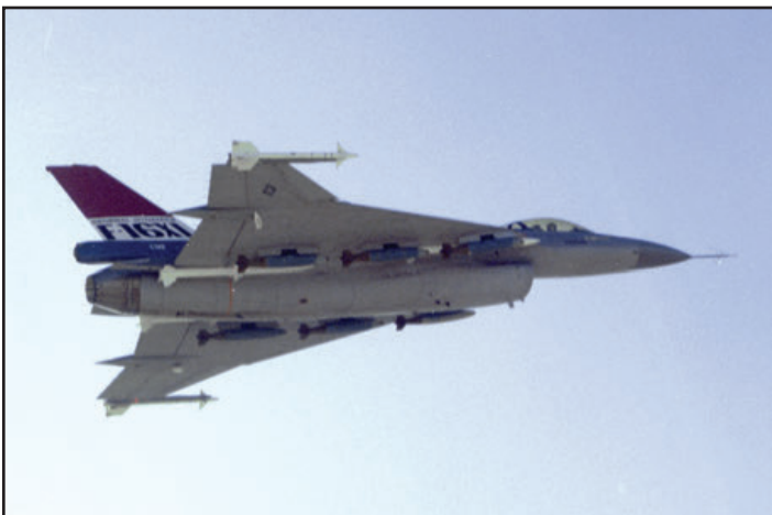
Beginning 13 October 1982, F-16XL, 75-0749, began a series of 11 stability & control, and weapon separation tests with 6 Mk82 bombs. The small white objects mounted on the trailing edge fairings are camera pods used for filming the bomb release. (AFTC History Office)
