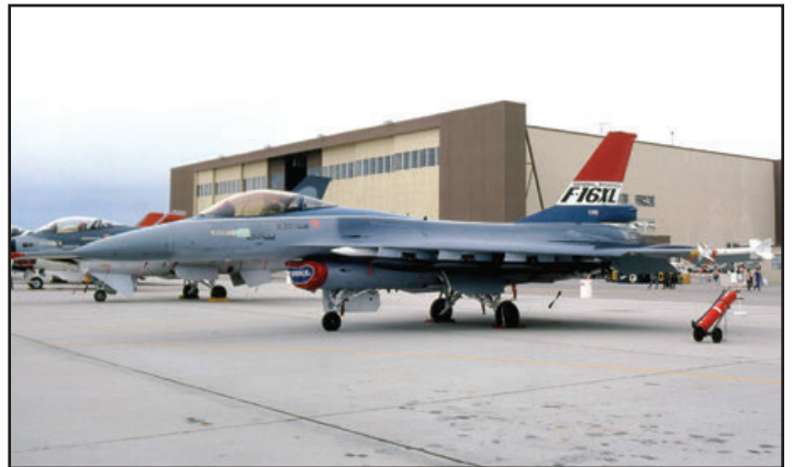
Close-up details of F-16XL, 75-0749 taken during the annual open house at Edwards AFB show aspects of the forward fuselage, Mk82 bomb & pylon, and trailing edge control surfaces. (Keith Svendsen)
