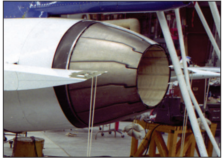
There was no discernible external difference in the engine exhaust nozzle of the GE F110 'Slimline' and F110-GE-129 engines. (Keith Svendsen- top left; NASA- top right)
