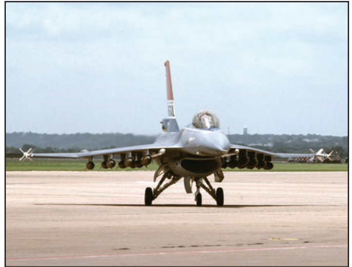
Carrying a full load of 16-Mk82 bombs, F-16XL, 75-0749, taxi's around the ramp at General Dynamics Ft. Worth facility. No records were located showing the aircraft ever flew in this configuration. (Lockheed Martin)
