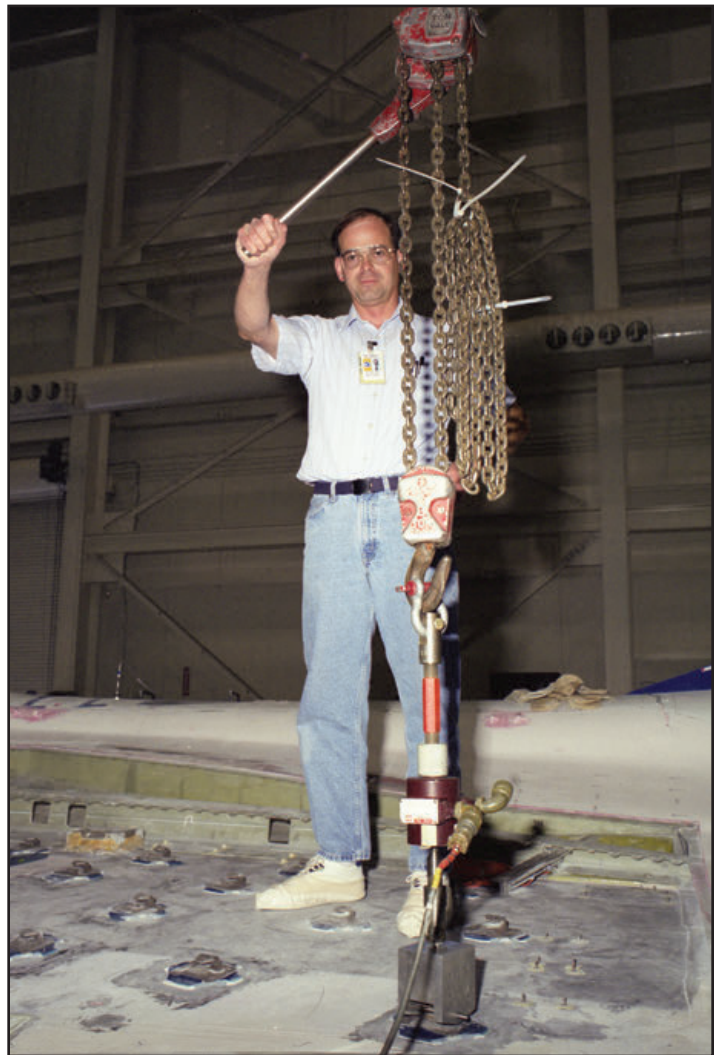
Prior to flight testing, each of the attachment fittings (top left) required load test verification. The suction glove was removed (left) and each fitting was cleaned of excess adhesive (middle left). NASA instrumentation technician, Bill Lokos, uses a calibrated pull assembly to test each pad on 14 April 1995 (above). (NASA)
