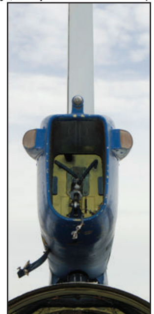
The dorsal fairing of the vertical stabilizer contained a Norwegian-type drag chute system with an increased area of 19-foot diameter, gold-color canopy. (Lockheed Martin- above left; Tony Landis- 2 above)
