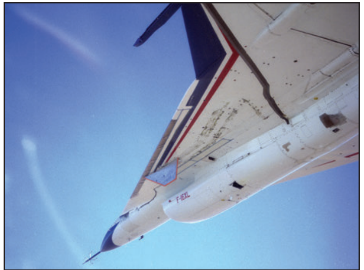
The first supersonic test flight took place on 22 November 1995 with Dana Purifoy at the controls. One of the many instruments added to NASA 848 was a charging patch particle detector placed on the leading edge of the vertical stabilizer. (NASA- all)
