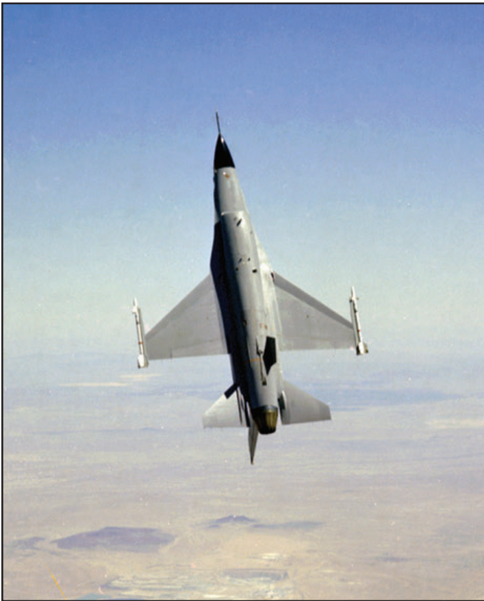
With F-16A, 75-0747, flying safety chase, YF-16A, 75-0745, is outfitted with two laser guided bombs during a sortie on 26 September 1977. (AFTC History Office)
