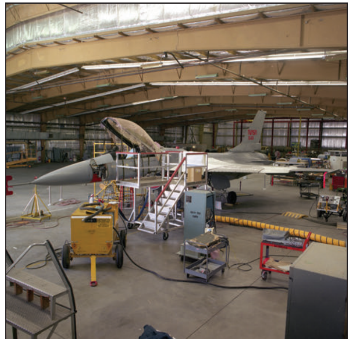
With the laminar flow wing glove installed, NASA 849 undergoes ground instrumentation checks inside hangar 4826 at NASA Dryden Flight Research Center in April 1990. (NASA- 2 above)
