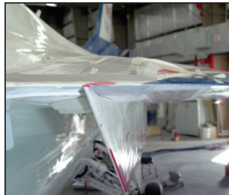
During May and June 1993, NASA technicians added more instrumentation, a modified leading edge, gun bay cover and shock fences under each wing to F-16XL NASA 848. (NASA- 6 above)
