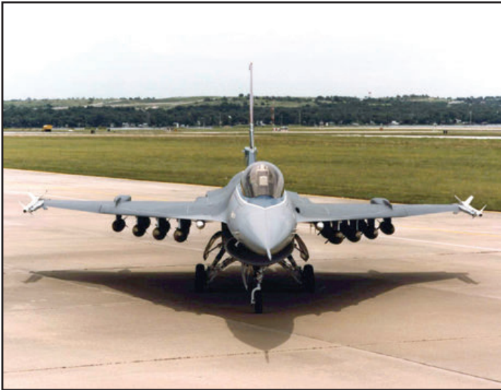
Carrying a full load of 16-Mk82 bombs, F-16XL, 75-0749, taxi's around the ramp at General Dynamics Ft. Worth facility. No records were located showing the aircraft ever flew in this configuration. (Lockheed Martin)
