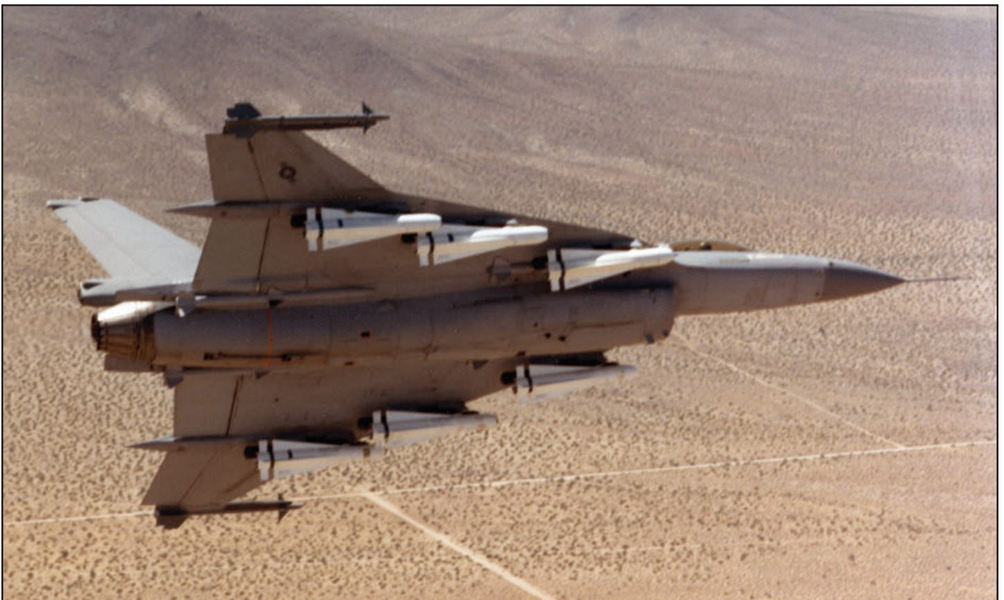
F-16XL, 75-0749, carried a weapon configuration of 6-AGM-65 Maverick missiles on multiple occasions during the test program to perform stability & control as well as flutter testing. An actual AGM-65 missile firing took place only a single time. (Sheryl Tierney collection)
