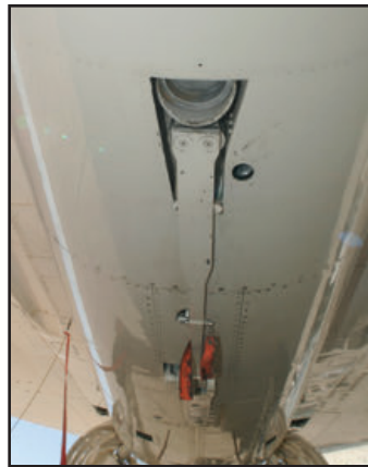
The 2 ventral fins carried by standard F-16's were not required on the F-16XL due to the lengthened fuselage. Standard F-16 tail hook arresting assembly is located in aft fuselage. (Keith Svendsen- above, left; Tony Landis- 2 above)
