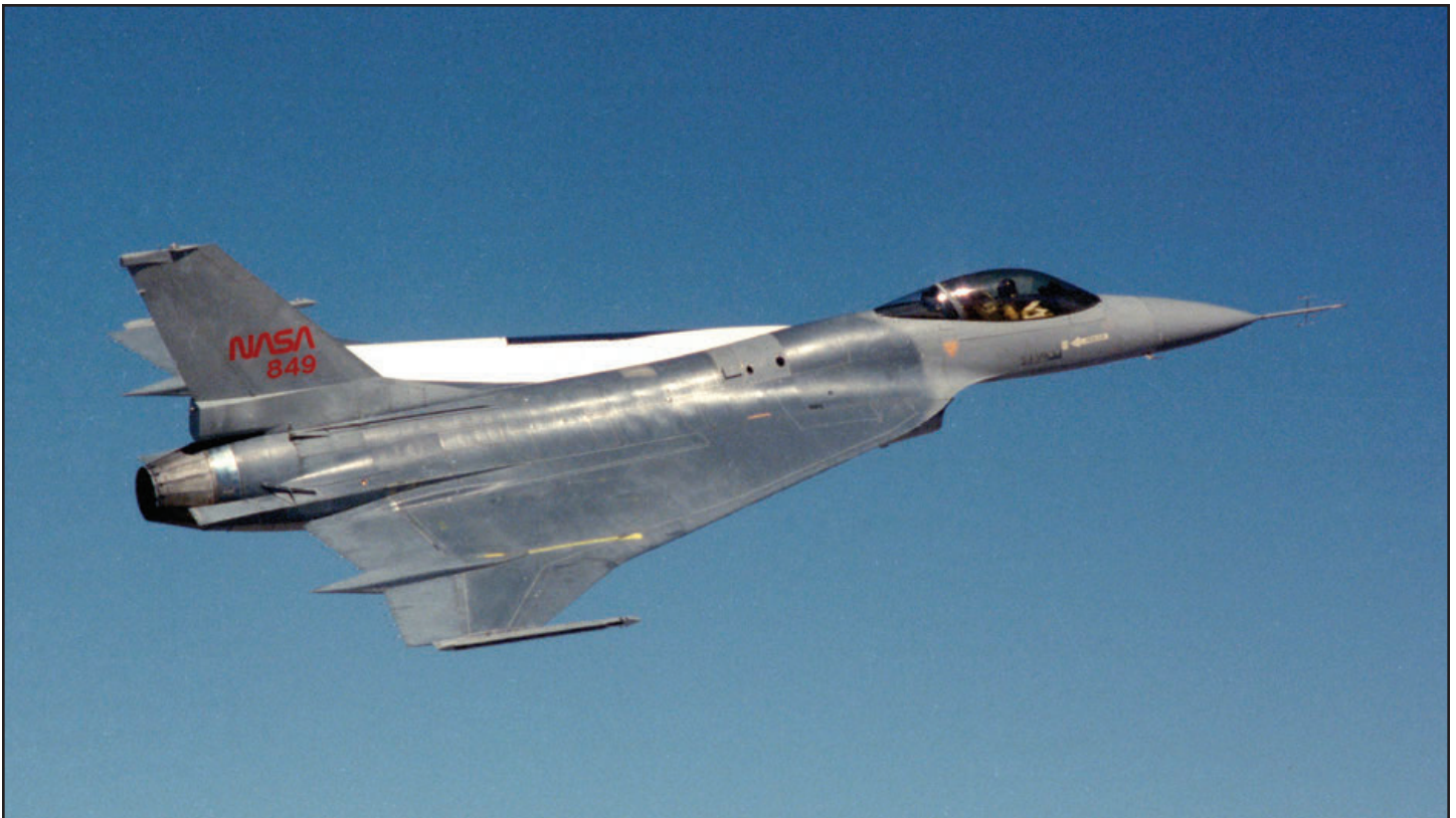
F-16XL NASA 849 during its first FCF on 3 May 1990, after the supersonic laminar flow control (SLFC) wing glove modification. Note the aircraft retains the spin chute mounting assemblies. (NASA)
