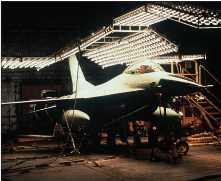
The Air Force made use of F-16A 75-0749 for early climatic testing, putting the FSD airframe through extreme heating and cold tests inside the McKinley Climatic Laboratory at Eglin AFB, FL. (USAF)
