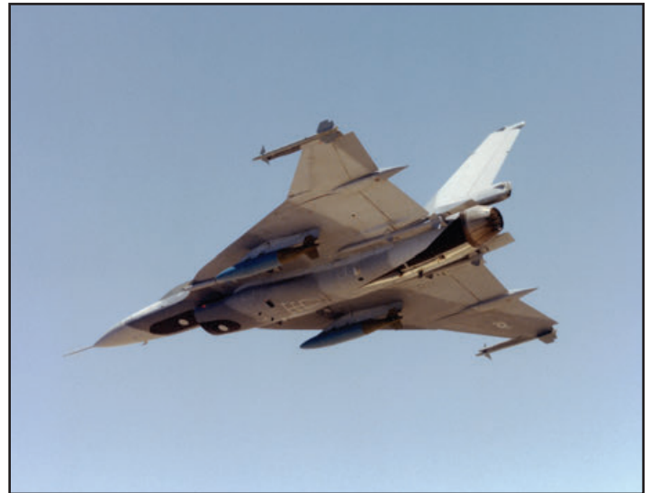
One of many different weapon load configurations tested on the two F-16XL aircraft during the test program, F-16XL, 75-0747, is carrying 4-Mk84 bombs during a mission on 13 July 1983. Crew members are Lt. Col. Ed Thomas and Capt. Keith Svendsen. (Lockheed Martin- both above)
