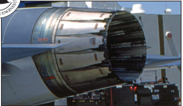
Powering F-16XL, 75-0749, throughout the entire test program was a Pratt & Whitney, F100-PW-200 afterburning turbofan engine capable of providing approximately 24,000 lbs maximum thrust, similar to those used in the basic F-16. (Pratt & Whitney- Top 2; USAF- above left; Keith Svendsen- above right)
