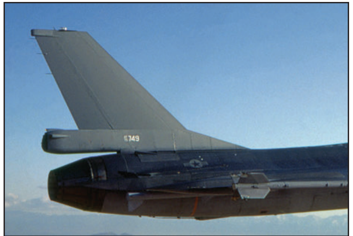
The gray walkway striping and other stenciling applied over the FS36118 dark gray and blue were FS36231 gray. When the demonstrator markings were painted over in March 1983, the vertical stabilizer received a coat of FS36270 gray. (Lockheed Martin- top, left; Keith Svendsen- top, right)
