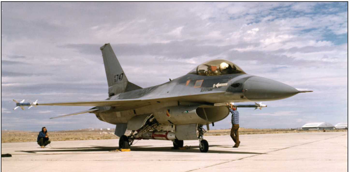
Ground crewman at Edwards AFB, CA, perform final checks on 75-0747 carrying a B-61 'Sandia' bomb on the centerline station at the 'last chance' area next to the runway. With the gray radome and standardized serial number on the tail, 747 is looking closer to the operational fleet. (National Archives)
