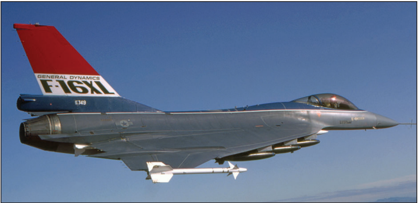
F-16XL, 75-0749, is shown with a during a performance test mission, loaded with 12-Mk82 bombs on 10 December 1982 with General Dynamics pilot 'Joe Bill' Dryden in the cockpit. (Keith Svendsen)
