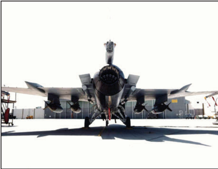
One of many different weapon load configurations tested on the two F-16XL aircraft during the test program, F-16XL, 75-0747, is carrying 4-Mk84 bombs during a mission on 13 July 1983. Crew members are Lt. Col. Ed Thomas and Capt. Keith Svendsen. (Lockheed Martin- both above)
