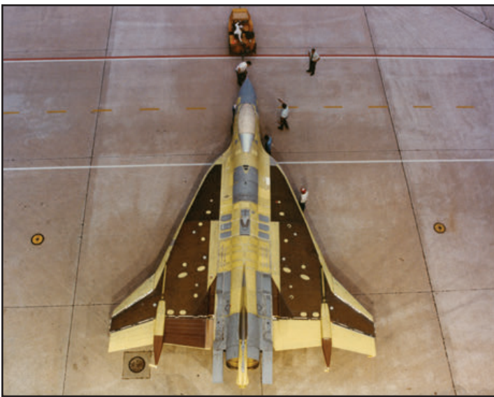
With loads testing successfully completed, the F-16XL, went through final assembly of the air-frame having the control surfaces, landing gear, nose radome and other internal components installed. The aircraft is shown here heading to the paint shop during May 1982. (Lockheed Martin)
