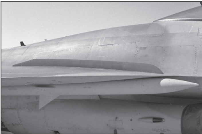
Inboard fences were added to F-16XL, 75-0749, for single flight on 7 July 1983 in an attempt to address a minor pitch gallop anomaly. (Keith Svendsen) Lt. Col. Marty Bushnell and Alex Wolfe bring F-16XL, 75-0747, back from high-speed envelope expansion mission on 26 May 1983. (Michael Grove, Sr.)
