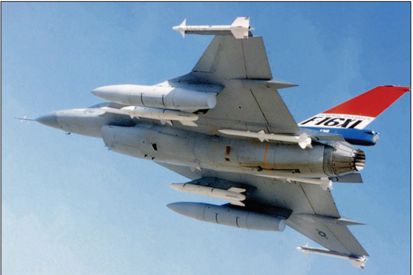
F-16XL, 75-0749, performed two stability & control, and flutter test flights on 7 December 1982 loaded with 2-370 gallon wing tanks and 2-BDU-38 (simulated B61 nuclear bomb) practice bombs. (Sheryl Tierney Collection)
