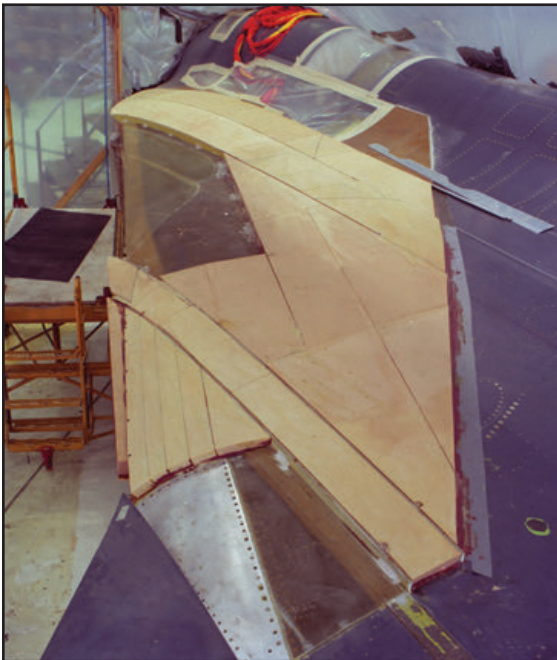
As seen in these images taken on 21 July 1989, NASA technicians immediately went to work installing the small laminar flow wing glove on the left wing of XL-1, soon to be bearing serial number NASA 849. (Lockheed Martin)
