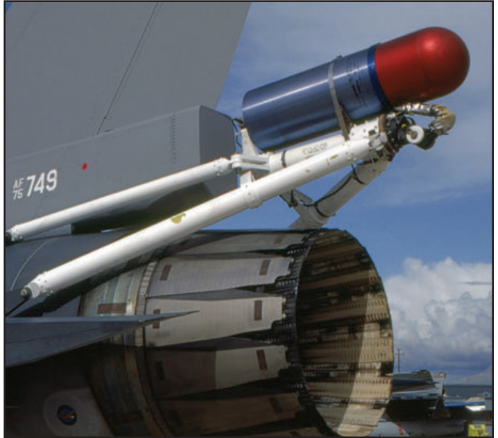
Close-up detail of the spin chute modification on F-16XL, 75-0749 on 3 March 1983. Note that the drag chute box has been blocked off and the tail of the aircraft is now overall gray with white serial number. (Keith Svendsen)
