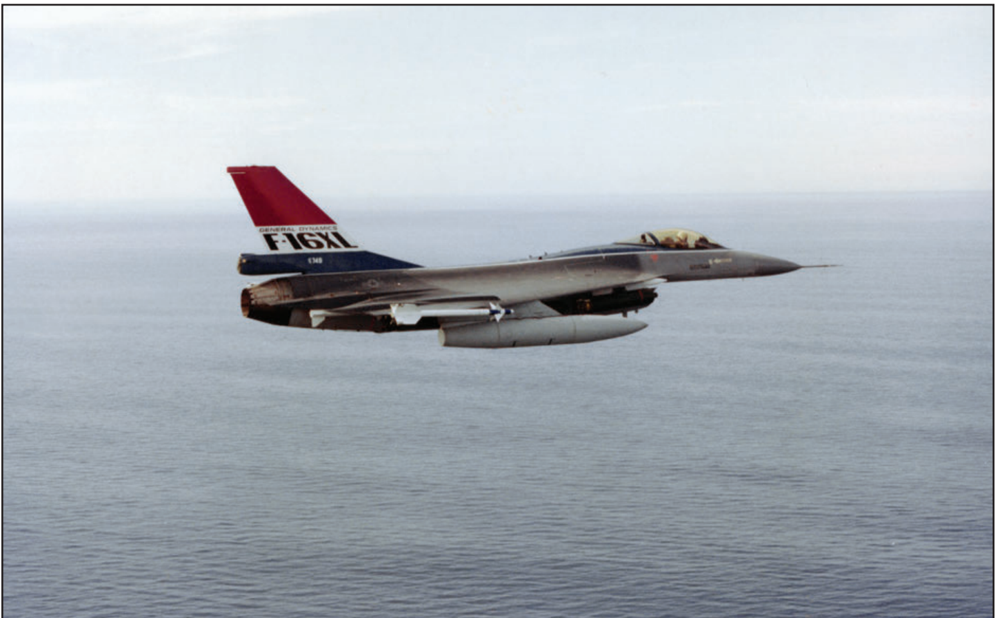
F-16XL Combined Test Force (CTF) deputy director, Lt. Col. Edwin Thomas, takes XL-1 over the Pacific Ocean during a performance check flight, carrying 6-SUU-65 cluster bombs and 370 gallon wing tanks. (Sheryl Tierney collection)
