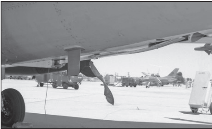
The 2 ventral fins carried by standard F-16's were not required on the F-16XL due to the lengthened fuselage. Standard F-16 tail hook arresting assembly is located in aft fuselage. (Keith Svendsen- above, left; Tony Landis- 2 above)
