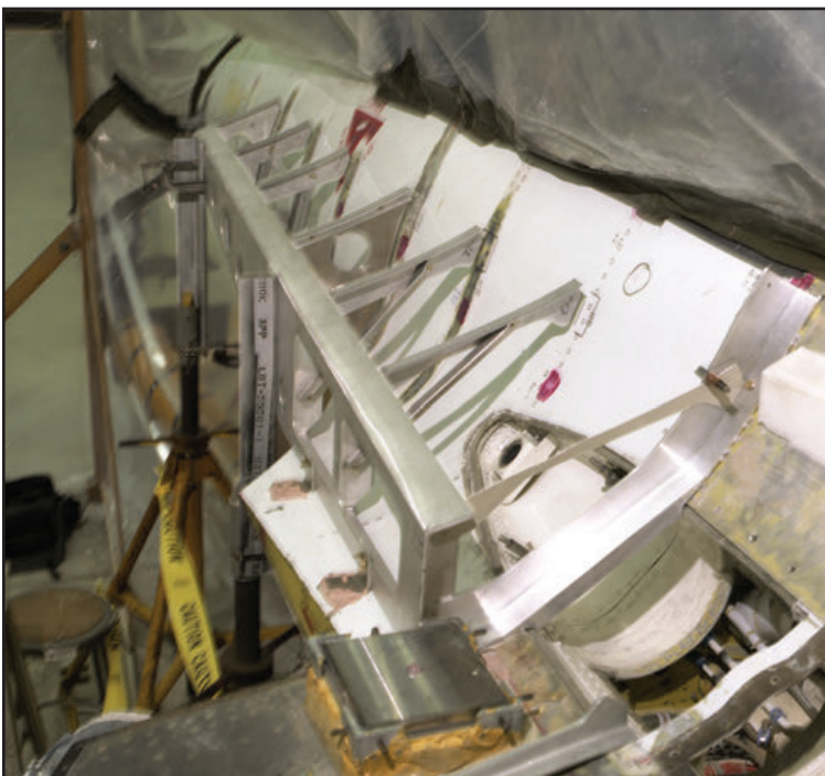
Modifications to NASA 848 began in July 1993 and continued over the next two years. The forward structure for the new wing is shown above. (NASA- all)
