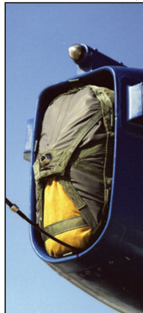
The dorsal fairing of the vertical stabilizer contained a Norwegian-type drag chute system with an increased area of 19-foot diameter, gold-color canopy. (Lockheed Martin- above left; Tony Landis- 2 above)
