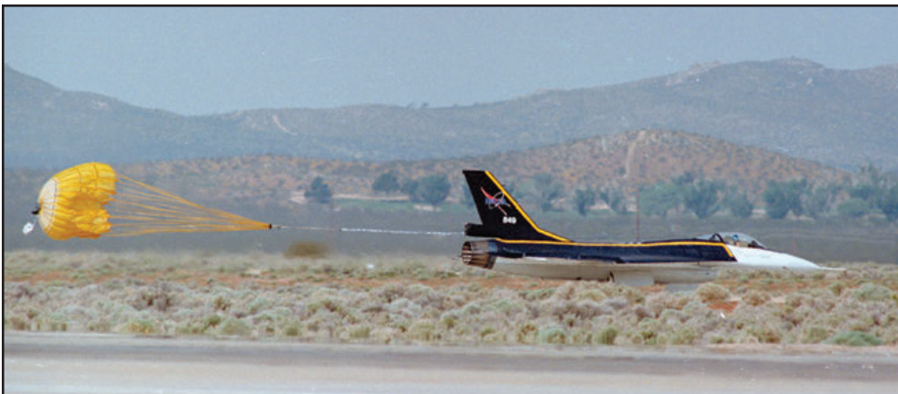
F-16XL, NASA 849, performed numerous test missions during April and May 1995. The pilot often kept the landing parachute attached until they taxied off the runway to prevent the ground crews from having to retrieve it. (Tony Landis)
