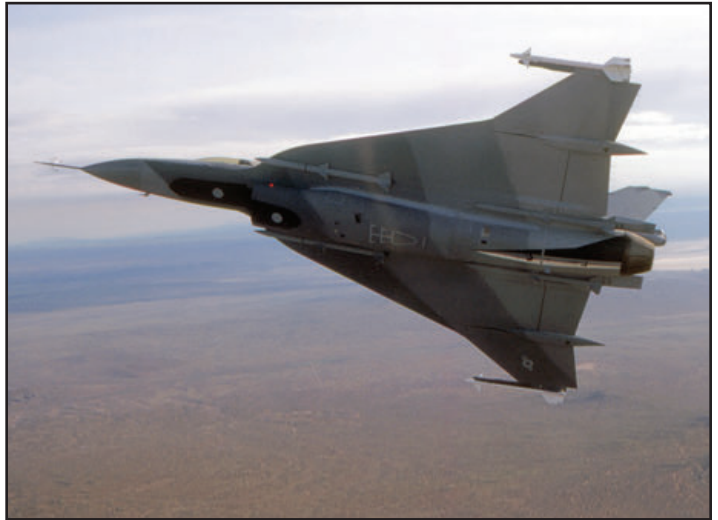
Originally a single-seat F-16A, XL-2 received a two-seat modification during conversion to an F-16XL air-frame. Visible in the inset is the updated data block used on the aircraft during the F-16XL test program. Note it shows the aircraft type as an F-16B and the serial number is now 75-0747A. (Keith Svendsen- all 4 above)
