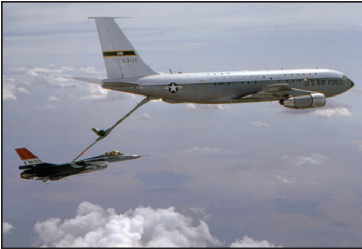
The F-16XL takes on fuel from NKC-135E, 55-3135 on 23 August 1982. The tanker was fitted with 50 small windows for nuclear readiness testing. (Keith Svendsen)
