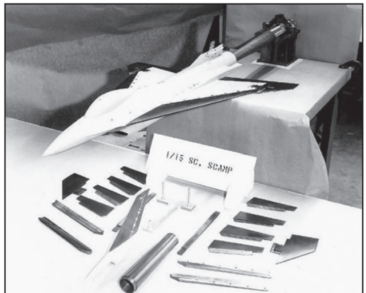
The 1/15th scale SCAMP wind tunnel model with various components changed out during wind tunnel testing. (Robert Wetherall collection)
