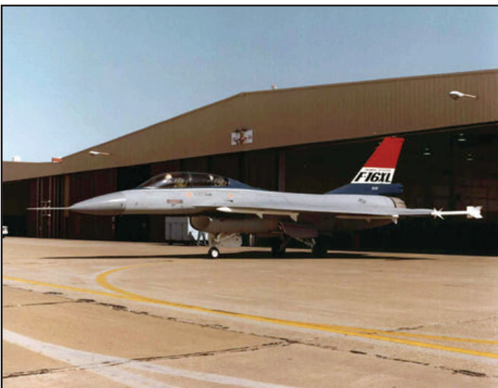
Taxi testing for the second F-16XL in October 1982, slowly building up to the final high-speed taxi on 30 October. At the end of the high-speed taxi, the braking parachute deployment was tested. (Lockheed Martin)
