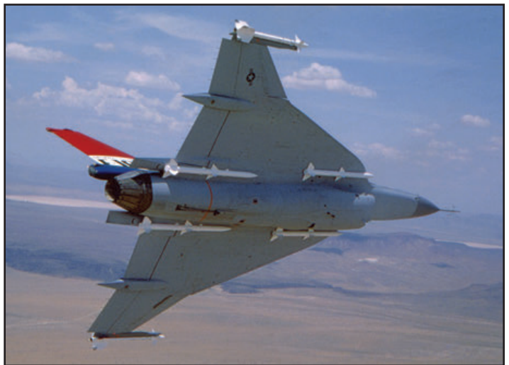
The primary air-to-air mission load consisted of an AIM-9 Sidewinder on each wingtip and 4 dummy AIM-120 AMRAAM missiles. (Keith Svendsen)
