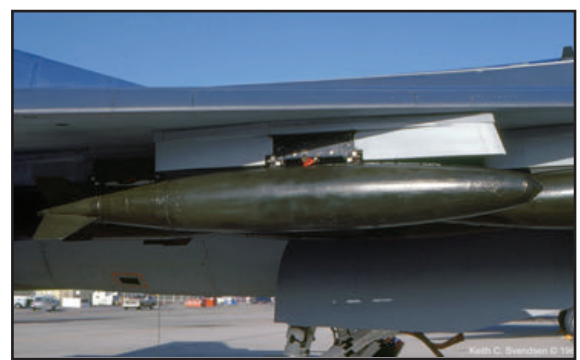
A typical air-to-ground mission load consisted of 12-Mk82, 500 pound, free-fall, gravity bombs attached to Lode 14 wing pylons. (Lockheed Martin- above; Keith Svendsen- right)
