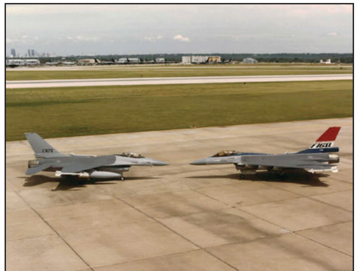
F-16XL 75-0749 is parked next to F-16A 81-0672 on the ramp in Ft. Worth. Both aircraft are configured for a typical air-to-ground mission. The F-16A required two external wing tanks and carried only 6-Mk82's, while the F-16XL could perform the same mission with twice the payload and no external tanks. (Lockheed Martin)
