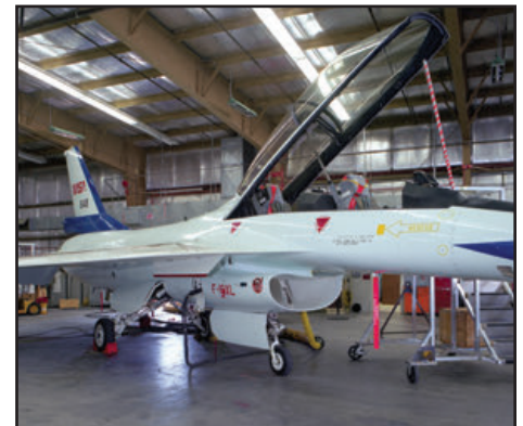
During May and June 1993, NASA technicians added more instrumentation, a modified leading edge, gun bay cover and shock fences under each wing to F-16XL NASA 848. (NASA- 6 above)
