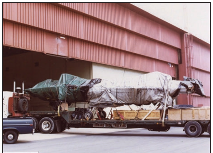
Performing during the annual open house at Edwards AFB on October 31, 1980, F-16A, 75-0747, suffered a blown nose tire on takeoff. The pilot chose to make an emergency landing on the dry lakebed and the aircraft was substantially damaged when the nose gear collapsed. The airframe was returned to General Dynamics via C-5 Galaxy and rebuilt as the two-seat F-16XL. (Lockheed Martin)
