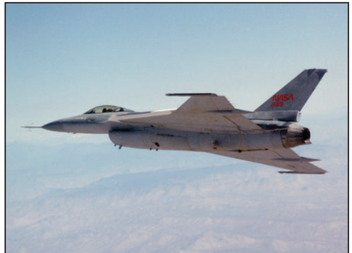
NASA test pilot Steven Ishmael takes F-16XL, NASA 849 up on its first Functional Check Flight (FCF) on 3 May 1990. While adding the laminar flow glove, the small strakes on the wing upper surface were removed. The medium gray panel in front of the in-flight refueling receptacle covers the suction pump assembly for the wing glove. (NASA- all)
