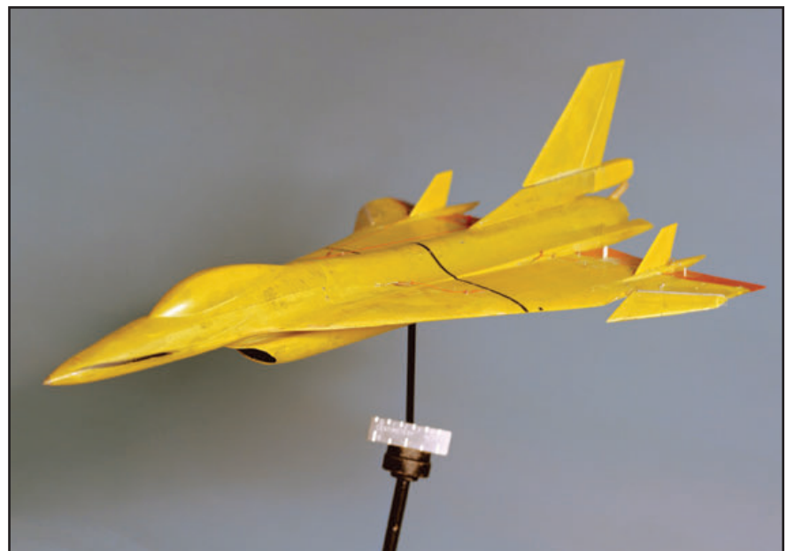
This model in the NASA Langley Research Center wind tunnel shows the change to the F-16 vertical stabilizer, minus the parachute housing. (NASA Langley)
