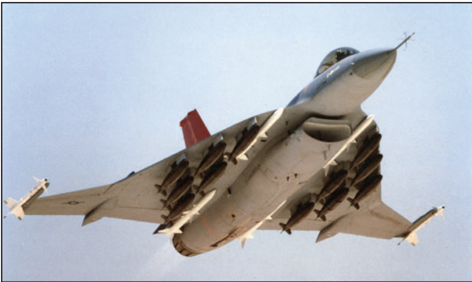
The first, and only, time F-16XL, 75-0749, released a load of 12 Mk82 bombs occurred during a flight on 24 August 1982 with GD pilot Alex Wolfe at the controls. All bombs separated clean and grouping remained tight until impact. (Craig Kaston collection, left; Lockheed Martin, all images below)
