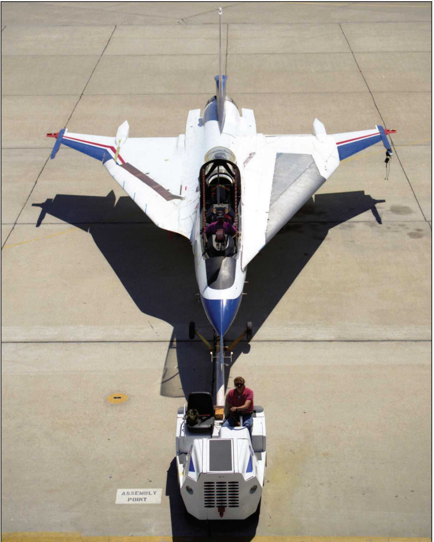
NASA aircraft maintenance chief, Tom Grindle, drives the tug pulling F-16XL, NASA 848, into position for the photographer. The significant change of shape to the left wing is readily noticeable in this view. (NASA)
