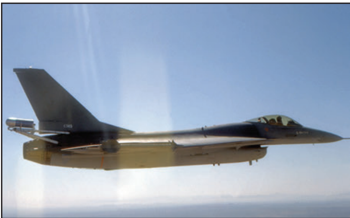
Sporting a fresh coat of paint, F-16XL 75-0749 is equipped with the spin chute assembly for additional high AoA testing on 7 August 1984, piloted by Lt. Col. Edwin Thomas. (Keith Svendsen- both above)
