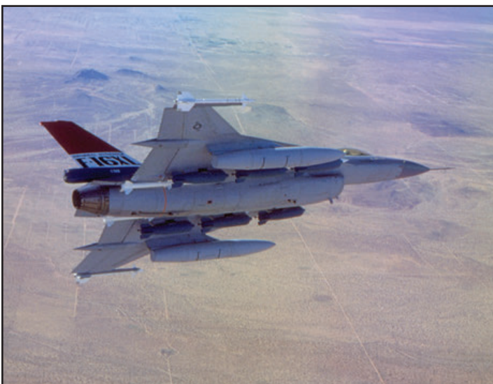
Taken during test missions on 13 December and 17 December 1982, the photos above, and the following page, show F-16XL, 75-0749, carrying a load of 6-CBU-58 cluster bombs and 2-370 gallon wing tanks in addition to the dummy AMRAAM's and Sidewinders. (Michael Grove, Sr.-2 at top; Keith Svendsen-3 above and 4 on following page)
