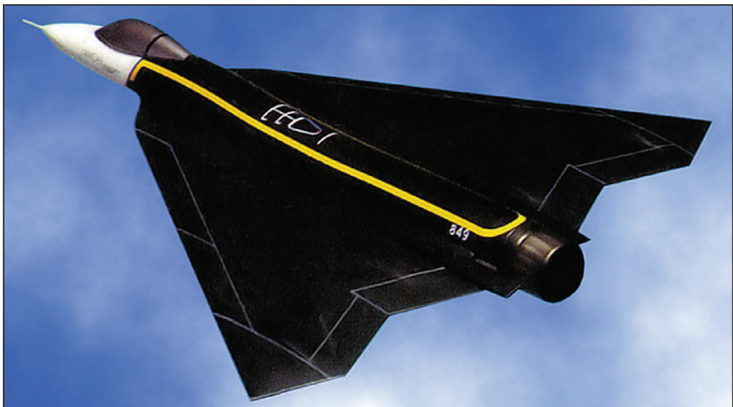
Lockheed Martin proposed tailless variations of the F-16XL under its Innovative Control Effectors (ICE) program as early as 1995. Many derivatives of this design were tested in the wind tunnel. (Lockheed Martin)
