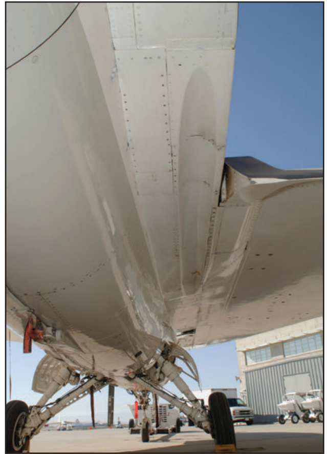
Wing hardpoints were built into the underside of the wing for the carriage of additional weapons or fuel tanks, while the fuselage is modified to allow for semi-submerged AMRAAM missiles. (Tony Landis)
