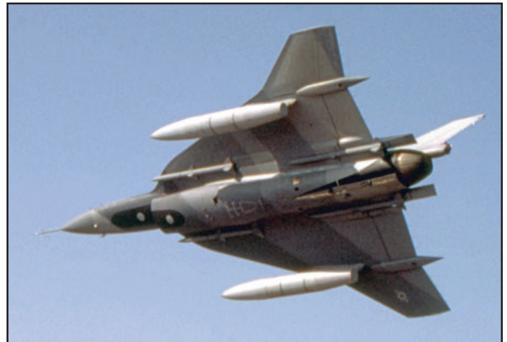
Both F-16XL aircraft performed test missions with wingtip fairings replacing the Sidewinder missile launch rails. (Lockheed Martin- both)
