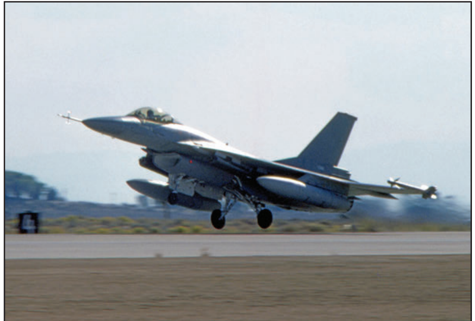
F-16XL, 75-0749, departs and returns to Edwards AFB during 1 of 3 brief, performance test flights on 28 October 1983 with 2-370 gallon wing tanks, and 6-SUU-65 weapon stores. (Keith Svendsen- both above)
