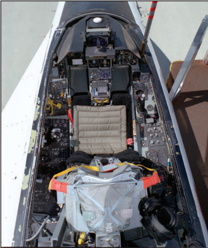
The series of images on this page and the following page show the front and aft cockpits of XL-2 in July 1996, near the end of the NASA test program. Note the addition of the white GPS antenna in front of the HUD, and controls for the Supersonic Laminar Flow experiment in the aft cockpit. (Tony Landis)
