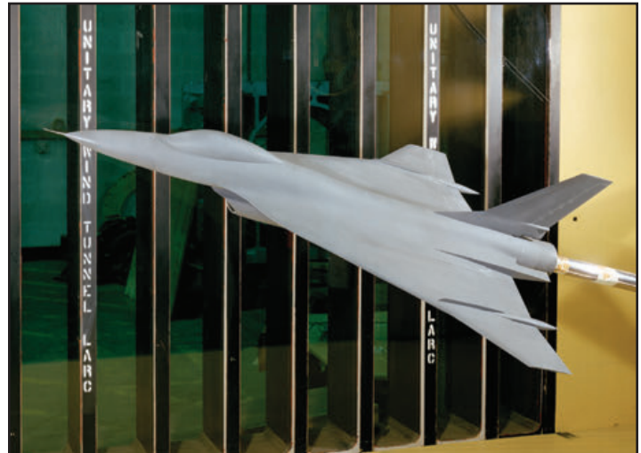
This model in the NASA Langley Research Center wind tunnel shows the change to the F-16 vertical stabilizer, minus the parachute housing. (NASA Langley)
