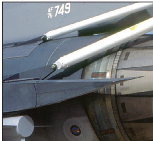
The gray walkway striping and other stenciling applied over the FS36118 dark gray and blue were FS36231 gray. When the demonstrator markings were painted over in March 1983, the vertical stabilizer received a coat of FS36270 gray. (Lockheed Martin- top, left; Keith Svendsen- top, right)
