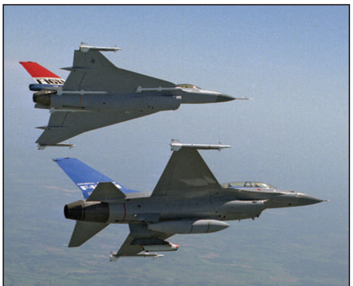
The F-16/79 was General Dynamics export variant of the F-16. With a different avionics package and powered by a General Electric J79 engine, it is shown in formation with the first F-16XL over the Texas landscape. (Lockheed Martin)
