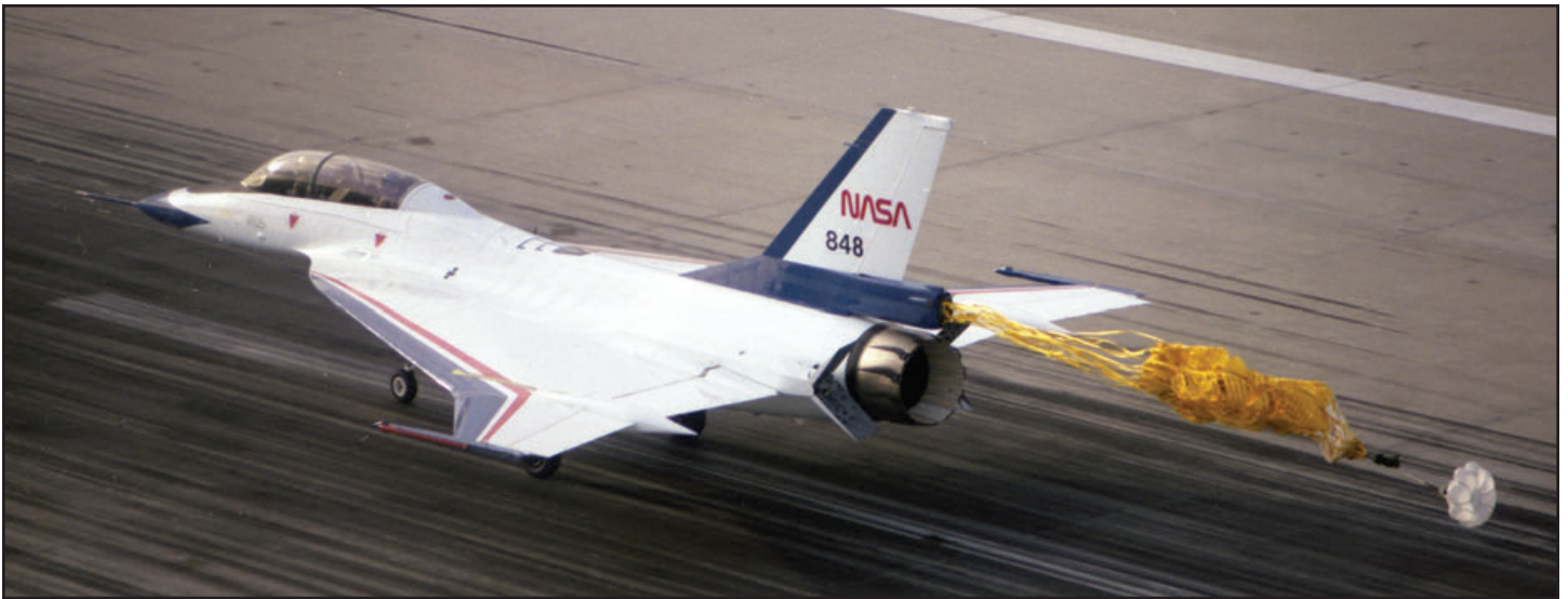
With its gold parachute streaming and speedbrakes deployed, F-16XL NASA 848 comes in to land on Edwards AFB runway 22 at the end of a test mission on 21 January 1993. (NASA)
