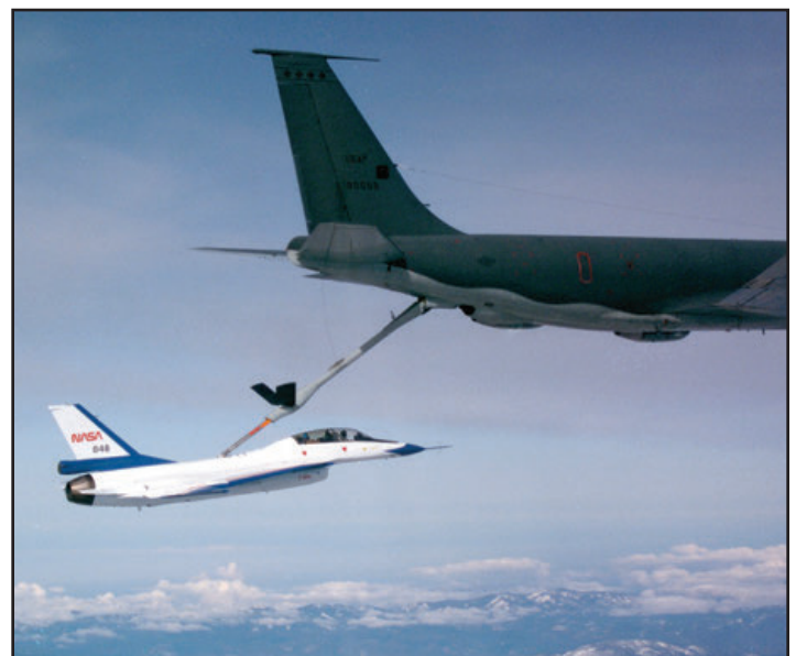
F-16XL NASA 848 during a test mission on 9 March 1992. Note the forward canopy section is clear while the aft canopy section is gold-tinted. A common practice on early two-seat F-16's. (NASA)
