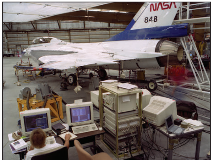
Ground vibration testing was also completed on NASA 848 in September 1997. (NASA)
