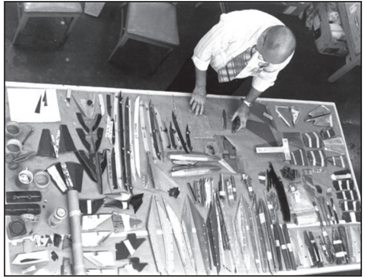
A table is set up next to the wind tunnel model where the test crew could lay out various components available for configuration changes. (Robert Bradley collection)
