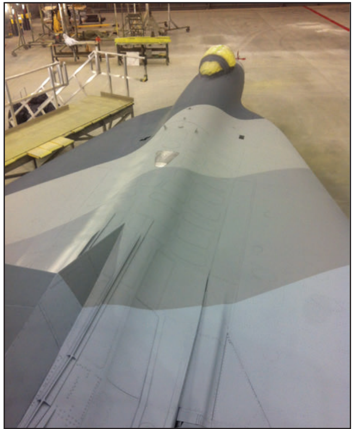
XL-1 received a fresh coat of paint in February/March 2019. After sanding and prep work, the aircraft received a green primer undercoat (top left). The museum chose a fictional gray paint scheme based on the 'splinter camouflage' scheme flown on XL-2 and added an 'ED' tailcode not carried by either F-16XL. (USAF)
