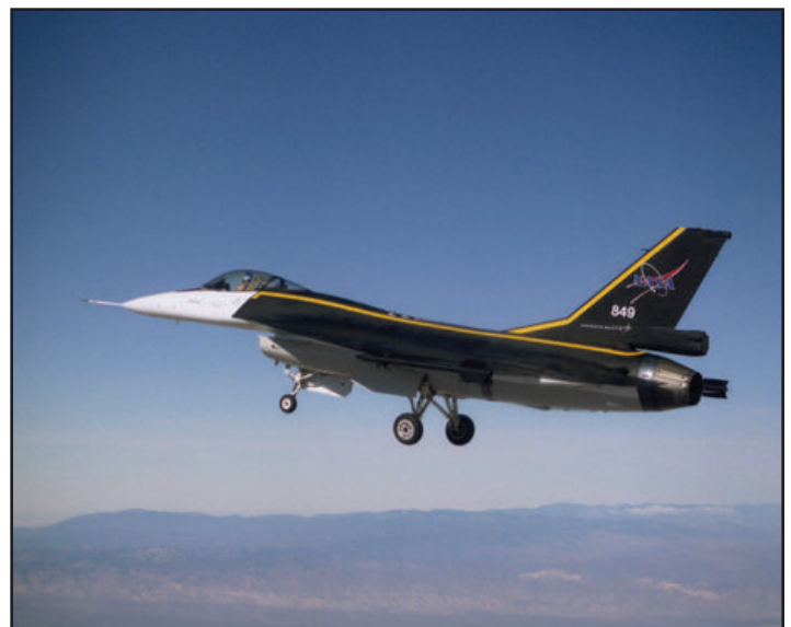
In 1997, NASA 849 received a digital fly-by-wire flight control system, replacing the original analog system. This gave the aircraft better flexibility as a flight testing platform. The F-16XL performed its first flight with the new system on 16 December 1997. The Lockheed Martin logo was added to the base of the vertical stabilizer during this time. (NASA)
