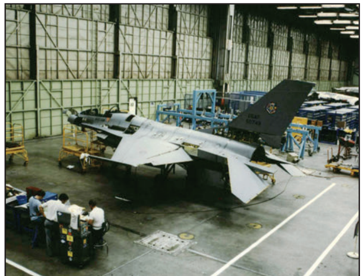
F-16A, 75-0749, prior to being placed in the demating jig. In addition to the new wing, two fuselage extensions were added to the fuselage structure. (Lockheed Martin)
