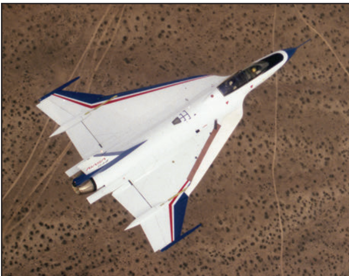
The modified right wing and missing wing strakes are visible in this view of NASA 848 on 3 February 1993. (NASA)
