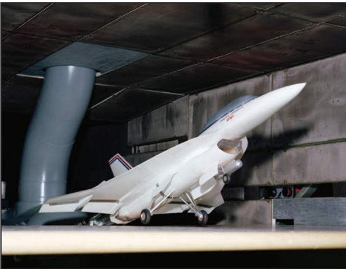
NASA's Lewis Research Center (now Glenn Research Center) in Cleveland, OH, was responsible for propulsion and engine inlet design testing. NASA Lewis made use of the 9 x 15 foot Low-Speed Wind Tunnel. (NASA Glenn)
