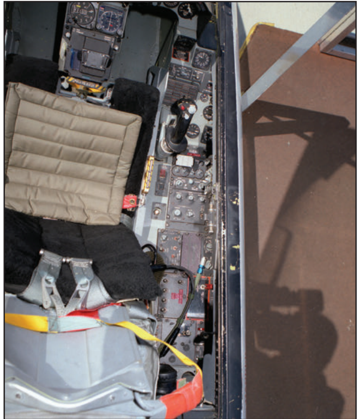
The series of images on this page and the following page show the front and aft cockpits of XL-2 in July 1996, near the end of the NASA test program. Note the addition of the white GPS antenna in front of the HUD, and controls for the Supersonic Laminar Flow experiment in the aft cockpit. (Tony Landis)
