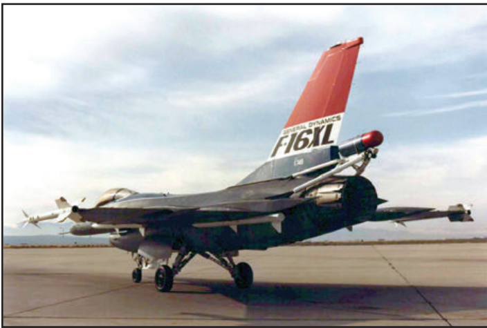
Prior to high Angle-of-Attack (AoA) testing, F-16XL, 74-0749 received a spin chute modification, which required the removal of the braking parachute housing. This mod took place at Edwards AFB during a 10-day period in January 1983. The spin chute was tested during a high speed taxi test on 22 January 1983 (top, left). The spin chute cockpit control panel in the F-16XL (above, right). (Keith Svendsen- top, right; Sheryl Tierney collection- top, right & above, right; Lockheed Martin- above, left)
