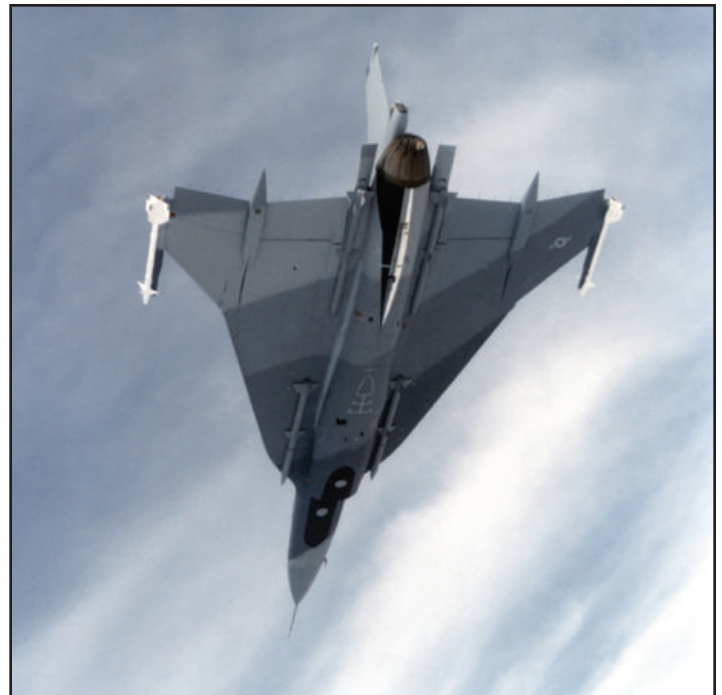
Officially known as Deceptive Camouflage, or Splinter Camouflage, this particular variation, which included a false canopy and upper surface markings applied to the bottom of the aircraft, was the brainchild of aviation artist Keith Ferris. Ferris designed many variations of the Splinter scheme that were tested on various aircraft during the 1970's and 1980's. (Lockheed Martin)
