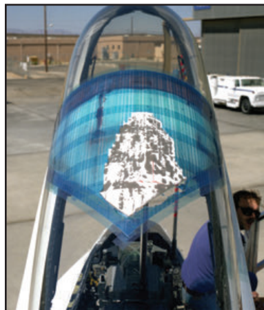
Prior to a research mission on 12 September 1996, NASA engineers attempted to modify the airflow over the canopy by adding thin foam covered in blue tape (above and far left). A portion of this section failed during the flight (left). Airflow tufts were also added near the back of the canopy. NASA technician, Bob Cummings, runs checks from the aft seat of the F-16XL (above). Note the different shock fence in the photo above left. (NASA- all)
