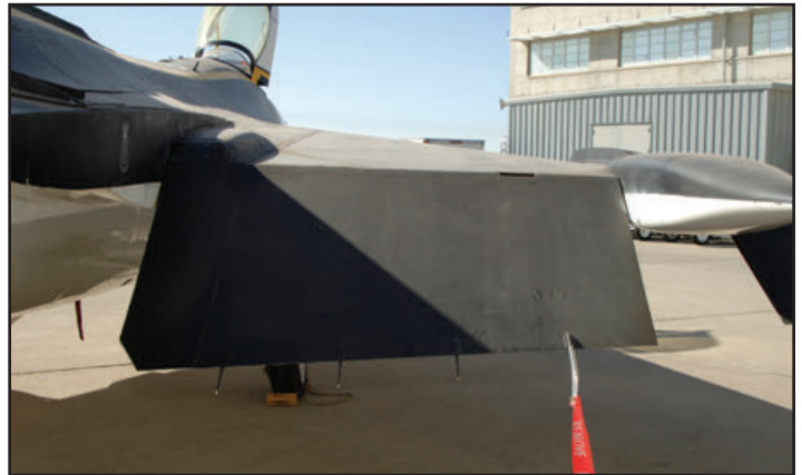
The wing is made up of graphite polyimide composite skins attached to an aluminum under-structure, each incorporating independently-actuated elevon and aileron for pitch and roll control. Leading edge flaps are installed outboard on leading edge sweep break. (Tony Landis)
