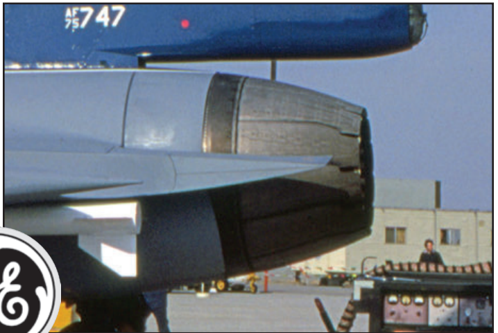
Powering F-16XL, 75-0749, throughout the entire test program was a Pratt & Whitney, F100-PW-200 afterburning turbofan engine capable of providing approximately 24,000 lbs maximum thrust, similar to those used in the basic F-16. (Pratt & Whitney- Top 2; USAF- above left; Keith Svendsen- above right)
