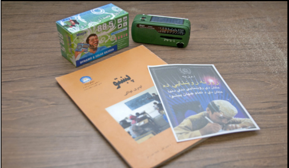
The Radio Literacy package includes one hand-crank radio and one handbook per family. This radio can receive AM, FM or shortwave radio frequencies and can be charged via hand-crank, solar panel, or operated off typical AAA batteries, said Master Sgt. Joel E. Fix, of Fort Belvoir, Va., 116th Infantry Brigade Combat Team, who oversaw the Radio Literacy program.
