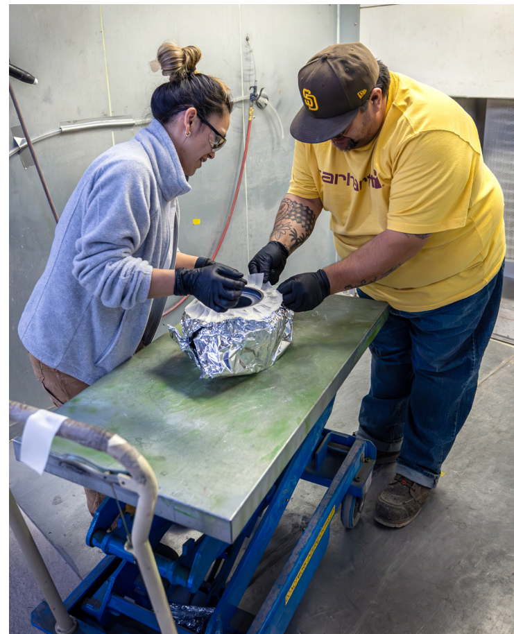
ABOVE: Danielle Blas and William Maine, both painter blaster mechanics, Shop 71, Painters Blasters and Tilers mask a portion of a part before spraying it with an epoxy powder, May 29, in Building 431. (U.S. Navy photo by Jeb Fach)
