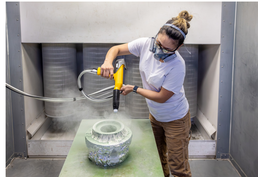
ABOVE: Danielle Blas, painter blaster mechanic, Shop 71, Painters Blasters and Tilesetters, sprays a part with an epoxy powder, May 29, in Building 431. (U.S. Navy photo by Jeb Fach)
