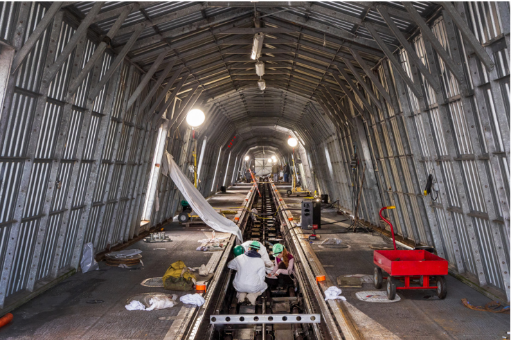
ABOVE: Aircraft Launch and Recovery team members from Shop 38, Marine Machinist, work to align one of three catapults aboard USS Nimitz (CVN 68) Jan. 7, 2024, during a six-month planned incremental availability at PSNS & IMF. (U.S. Navy photo by Wendy Hallmark)
