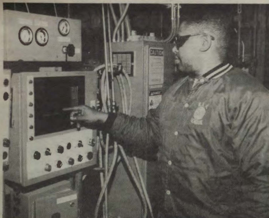
Eddie Fowler programs the forge hammer at a computer console. The hammer can be set to strike with a force of up to 197,000 pounds.
