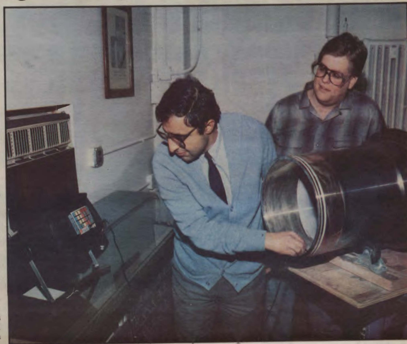
Larry Windschilt (left) of RIA's Quality Assurance Directorate and M.M.Y. El Monayer perform a non-destructive test designed to measure the thickness of bronze in a piston used on a gun mount.
