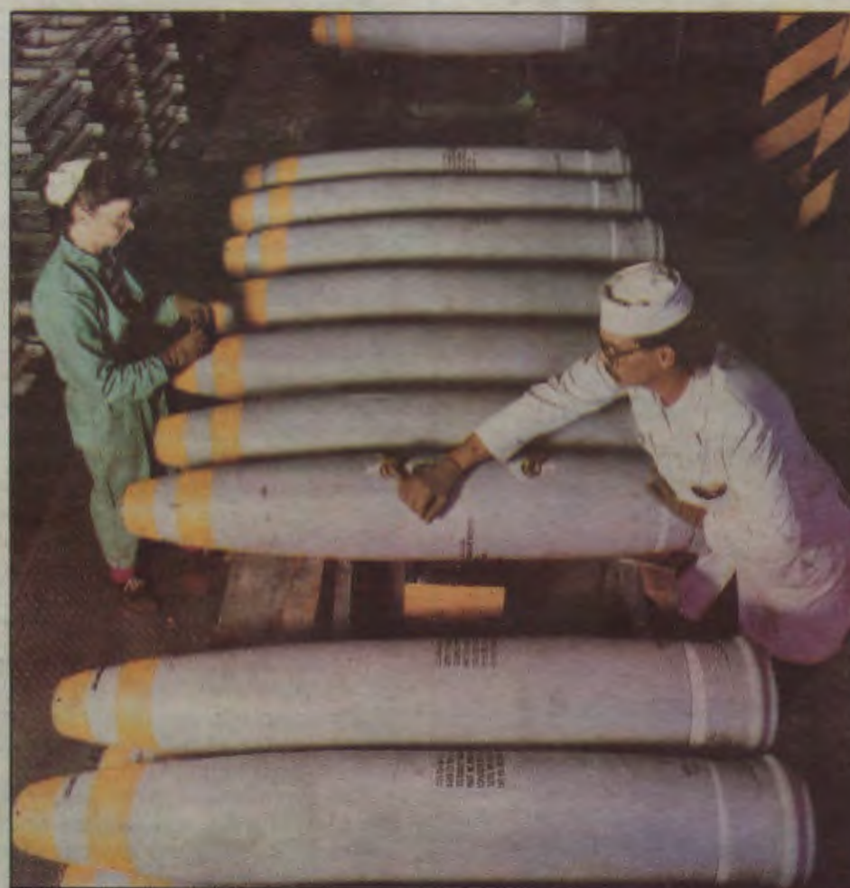
Aerial bombs are produced at McAlester Army Ammunition Plant, Okla. IOC's installations can produce items as large or larger than these bombs while meeting tolerances measured in thousandths of an inch.
