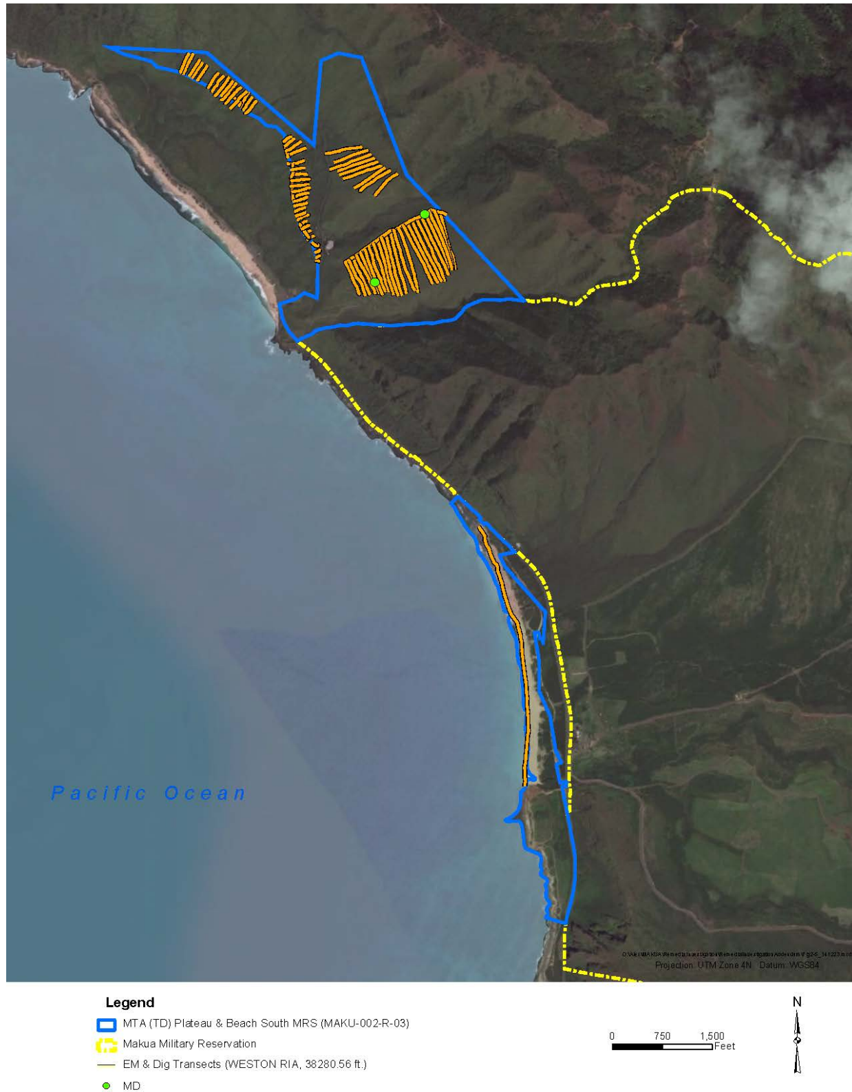
Figure 2-5: Remedial Investigation Addendum Geophysical Survey Transects and MEC Investigation Results
