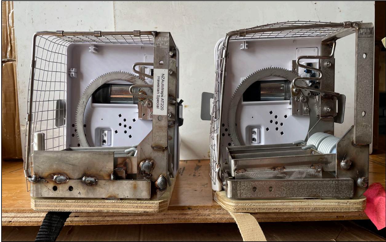
Figure 22: Two models of the AT-220 trap manufactured by NZ Auto Traps. The trap on the left (known as the ‘Hawaiian special’) is modified with an extended choke bar with the intent of making the trap more effective at humanely dispatching F. catus . The model on the right is the trap that ANRPO deployed during this reporting period. Photo taken by Troy Levinson
