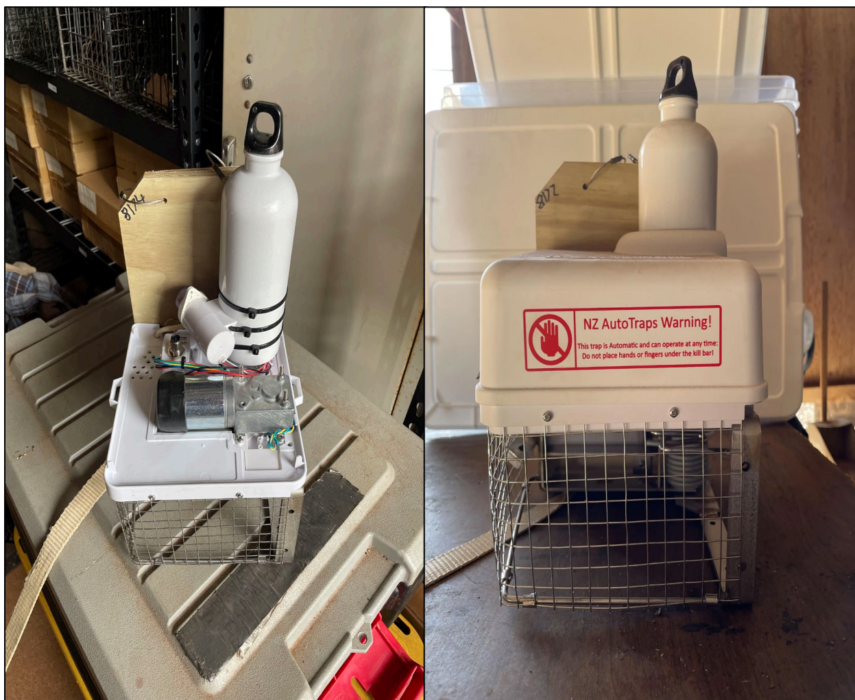
Figure 18: The AT-220 trap manufactured by NZ Auto Traps. The image on the left shows the internal components of the trap (battery hook up, electronic controller, bait bottle, bait pump). The image on the right shows the trap with the component cover which sits on top of all the electrical components and provides protection from weather and external damage. Photos by Troy Levinson
