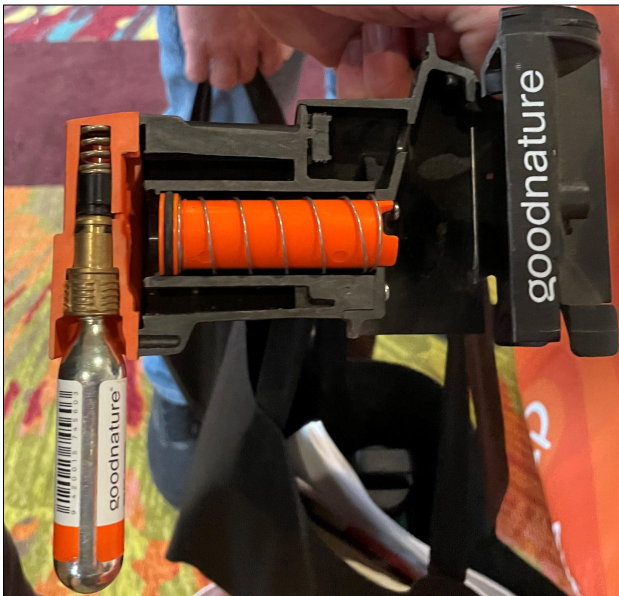
Figure 10: Cross section of a Goodnature A24 trap. This perspective shows the internal components and CO 2 reservoirs. Photo taken by Troy Levinson.
