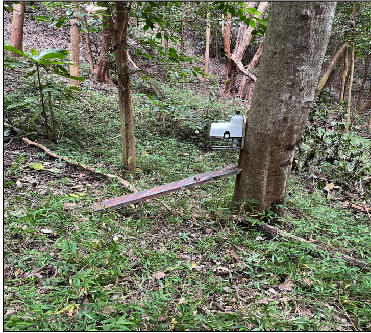
Figure 19: AT-220 trap setup in ‘Cyanea’ gulch, Ekahanui, Oahu. The ramp set up is recommended by NZ Auto Traps to assist in clearing carcasses from trap after lethal strikes. Photo taken by Troy Levinson.
