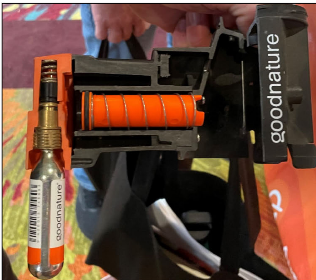
Figure 11: Cross section of a Goodnature A24 trap. This perspective shows the internal components and CO 2 reservoirs.
