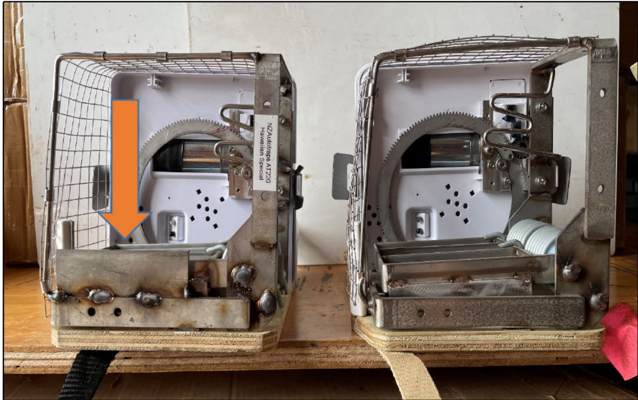
Figure 32: Two models of the AT220 trap manufactured by NZ Auto Traps. The trap on the left (known as the ‘Hawaiian special’) is modified with an extended choke (see orange arrow) bar with the intent of making the trap more effective at humanely dispatching F. catus . Photo taken by Troy Levinson
