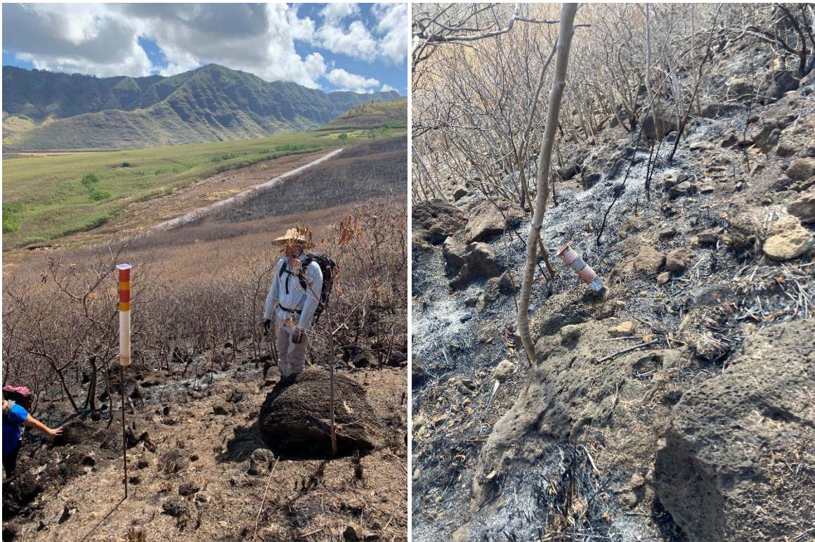
Left: undamaged Seibert Stake. Right: fire-damaged, melted Seibert Stake
