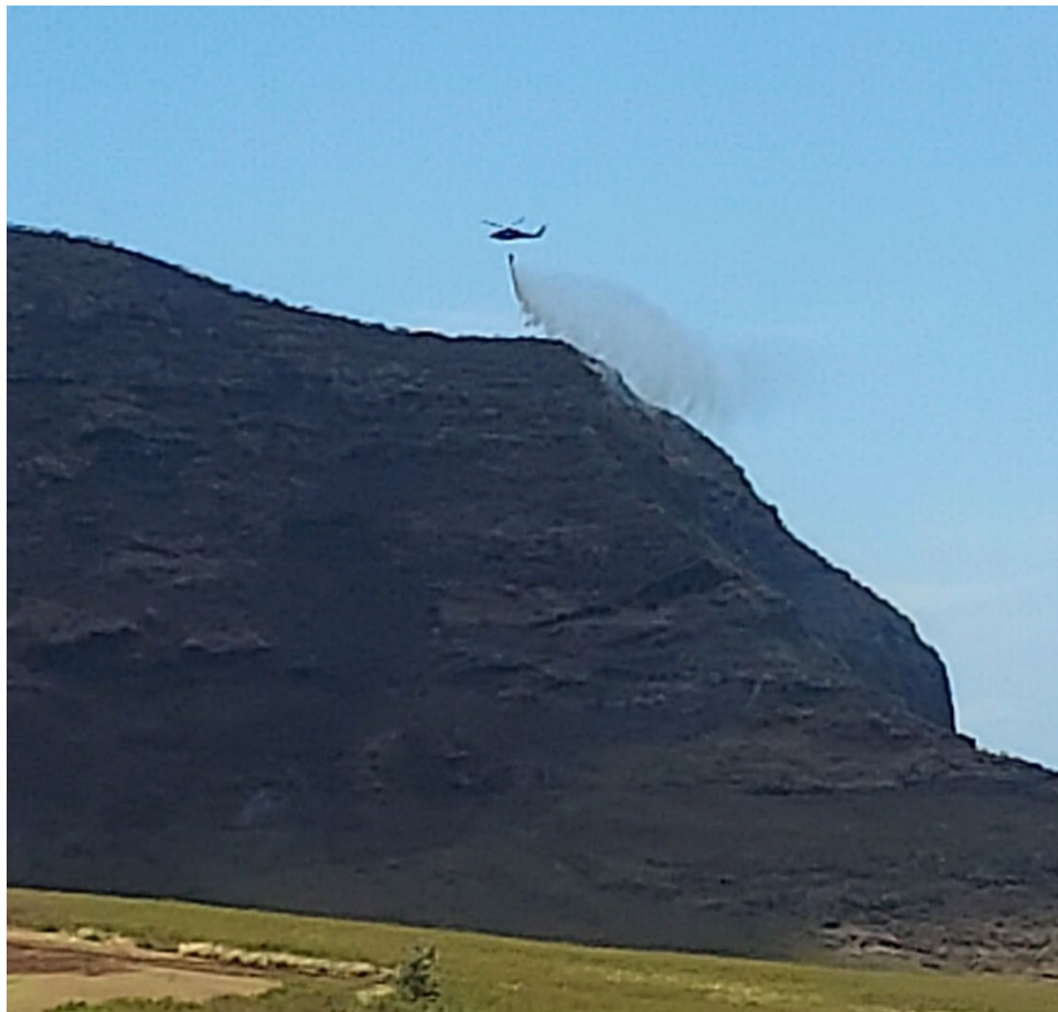
Blackhawk 440 dousing fire on ridge crest while maintaining airspeed to prevent downdraft
