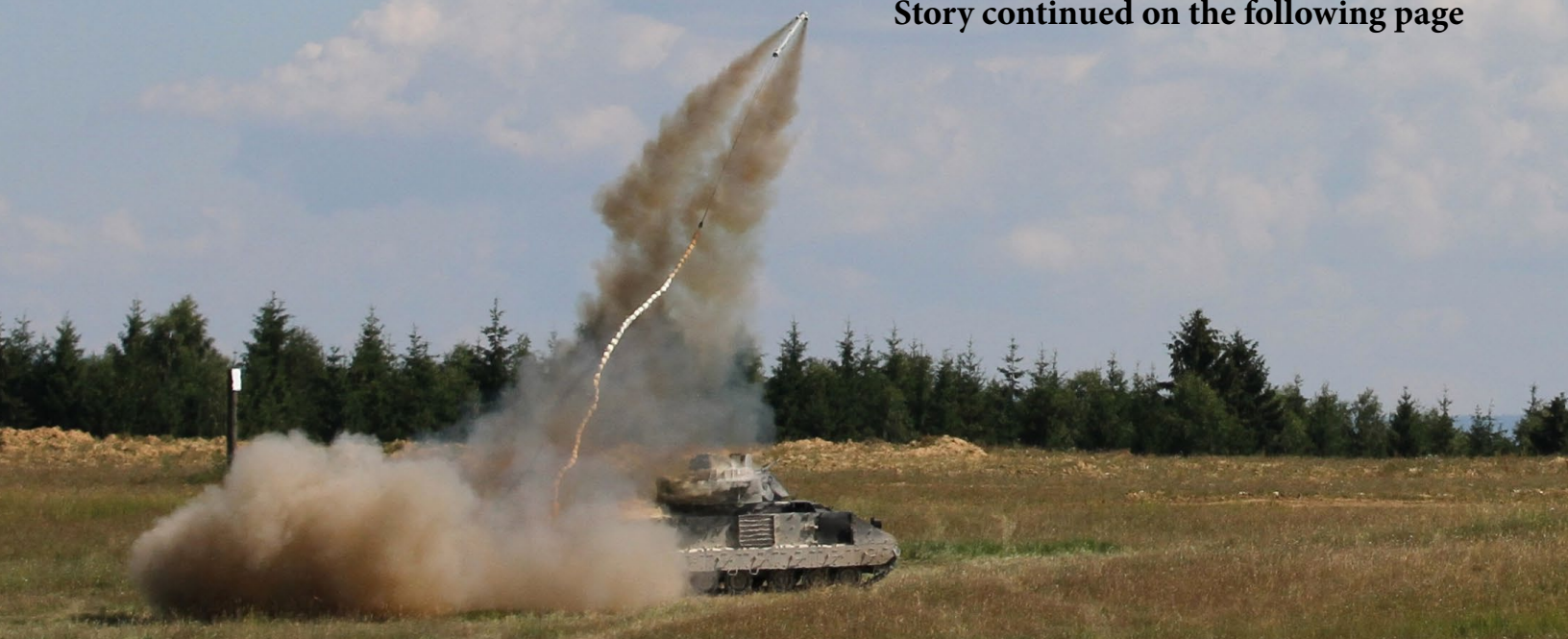
Combat engineers with Company B, 91st Brigade Engineer Battalion, 1st Brigade Combat Team, 1st Cavalry Division fire a mine clearing line charge during the combined arms live fire exercise at Grafenwoehr Army Base, Germany, June 27.
