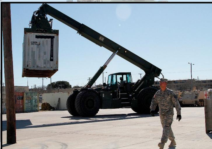
*Sgt. Gustavo Ocasio, a Muleskinner motor transport operator, guides an RT240 Kalmar Rough Terrain Container Handler as it moves shipping containers for transport, Jan. 14, at Fort Hood, Texas.*
