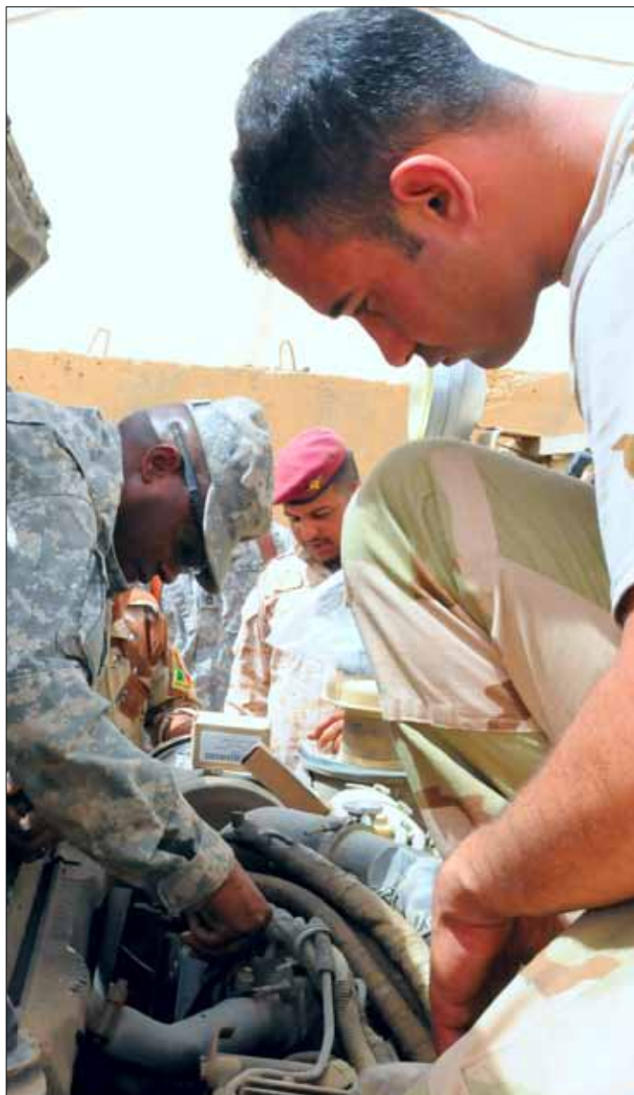
Staff Sgt. Hector Martyr, Maintenance Troop, Regimental Support Squadron, shows Soldiers with the 31st Iraqi Army Brigade the correct way to check for damage on a belt on a Humvee.
