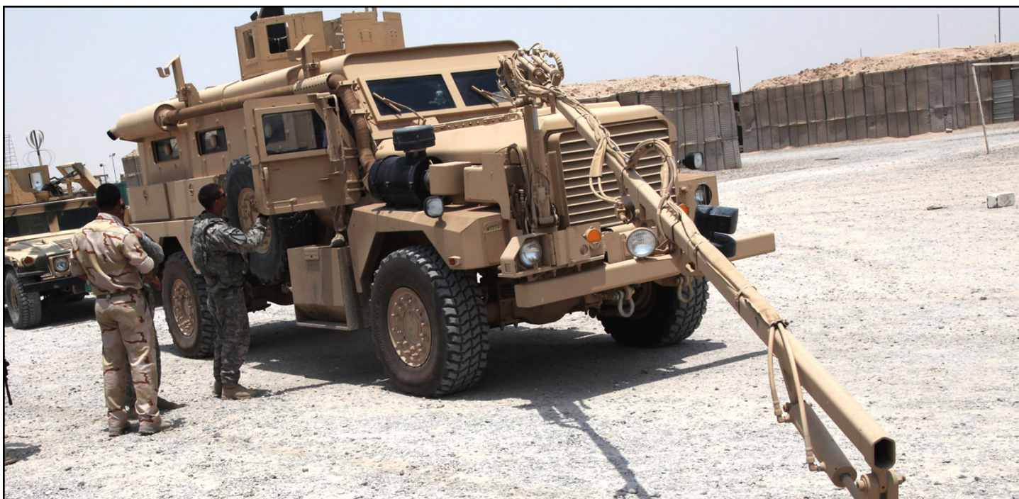
Soldiers from Headquarters and Headquarters Company, 1st Battalion, 12th Cavalry Regiment, 3rd Advise and Assist Brigade, 1st Cavalry Division instruct Iraqi Army engineers on use of the interrogation arm used for route clearance July 12.
