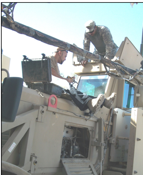
Spc. Johnny Wade C Co., 2-1 BSTB, and George Garcia, R4 installer, hook-up a Rhino battery cable on a Husky.
