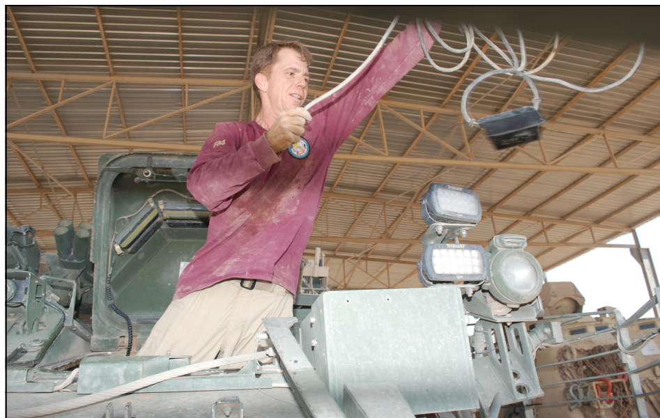
Steve Rolan, site manager, IED-Defeat, 1st Battalion, 402nd Army Field Support Brigade, removes a Rhino jamming system control unit from a Stryker at Joint Base Balad, Iraq.
