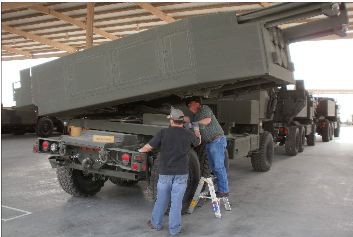
Personnel inspect hydraulic and electrical lines on the underside of a launcher.
