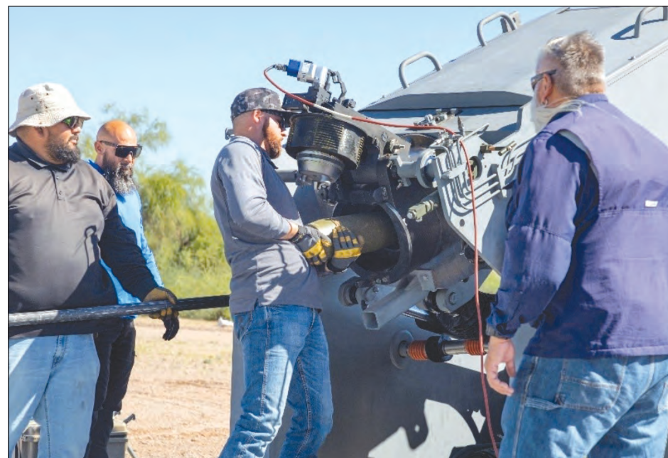
Once the system was set up Sorenson conducted acceptance firing. “We fired at four QEs [quadrant elevations] just to make sure everything was good as we elevated up and down. Most were done at zone five to introduce maximum shock and everything went well.”
