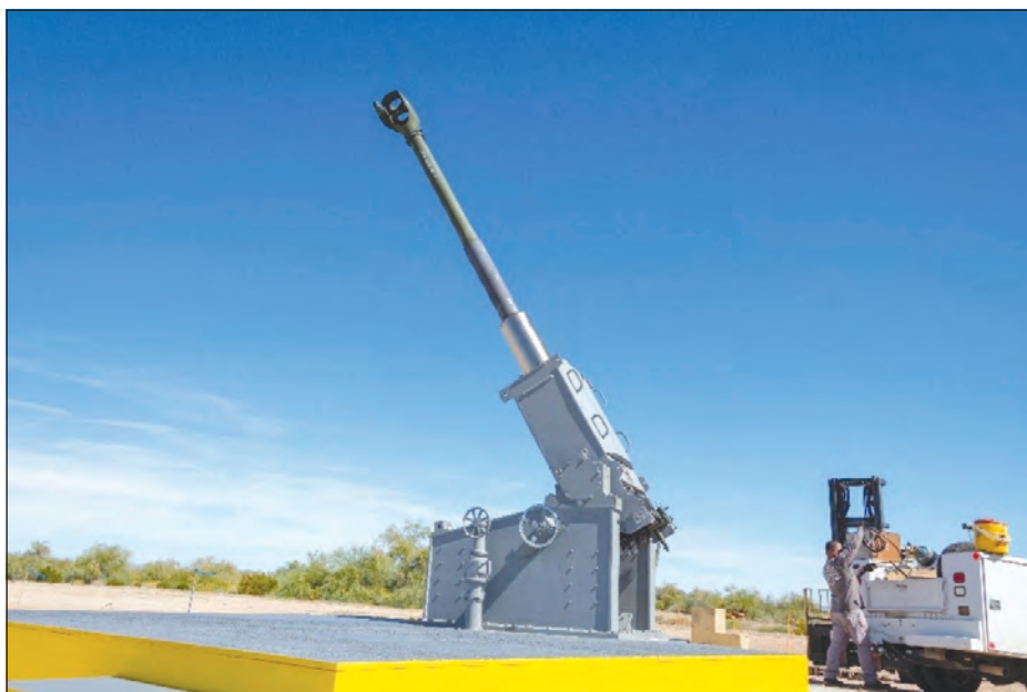
Yuma Test Center acquired a Proof Gun System (PGS) developed by U.S. Army Combat Capabilities Development Command Armaments Center, which allows a gun tube to be mounted and fired for testing without the weapon system. (U.S. Army photo)
