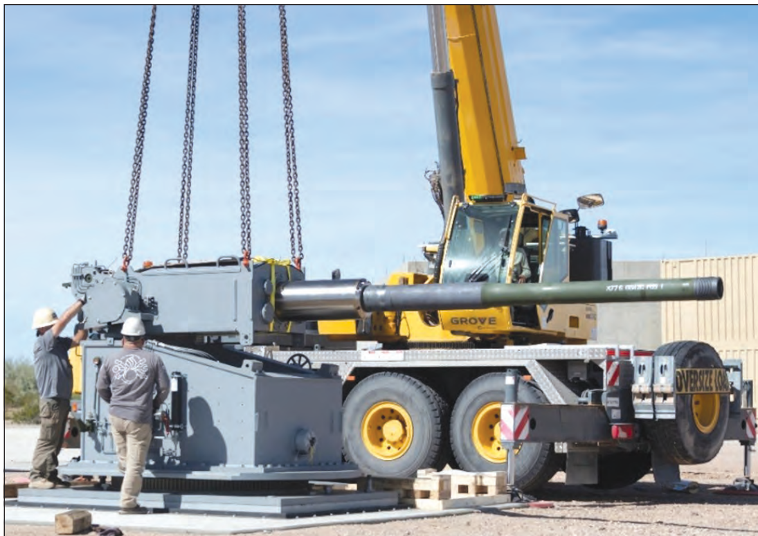
For the last several months, Yuma Test Center (YTC) worked to acquire, assemble, emplace and test fire the first of two Proof Gun System. YTC crews placed the system on a reaction mass built to sustain the immense power of firing. (U.S. Army photos)
