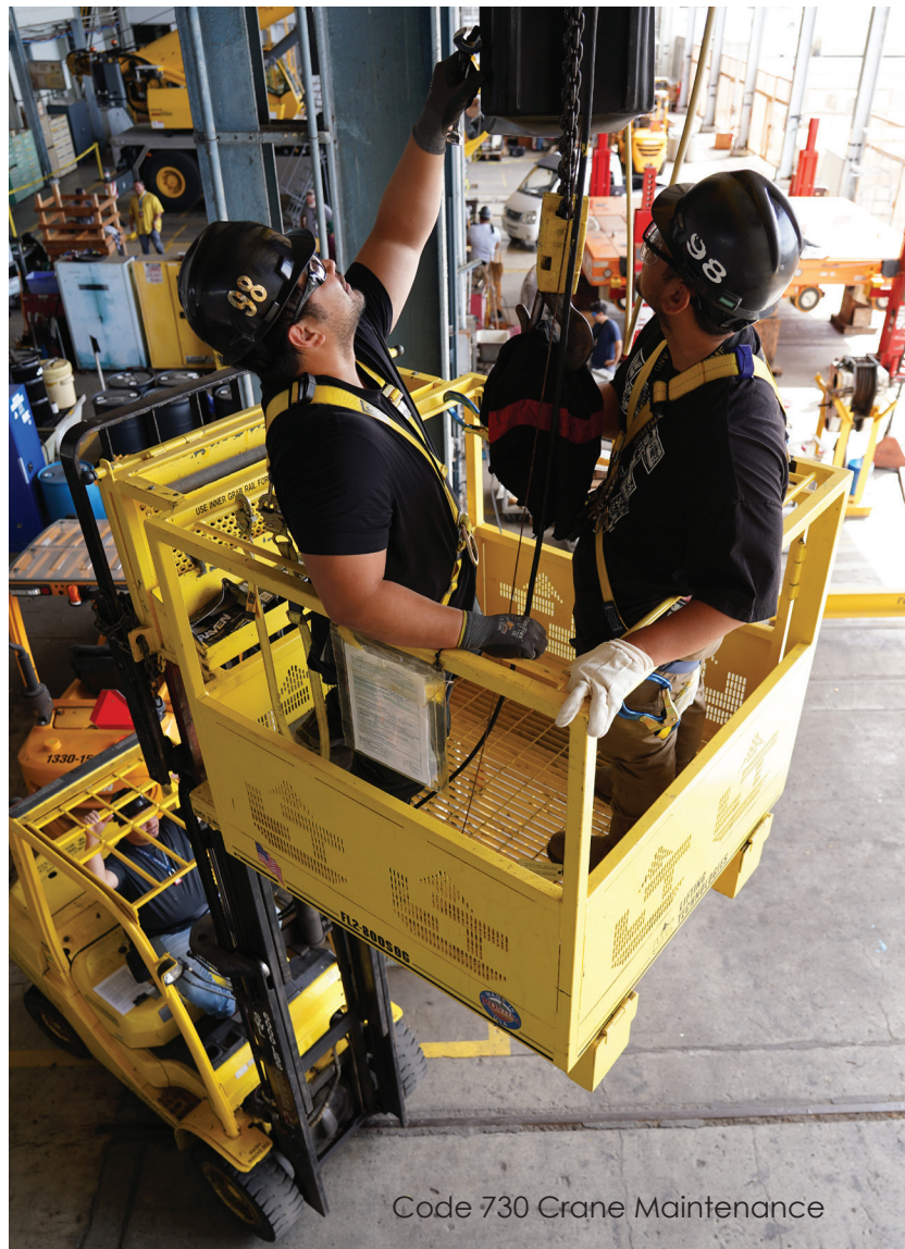
Code 730 Crane Maintenance Mechanics Matthew Solomona and Jharrin Kanehailua lubricate the load chain on a CAT III crane.
