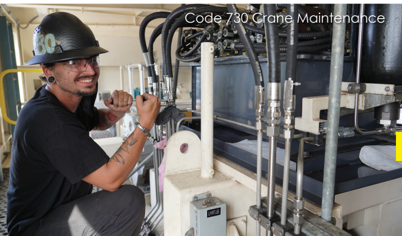
Code 730 Crane Maintenance Mechanic Colten Pregana checks hydraulic connections on a portal crane.
