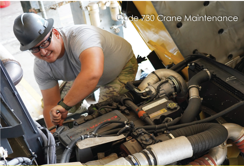
Code 730 Crane Maintenance Mechanical Apprentice Brant Shiroma performs an engine leak repair on a mobile crane.
