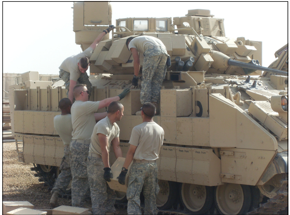
Soldiers from the 3rd Armored Cavalry Regiment, 3rd Infantry Division, install Bradley Reactive Armor Tile II kits at Contingency Operating Station Kalsu.
