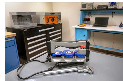
ABOVE: The LED-based UVC sanitizer was designed to help combat COVID-19 in 2020.
