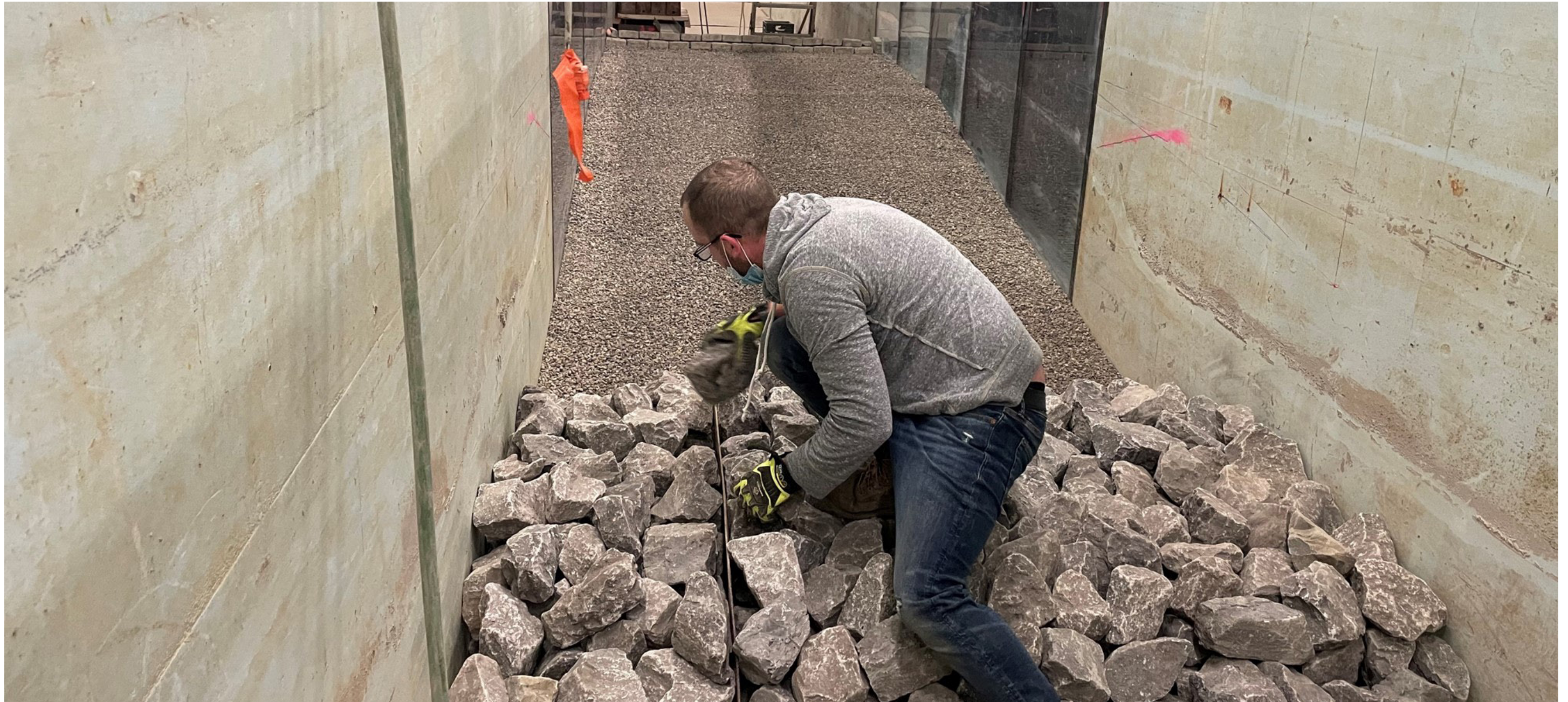
Offshore breakwater in foreground; dynamic revetment and stepped salvaged stone at rear.
