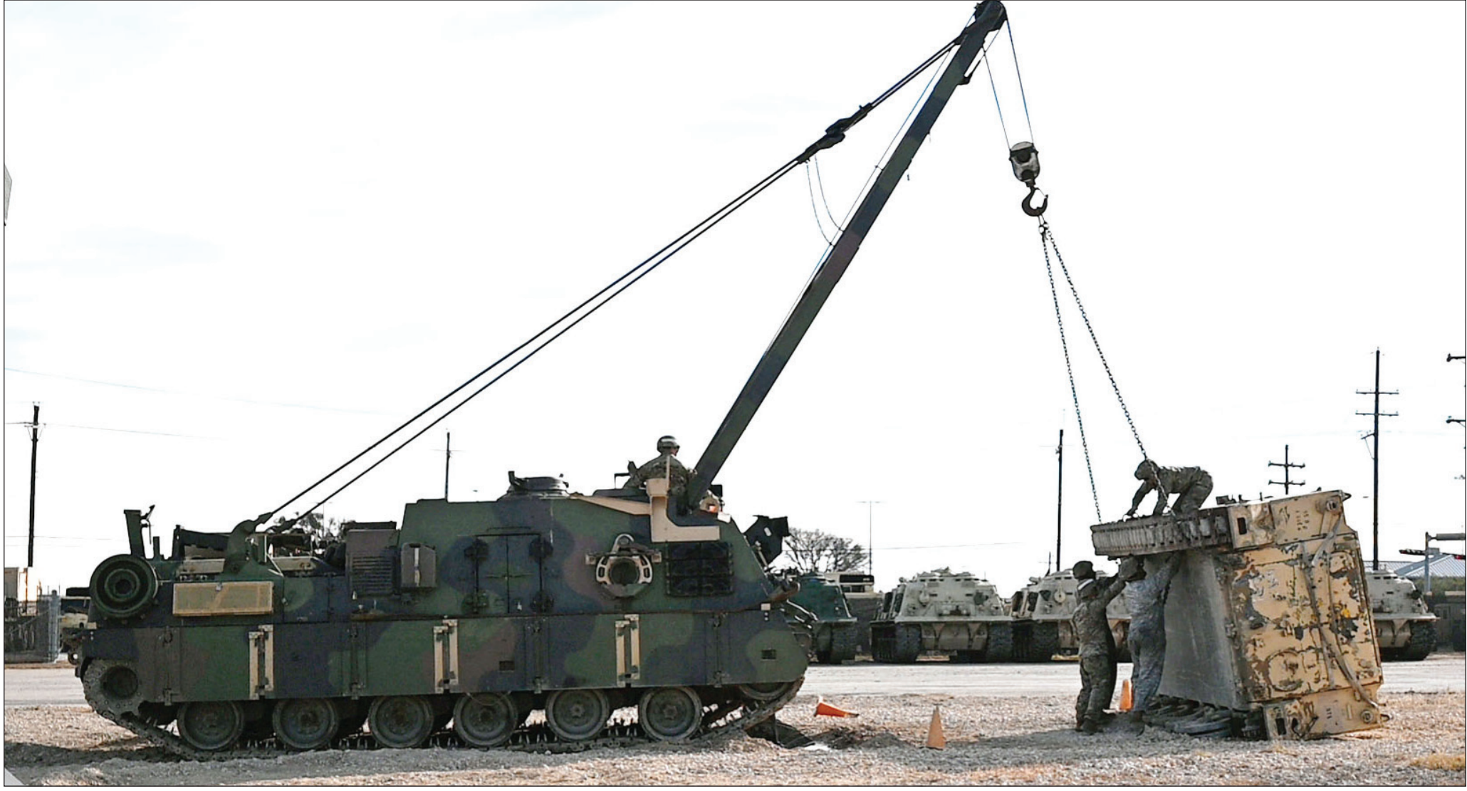
ABOVE, Track vehicle maintainer Soldiers begin an exercise to properly right a M113 armored personnel carrier during recovery training. Jan. 15 at Fort Cavazos. TOP RIGHT, Sgt. Sara Black, a track vehicle repairer, 1st Squadron, 7th Cavalry Regiment, 1st Cavalry Division, secures a tow hook to begin recovery operations on an M113 armored personnel carrier during the 17-day recovery training program Jan. 15 at Fort Cavazos.
