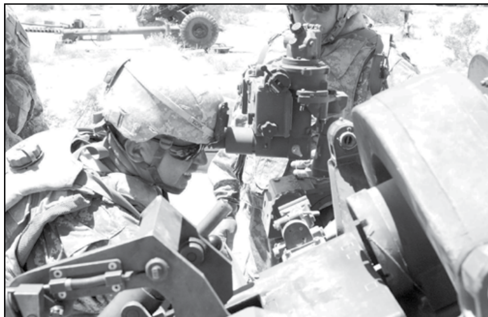
Sgt. Michael York, of Batt. A, gunner from Asheboro, N.C., views the sights of an M109, a 105mm howitzer to adjust the upper and lower limits in preparation of a live-fire calibration at NTC.
