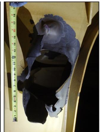
*Top: Debris fragments from an Iranian-made Shahed-136 unmanned aerial vehicle (UAV) collected as evidence by EODMU-3 aboard M/T Pacific Zircon. Bottom: Images taken by EODMU-3 aboard M/T Pacific Zircon showing shipboard damage from a UAV. (U.S. Navy photos)*
