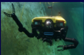
A VR DEFENDER ROV: Used for close-in reconnaissance, rapid reacquisition, and object recovery and emplacement
