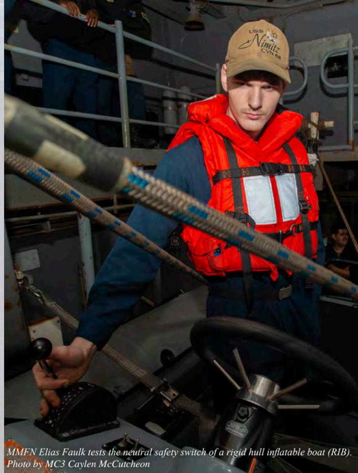
MMFN Elias Faulk tests the neutral safety switch of a rigid hull inflatable boat (RIB). Photo by MC3 Caylen McCutcheon
