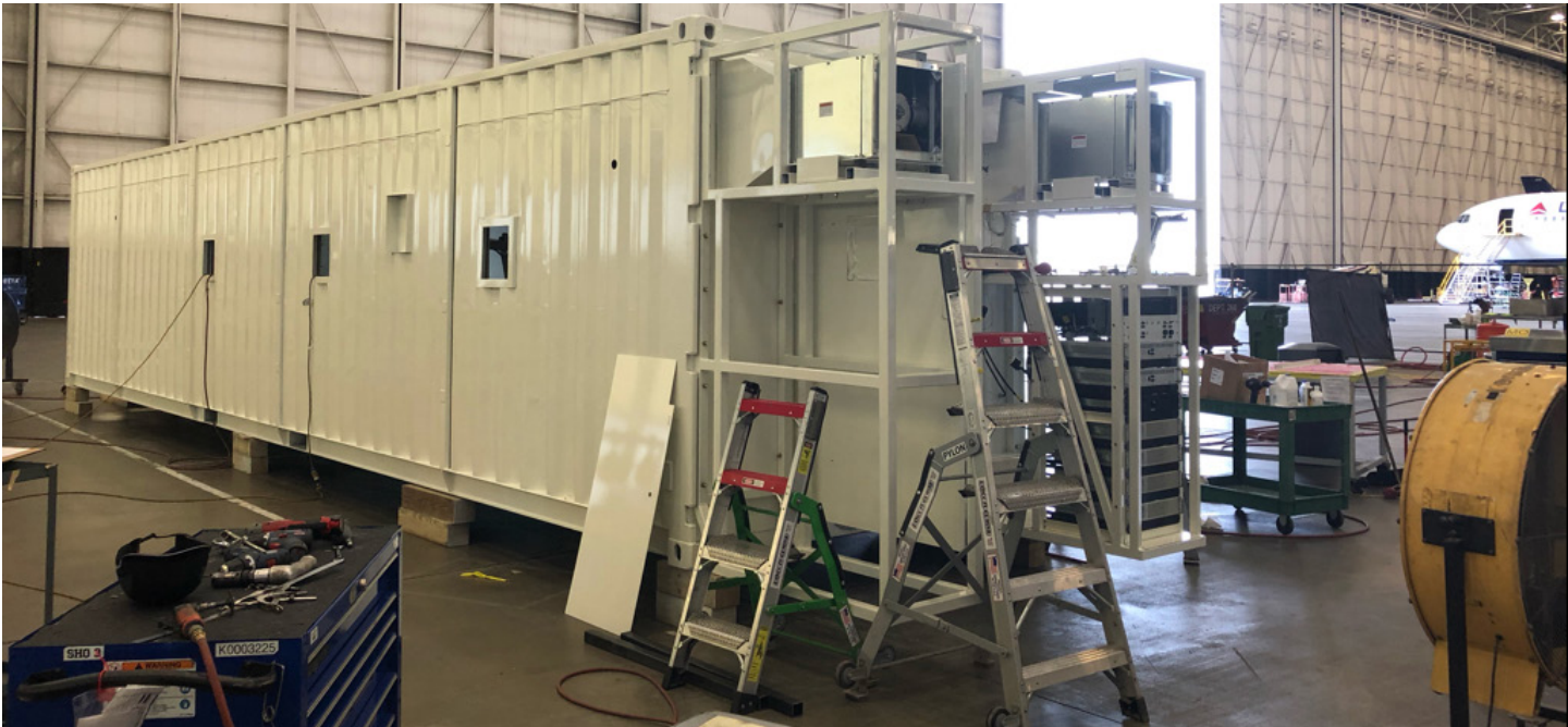
The exterior of the negative pressure Conex is designed to safely move COVID-19 patients by military aircraft while minimizing the infection risk to pilots and flight crew. DCMA provided technical support and quality assurance to ensure the NPC met all specifications and requirement during its rapid development and fielding. (DCMA photo by Vern Lewis)
