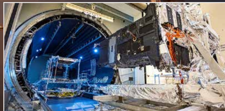
(Top left ) The GEO-5 satellite’s successful launch from Space Launch Complex 41 pad at Cape Canaveral Space Force Station, Florida. (Left) The SBIRS GEO-5 satellite enters a vacuum chamber at Lockheed Martin’s Sunnyvale, Calif., production facility to begin Thermal Vacuum testing. (Above) Also, in Sunnyvale, Lockheed Martin Space integrated the GEO-5 Space Vehicle. Space vehicles undergo acoustic testing, which verifies the satellite’s ability to withstand high levels of vibration in space. (Photos courtesy of Lockheed Martin and ULA)
