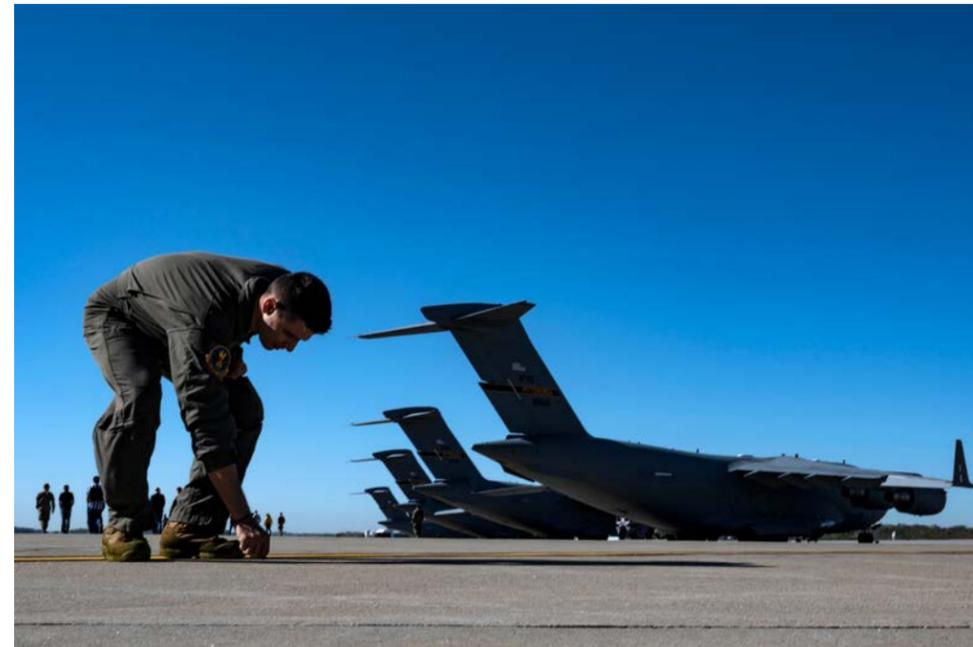
Tech. Sgt. Travis Hendell, 758th Airlift Squadron loadmaster, picks up a piece of foreign object debris, or FOD, during a 'FOD' walk at the Pittsburgh International Airport Air Reserve Station, Pennsylvania. Performing 'FOD' walks protects aircraft engines from any objects on the flight line that could be sucked into the engine and destroy it. (Air Force photo by Joshua Seybert)
