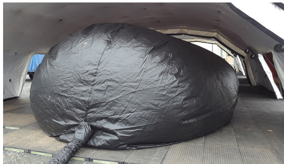
Inflatable bladder to raise the tents, and lower the tents. Also appearing in this photo is the portable floor. (Photo credit Major Richard Greenalch, Second CO. Governor's Foot Guard)
