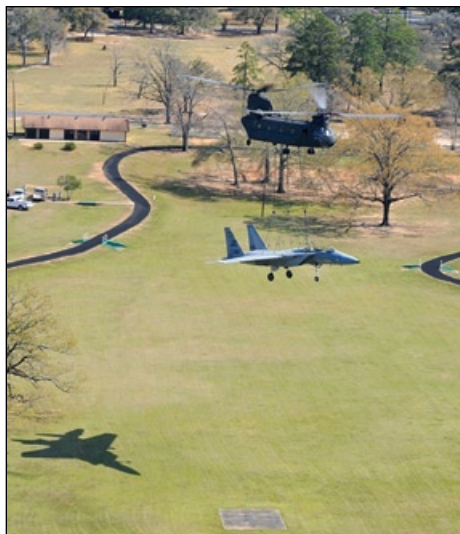
Right, Staff Sgt. Michael Chaney and Sgt. John T. Rogers of the Mississippi Army National Guard's B Company, 1/111th Aviation, helicopter crew complete the process of hooking the 159th Fighter Wing F-15 static display on three mounting points in preparation for flight to Camp Beauregard in Pineville, La., March 4.
