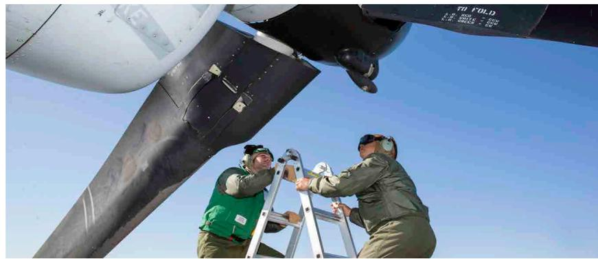
↑ Marines assigned to Marine Medium Tilt Rotor Squadron (VMM) 264 inspect a rotor air intake of an MV-22 Osprey parked on the flight deck aboard the amphibious assault ship USS WASP (LHD 1). (Photo by Mass Communication Specialist 2nd Class Nathan Wilkes)
