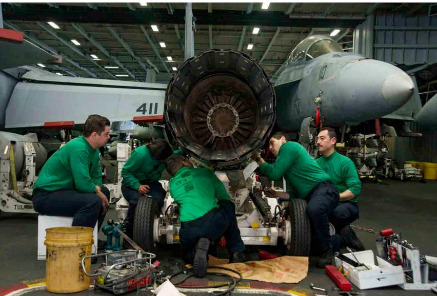
↑ Sailors conduct maintenance on a jet engine in the hangar bay of the aircraft carrier USS DWIGHT D. EISENHOWER (CVN 69). (Photo by Mass Communication Specialist Seaman Casey S. Trietsch)
