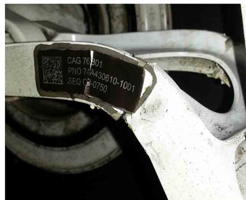
The nose landing gear lower torque arm of an FA-18E Super Hornet mentioned in the article was bent at an angle. The aircraft landed safely but left maintenance crews with many questions about how it was damaged. Photo by AM1 Justin Asper
