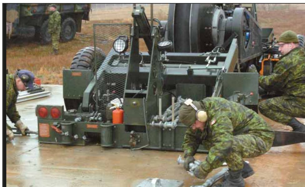
Students install the MAAS on concrete as part of an emergency installation.
