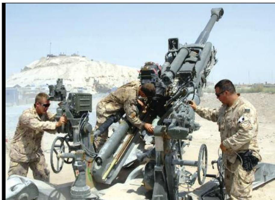
Soldiers from D Battery, 2 RCHA, in Afghanistan, prepare to fire their M777. The M777 delivers accurate supporting fire with explosive, smoke or illuminating rounds, and has a range of several kilometres.
