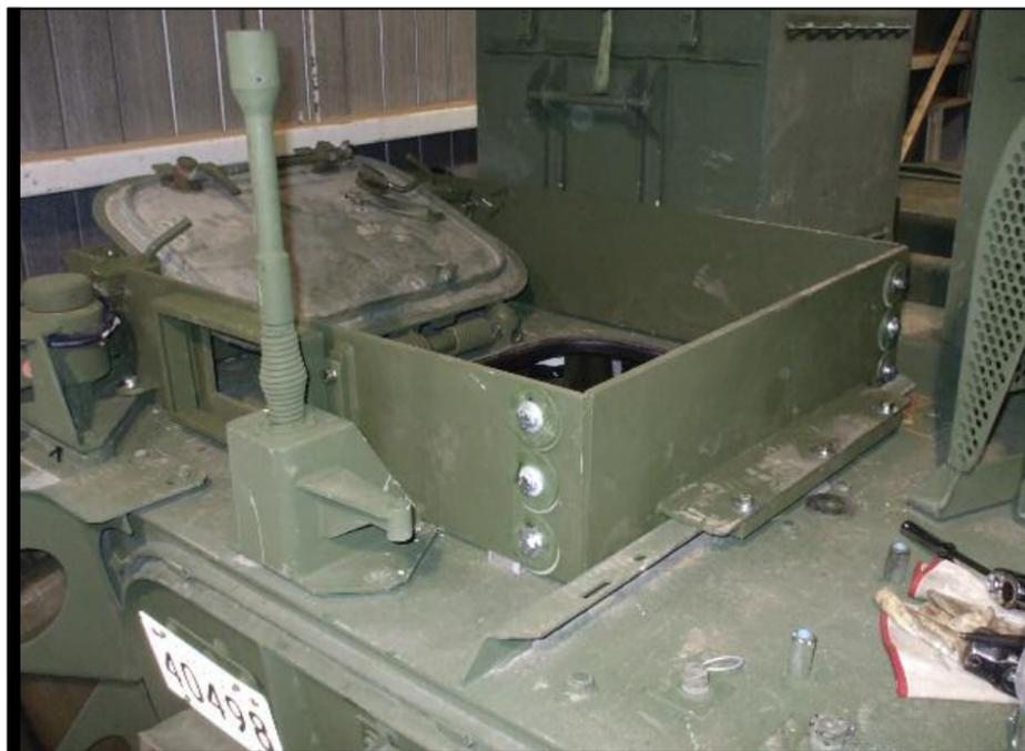
A LAV III Engineer fitted with an exposed crew protection kit.
