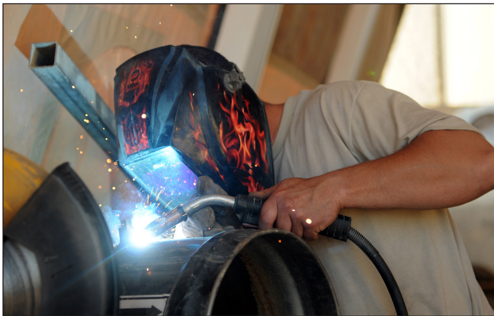
Pfc. Nathan Bates, a combat welder with Troop D, 1st Squadron, 75th Cavalry Regiment, joins two pieces of metal, turning an empty drum into a portable shower for one of the Squadron’s Combat Outposts.
