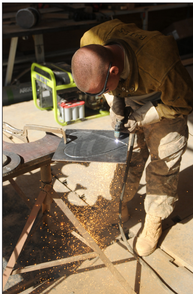
Pfc. Nathan Bates cuts metal with a plasma cutter at the squadron’s welding shop. The welders cut and shape metals to make custom parts needed.
