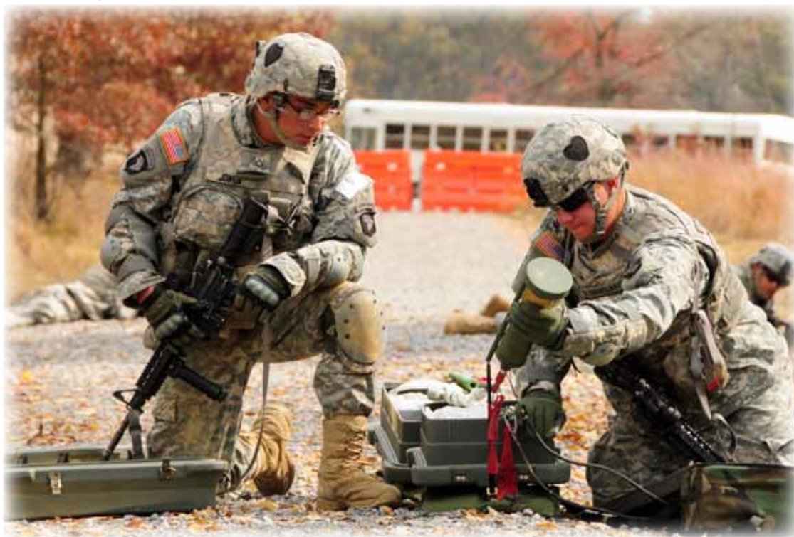
Pfc. Michael Jones and Pfc. Alexander Kornelakis, combat engineers with Company A, 2nd Brigade Special Troops Battalion, 2nd Brigade Combat Team, 101st Airborne Division (Air Assault), set up an anti-personnel obstacle breaching system during 'Sapper Stakes' at Fort Campbell, Ky., Oct. 26. Called 'APOBS', the system launches a line of explosive devices to trigger nearby hidden bombs to detonate, saving Soldier's lives in the field.
