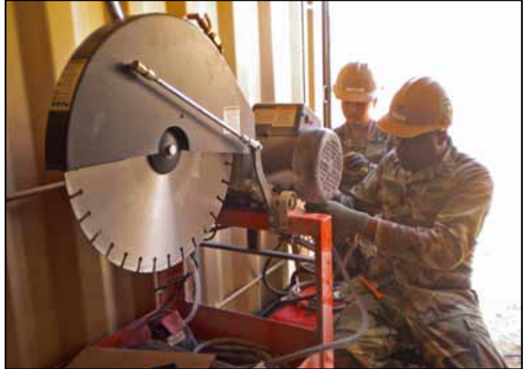
CE3 Foster and CECN Cusay wire up a block saw
