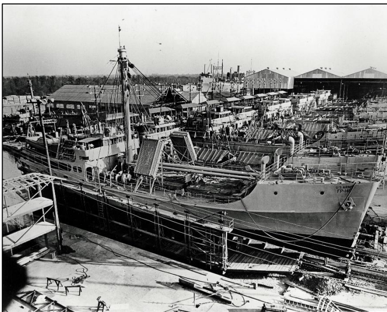
Figure 7: Freight/Shipping (FS) ship assembly line at the Higgins Shipyard's Industrial Canal facility in New Orleans ( www.nationalww2museum.org ).
