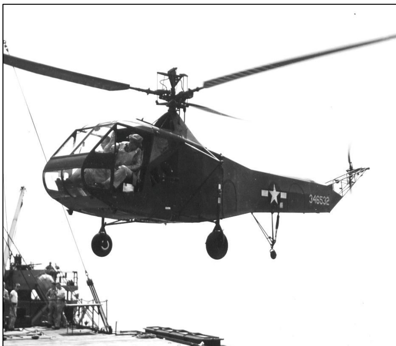
Figure 28: Sikorsky R-4B Hoverfly preparing to land on Repair Ship.
